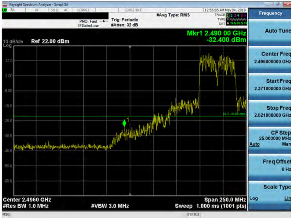
Plot 7-19. Lower Band Edge Plot (Band 38 QPSK – PCC:20 MHz SCC:15 MHz – Full RB)
