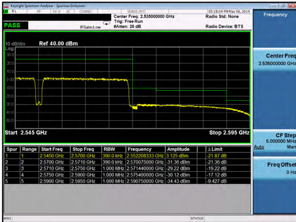
Plot 7-10. Upper Band Edge Plot (Band 20 QPSK – PCC:20 MHz SCC:20 MHz – Full RB)
