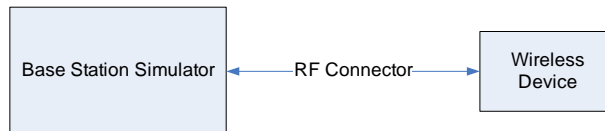
Figure 9-1 Power Measurement Setup
