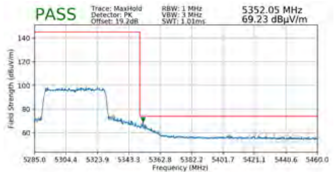
Plot 7-268. Radiated Upper Band Edge Plot SISO ANT1 (Peak – UNII Band 2A)
