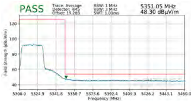
Plot 7-258. Radiated Upper Band Edge Plot SISO ANT1 (Average – UNII Band 2A)
