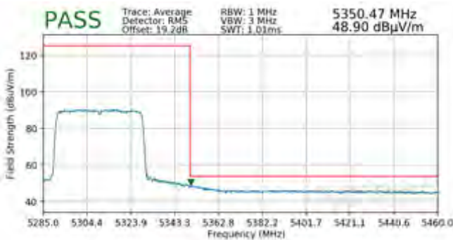
Plot 7-294. Radiated Upper Band Edge Plot SISO ANT2 (Average – UNII Band 2A)
