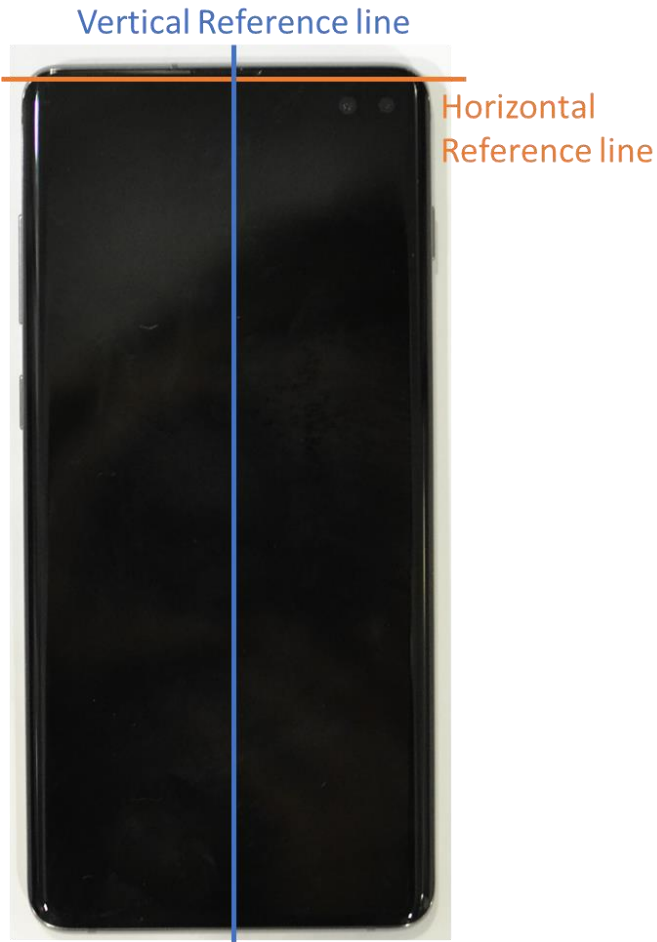
SAR Test Setup Photo 22 – Horizontal and Vertical Reference Lines
