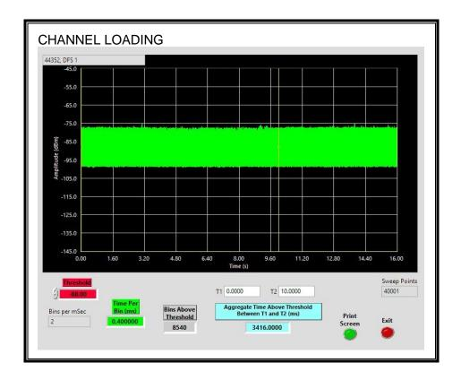
The level of traffic loading on the channel by the EUT is 34.16%.
