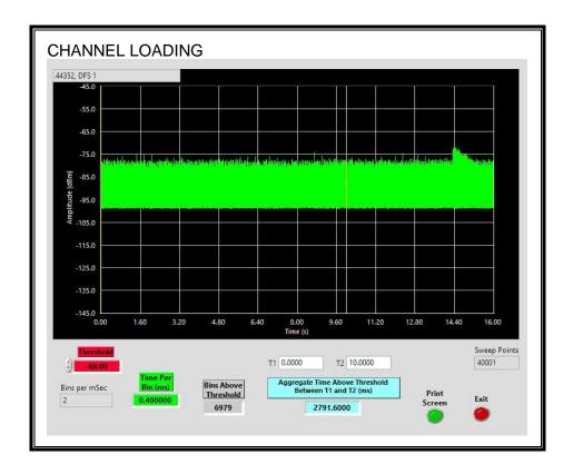
The level of traffic loading on the channel by the EUT is 27.916%.
