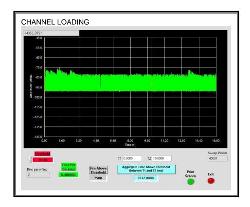
The level of traffic loading on the channel by the EUT is 30.32%.
