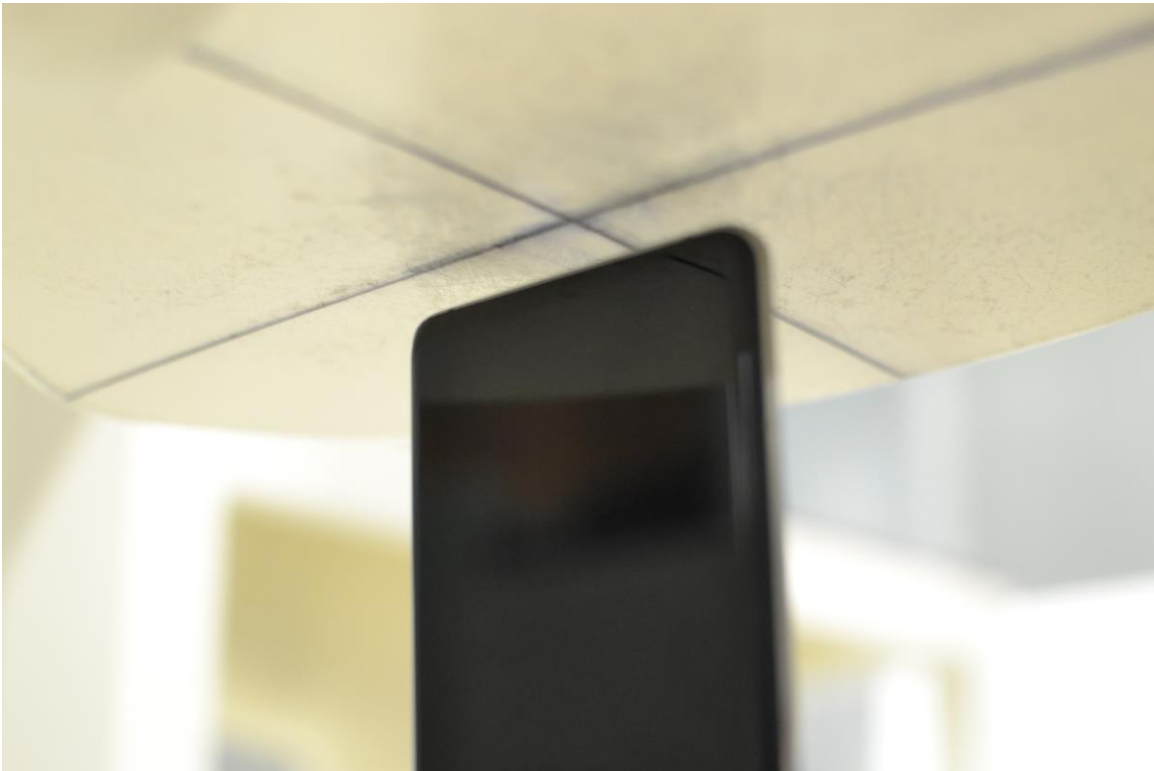
SAR Test Setup Photo 15 – Bottom Edge at 9 mm
