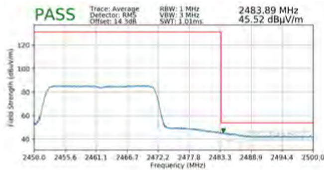
Plot 7-203. Radiated Restricted Band Edge Measurement SISO ANT2 with WCP (Average – 242 Tones)
