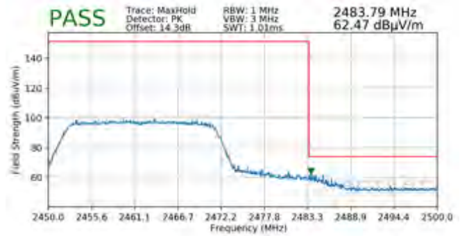
Plot 7-182. Radiated Restricted Band Edge Measurement SISO ANT1 with WCP (Peak – 242 Tones)
