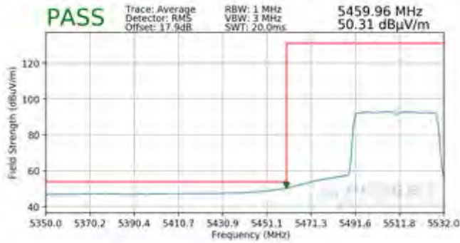
Plot 7-332. Radiated Lower Band Edge Plot SISO ANT2 (Average – UNII Band 2C)
