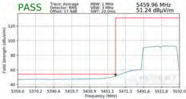
Plot 7-305. Radiated Lower Band Edge Plot SISO ANT1 (Average – UNII Band 2C)
