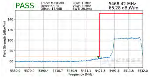
Plot 7-333. Radiated Lower Band Edge Plot SISO ANT2 (Peak – UNII Band 2C)
