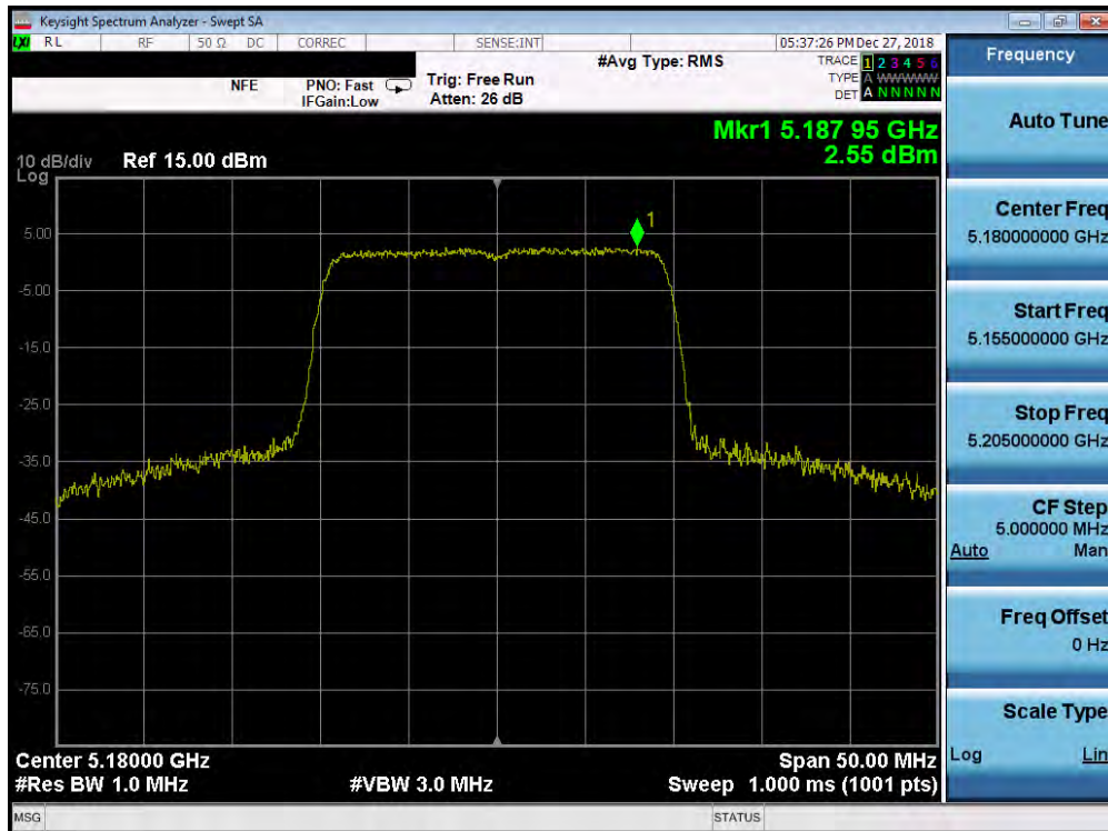
Plot 7-139. Power Spectral Density Plot SISO ANT1 (20MHz BW 802.11ax (UNII Band 1) – Ch. 36)
