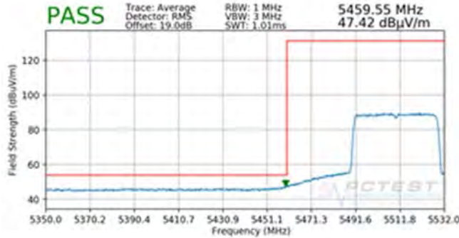
Plot 7-736. Radiated Lower Band Edge Plot SISO ANT2 (Average – UNII Band 2C – 484 Tones)
