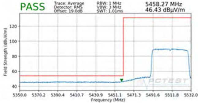
Plot 7-688. Radiated Lower Band Edge Plot SISO ANT1 (Average – UNII Band 2C – 484 Tones)
