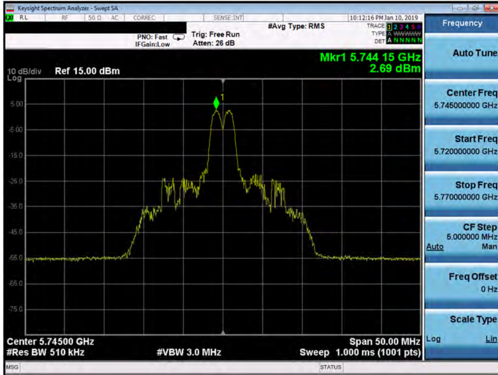
Plot 7-517. Power Spectral Density Plot MIMO ANT2 (20MHz BW 802.11ax – 26 Tones (UNII Band 3) – Ch. 149)
