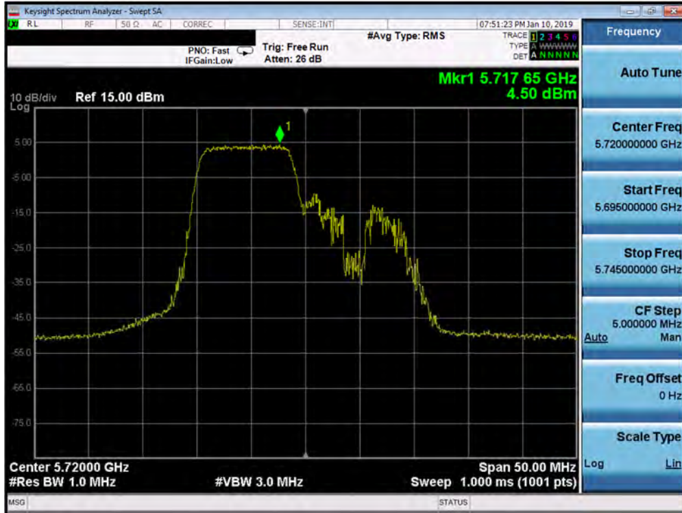
Plot 7-435. Power Spectral Density Plot MIMO ANT1 (20MHz BW 802.11ax – 106 Tones (UNII Band 2C) – Ch. 144)
