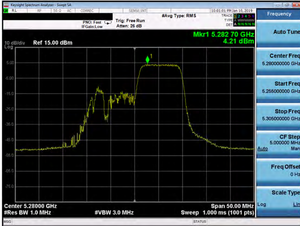
Plot 7-557. Power Spectral Density Plot MIMO ANT2 (20MHz BW 802.11ax – 106 Tones (UNII Band 2A) – Ch. 56)
