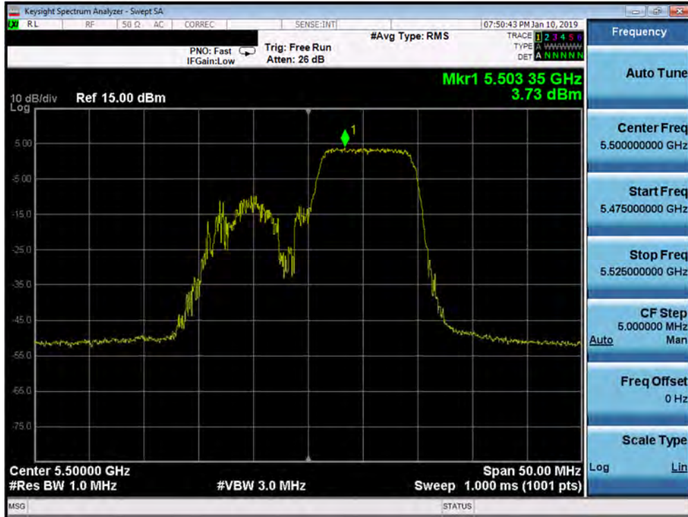
Plot 7-433. Power Spectral Density Plot MIMO ANT1 (20MHz BW 802.11ax – 106 Tones (UNII Band 2C) – Ch. 100)
