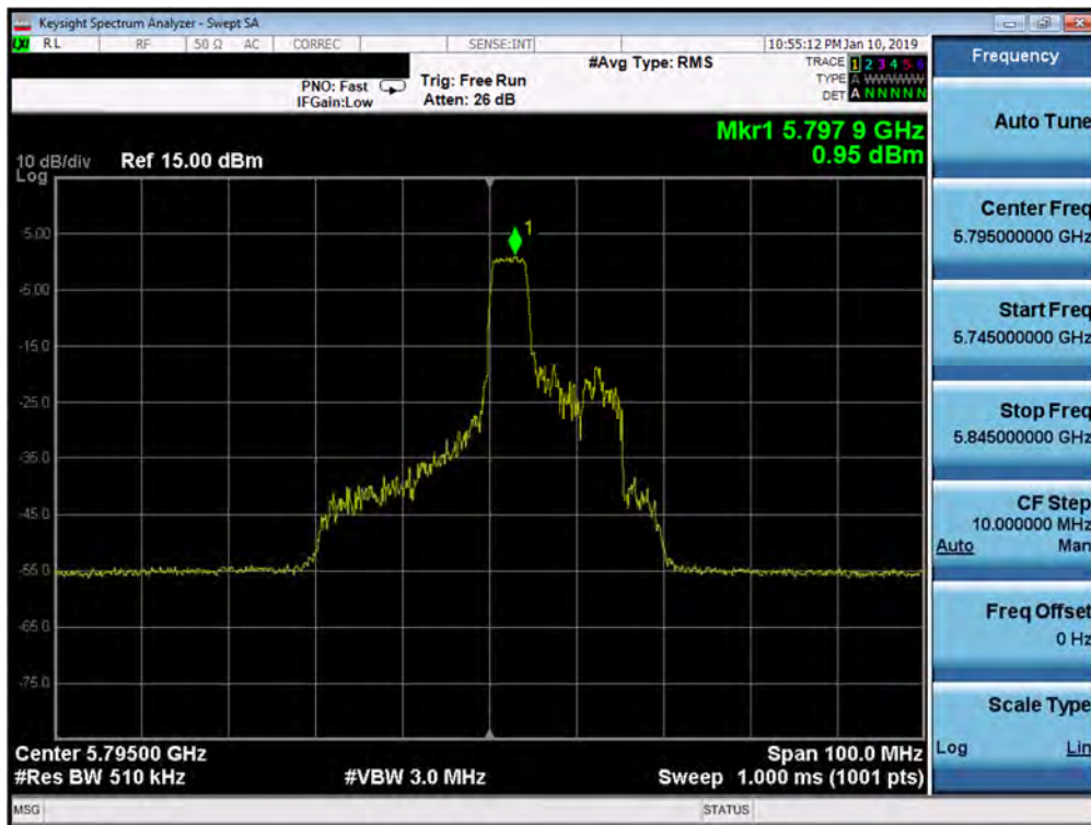
Plot 7-548. Power Spectral Density Plot MIMO ANT2 (40MHz BW 802.11ax – 52 Tones (UNII Band 3) – Ch. 159)
