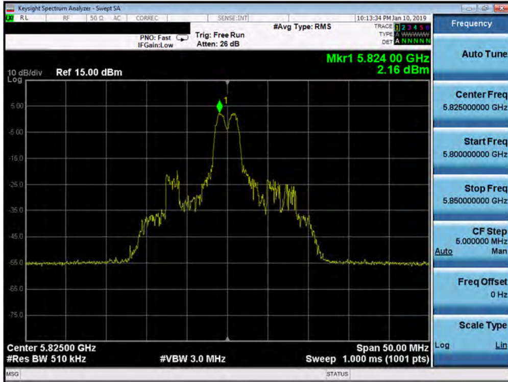
Plot 7-519. Power Spectral Density Plot MIMO ANT2 (20MHz BW 802.11ax – 26 Tones (UNII Band 3) – Ch. 165)
