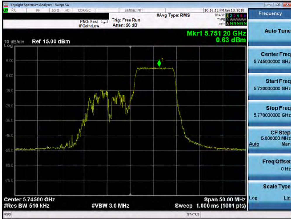
Plot 7-571. Power Spectral Density Plot MIMO ANT2 (20MHz BW 802.11ax – 106 Tones (UNII Band 3) – Ch. 149)
