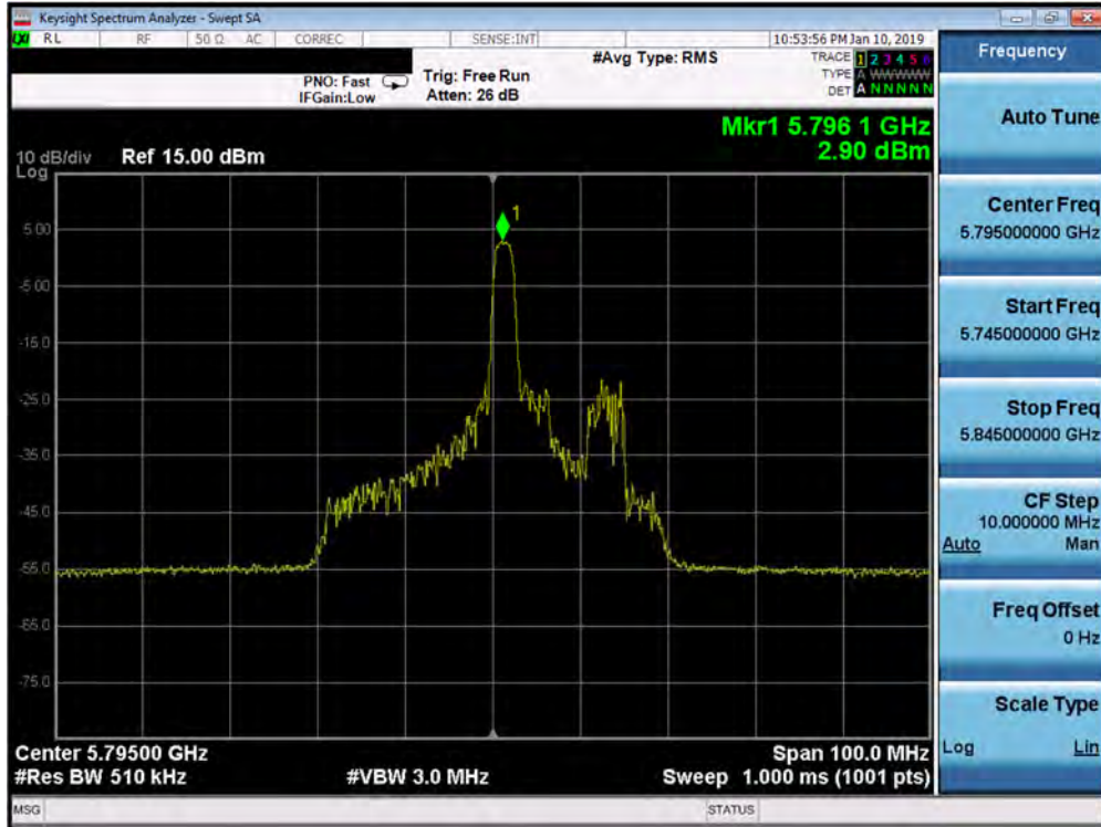
Plot 7-521. Power Spectral Density Plot MIMO ANT2 (40MHz BW 802.11ax – 26 Tones (UNII Band 3) – Ch. 159)
