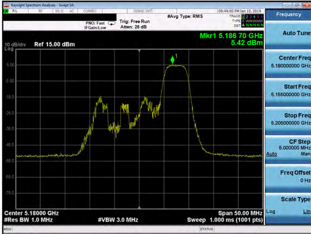
Plot 7-523. Power Spectral Density Plot MIMO ANT2 (20MHz BW 802.11ax – 52 Tones (UNII Band 1) – Ch. 36)
