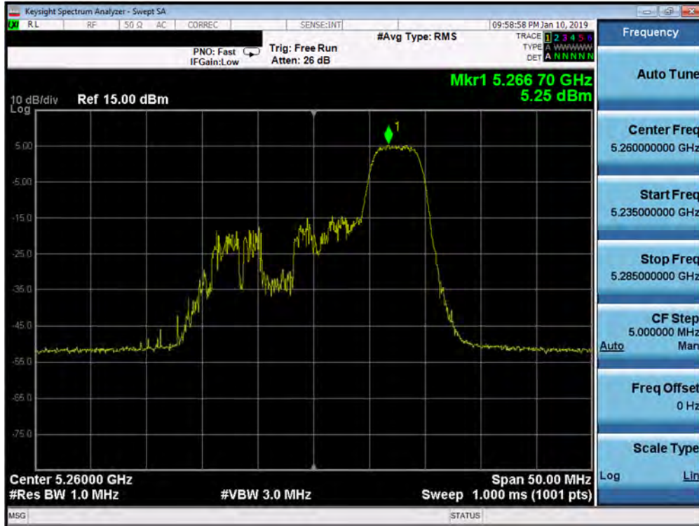
Plot 7-529. Power Spectral Density Plot MIMO ANT2 (20MHz BW 802.11ax – 52 Tones (UNII Band 2A) – Ch. 52)
