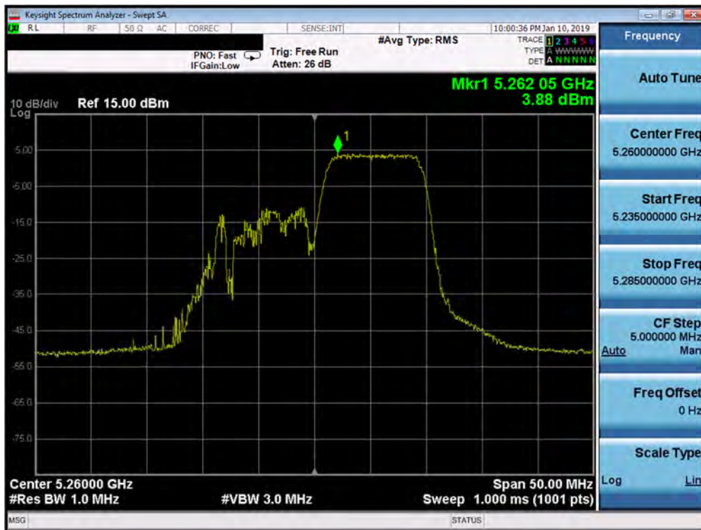
Plot 7-556. Power Spectral Density Plot MIMO ANT2 (20MHz BW 802.11ax – 106 Tones (UNII Band 2A) – Ch. 52)
