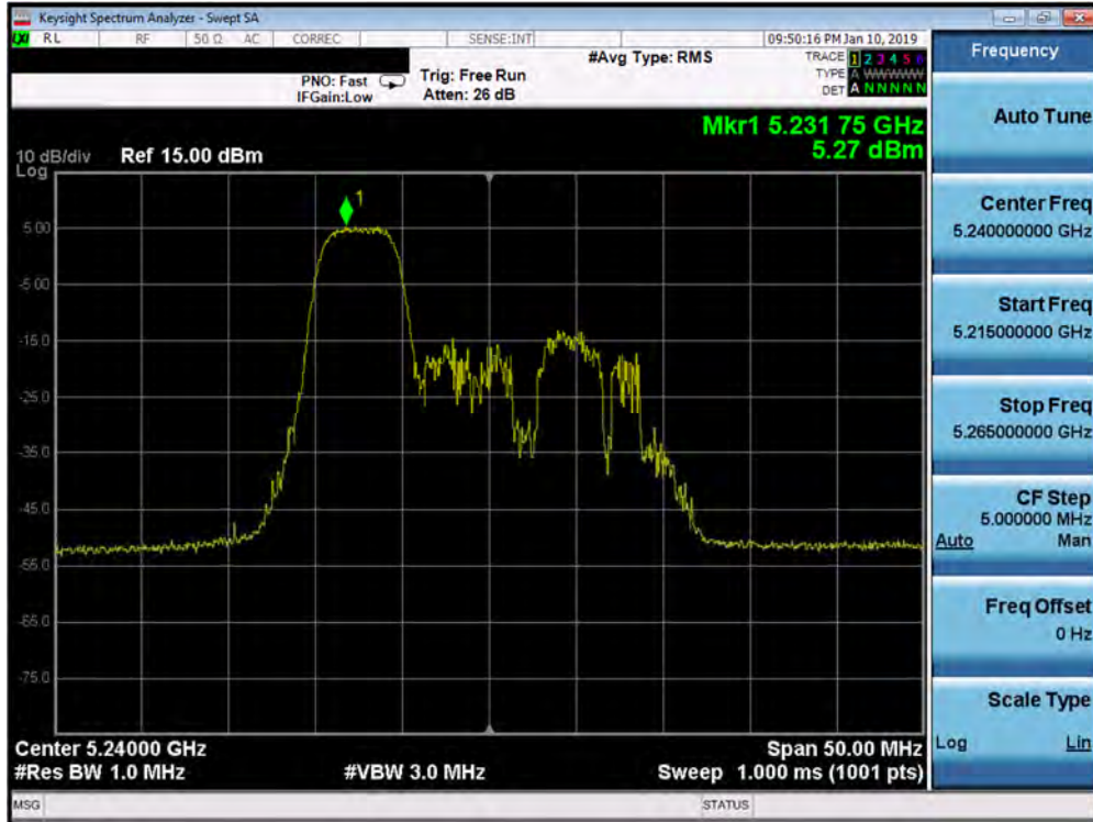
Plot 7-525. Power Spectral Density Plot MIMO ANT2 (20MHz BW 802.11ax – 52 Tones (UNII Band 1) – Ch. 48)
