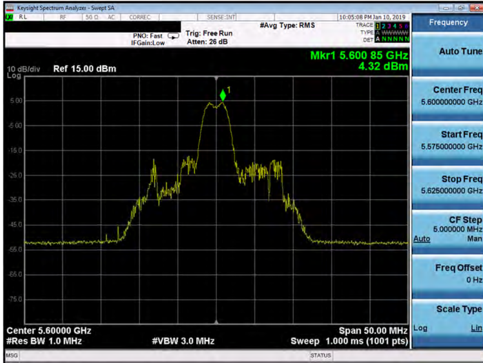
Plot 7-509. Power Spectral Density Plot MIMO ANT2 (20MHz BW 802.11ax – 26 Tones (UNII Band 2C) – Ch. 120)
