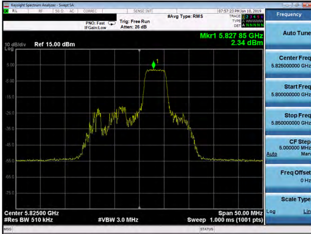
Plot 7-417. Power Spectral Density Plot MIMO ANT1 (20MHz BW 802.11ax – 52 Tones (UNII Band 3) – Ch. 165)
