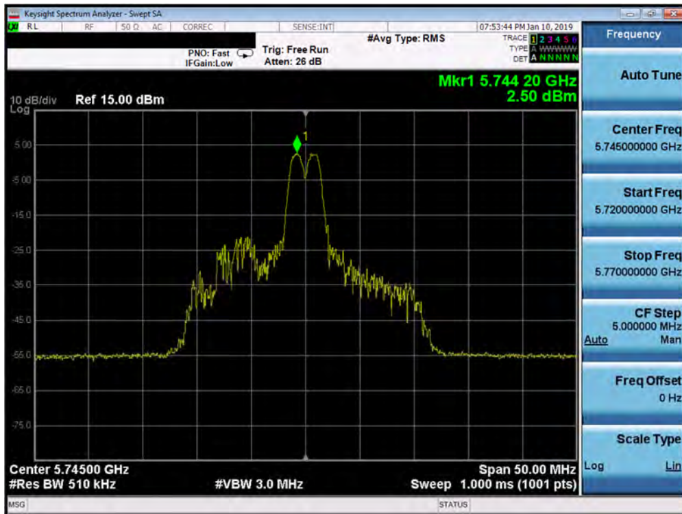
Plot 7-388. Power Spectral Density Plot MIMO ANT1 (20MHz BW 802.11ax – 26 Tones (UNII Band 3) – Ch. 149)
