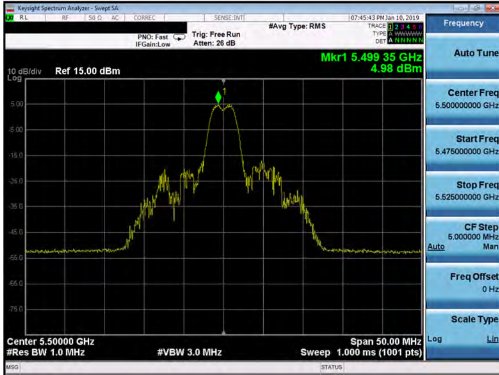
Plot 7-379. Power Spectral Density Plot MIMO ANT1 (20MHz BW 802.11ax – 26 Tones (UNII Band 2C) – Ch. 100)
