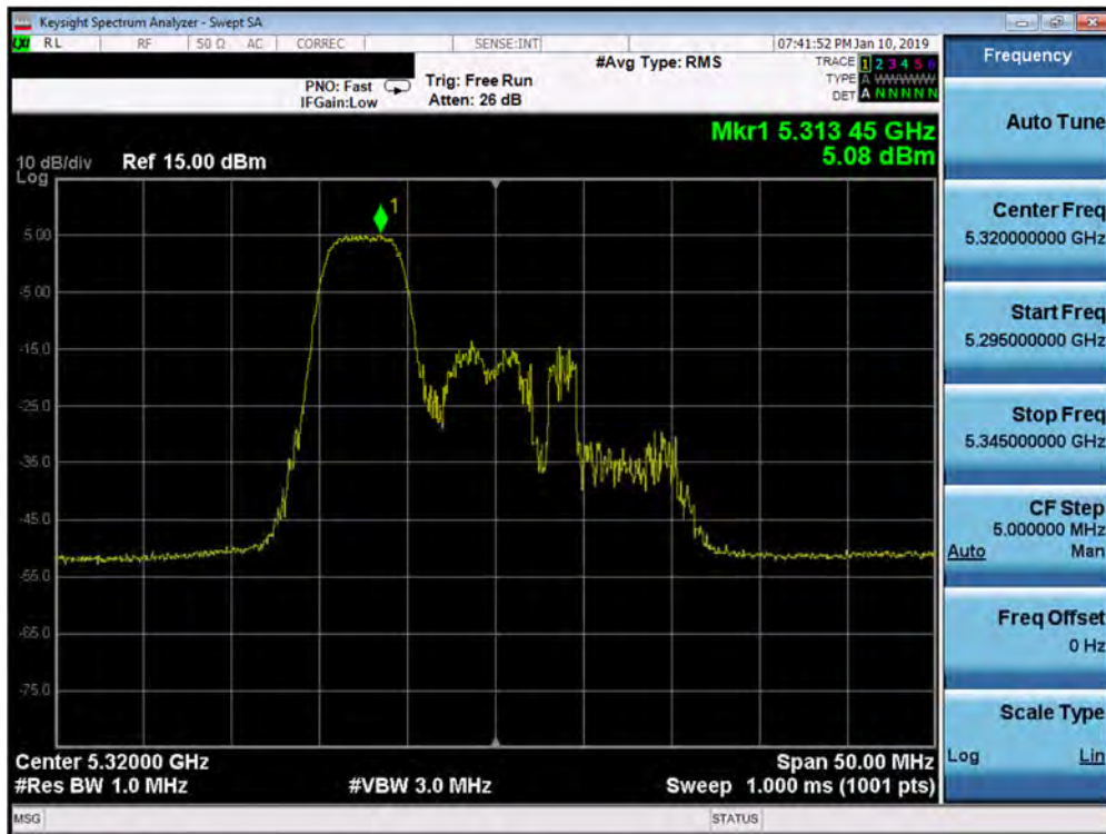
Plot 7-402. Power Spectral Density Plot MIMO ANT1 (20MHz BW 802.11ax – 52 Tones (UNII Band 2A) – Ch. 64)
