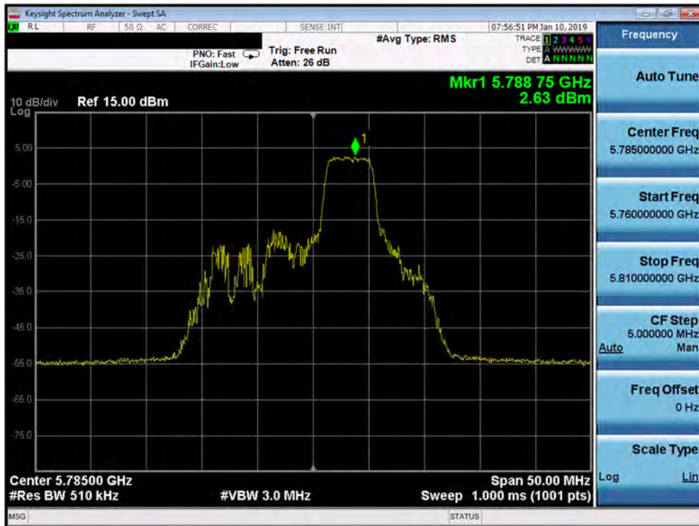
Plot 7-416. Power Spectral Density Plot MIMO ANT1 (20MHz BW 802.11ax – 52 Tones (UNII Band 3) – Ch. 157)
