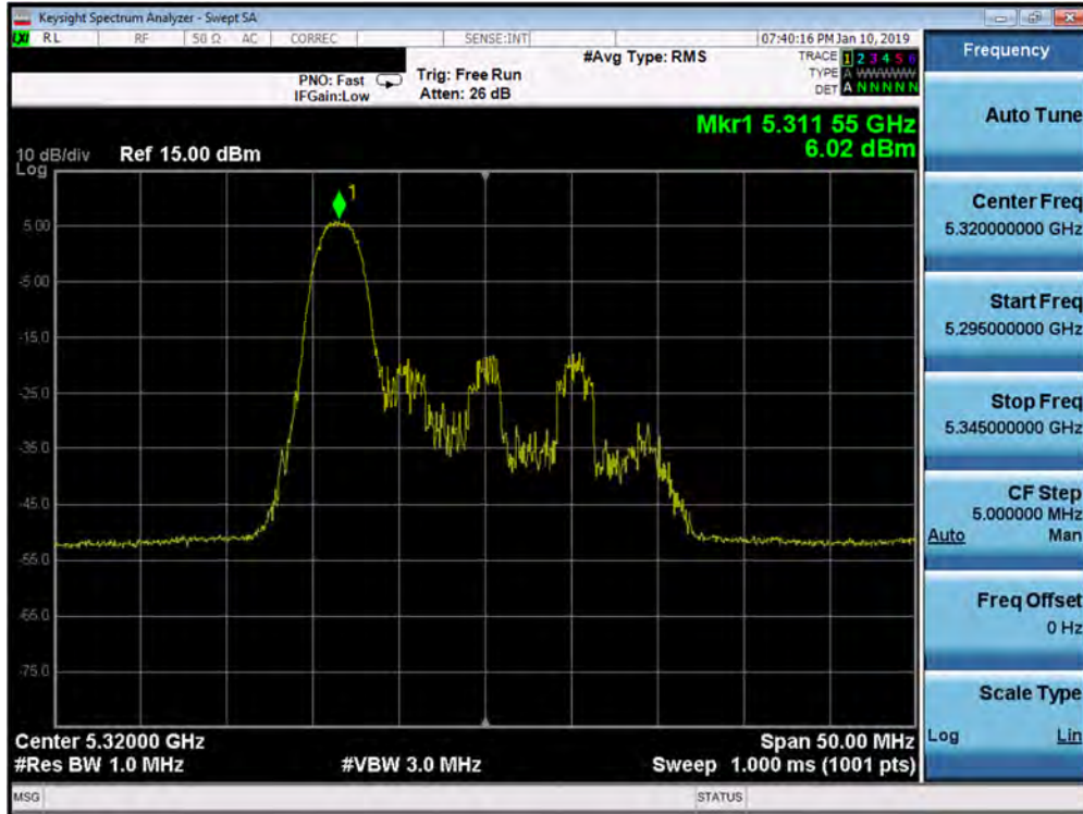
Plot 7-375. Power Spectral Density Plot MIMO ANT1 (20MHz BW 802.11ax – 26 Tones (UNII Band 2A) – Ch. 64)
