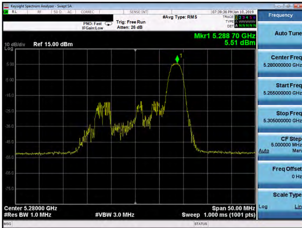
Plot 7-374. Power Spectral Density Plot MIMO ANT1 (20MHz BW 802.11ax – 26 Tones (UNII Band 2A) – Ch. 56)
