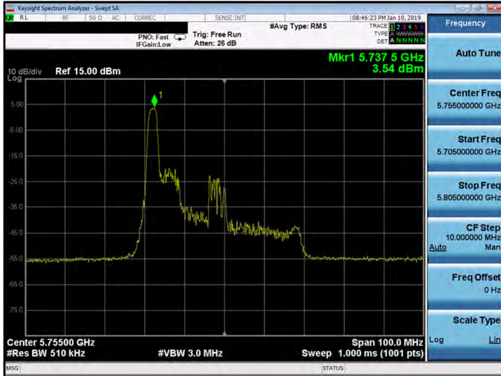
Plot 7-391. Power Spectral Density Plot MIMO ANT1 (40MHz BW 802.11ax – 26 Tones (UNII Band 3) – Ch. 151)
