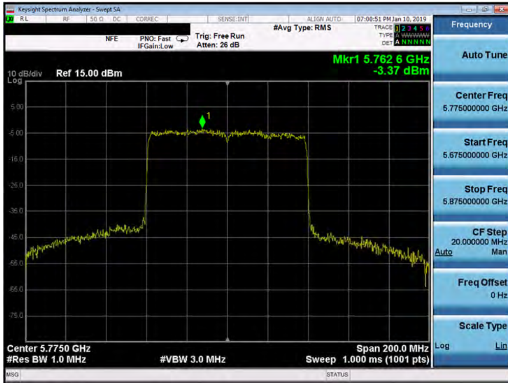
Plot 7-366. Power Spectral Density Plot SISO ANT2 (80MHz BW 802.11ax – 996 Tones (UNII Band 3) – Ch. 155)
