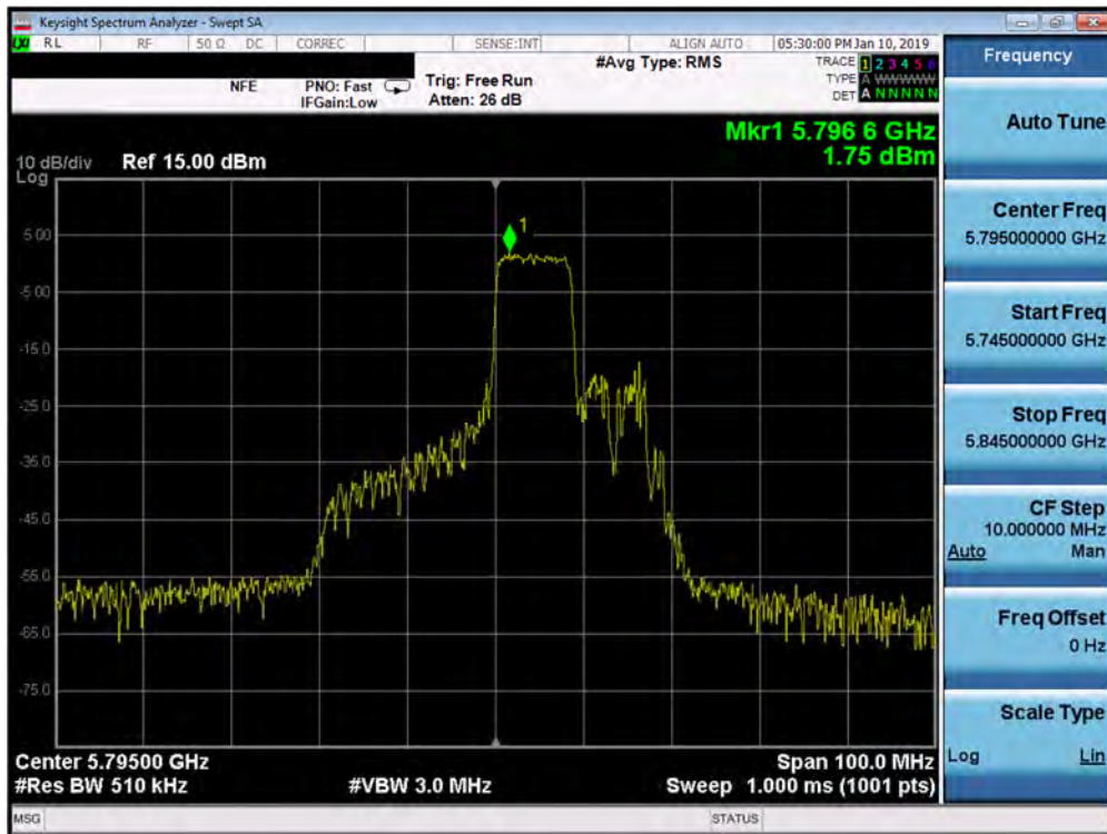
Plot 7-317. Power Spectral Density Plot SISO ANT2 (40MHz BW 802.11ax – 106 Tones (UNII Band 3) – Ch. 159)
