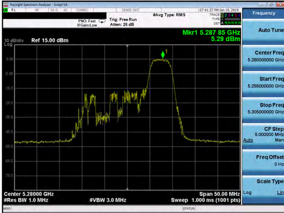
Plot 7-401. Power Spectral Density Plot MIMO ANT1 (20MHz BW 802.11ax – 52 Tones (UNII Band 2A) – Ch. 56)
