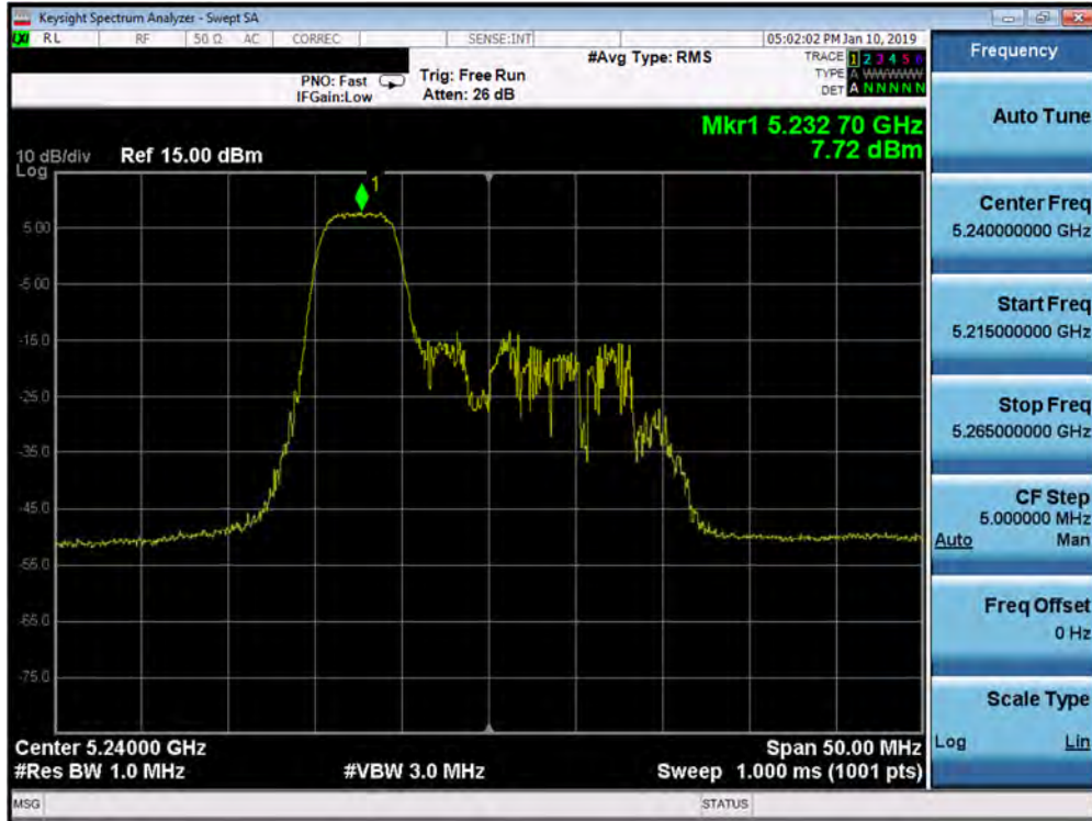
Plot 7-138. Power Spectral Density Plot SISO ANT1 (20MHz BW 802.11ax – 52 Tones (UNII Band 1) – Ch. 48)
