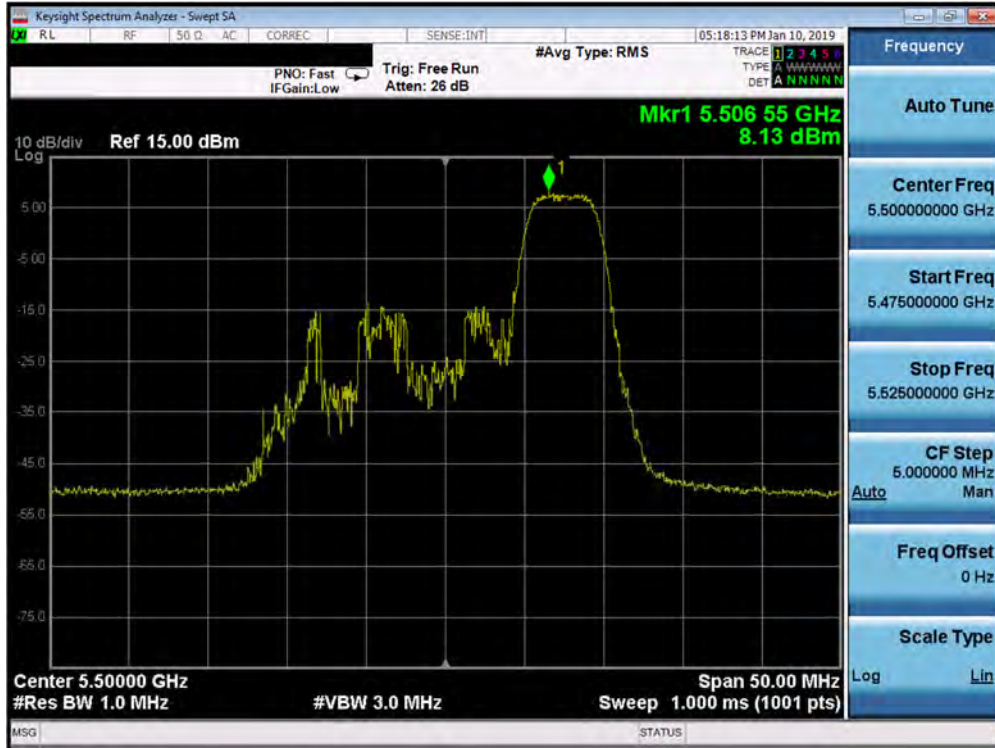
Plot 7-148. Power Spectral Density Plot SISO ANT1 (20MHz BW 802.11ax – 52 Tones (UNII Band 2C) – Ch. 100)
