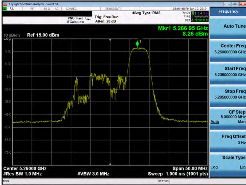
Plot 7-142. Power Spectral Density Plot SISO ANT1 (20MHz BW 802.11ax – 52 Tones (UNII Band 2A) – Ch. 52)
