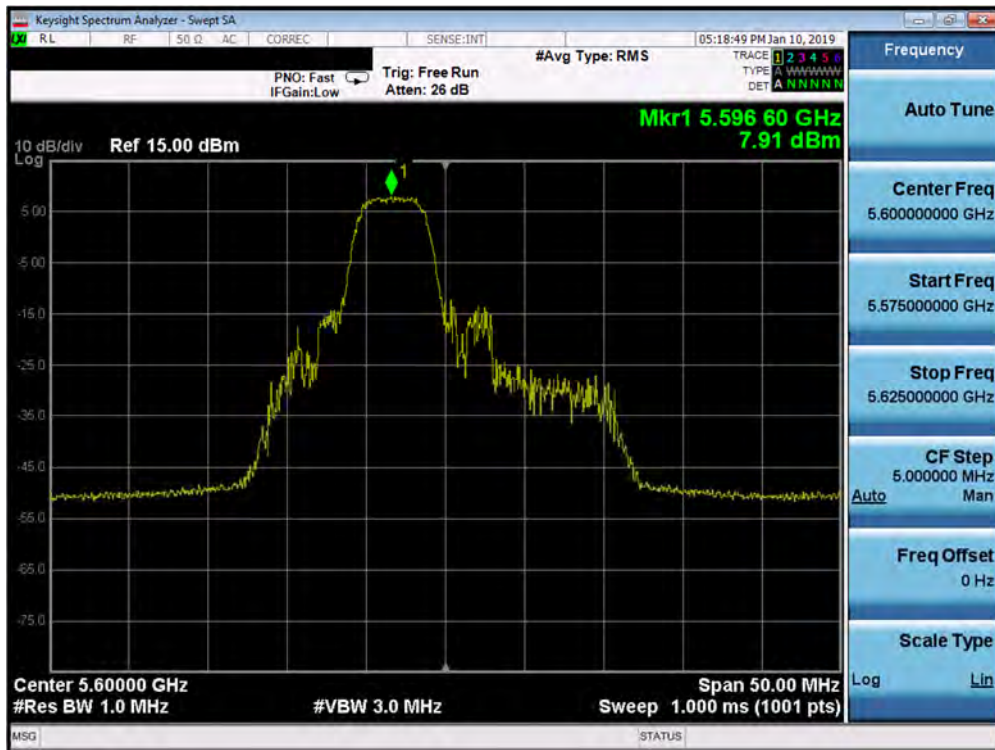
Plot 7-149. Power Spectral Density Plot SISO ANT1 (20MHz BW 802.11ax – 52 Tones (UNII Band 2C) – Ch. 120)
