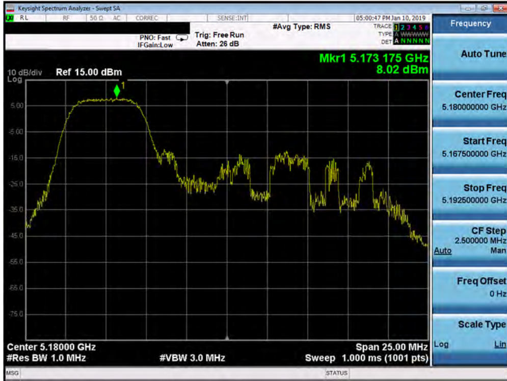
Plot 7-136. Power Spectral Density Plot SISO ANT1 (20MHz BW 802.11ax – 52 Tones (UNII Band 1) – Ch. 36)
