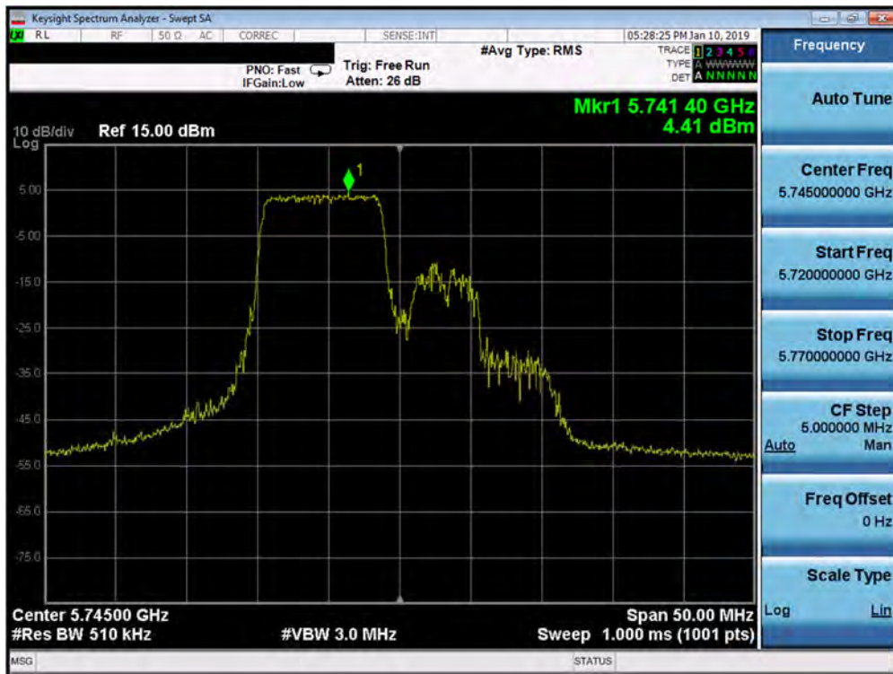
Plot 7-184. Power Spectral Density Plot SISO ANT1 (20MHz BW 802.11ax – 106 Tones (UNII Band 3) – Ch. 149)
