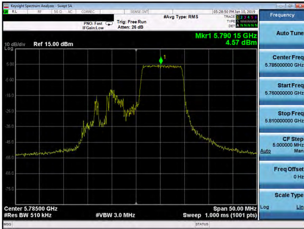
Plot 7-185. Power Spectral Density Plot SISO ANT1 (20MHz BW 802.11ax – 106 Tones (UNII Band 3) – Ch. 157)
