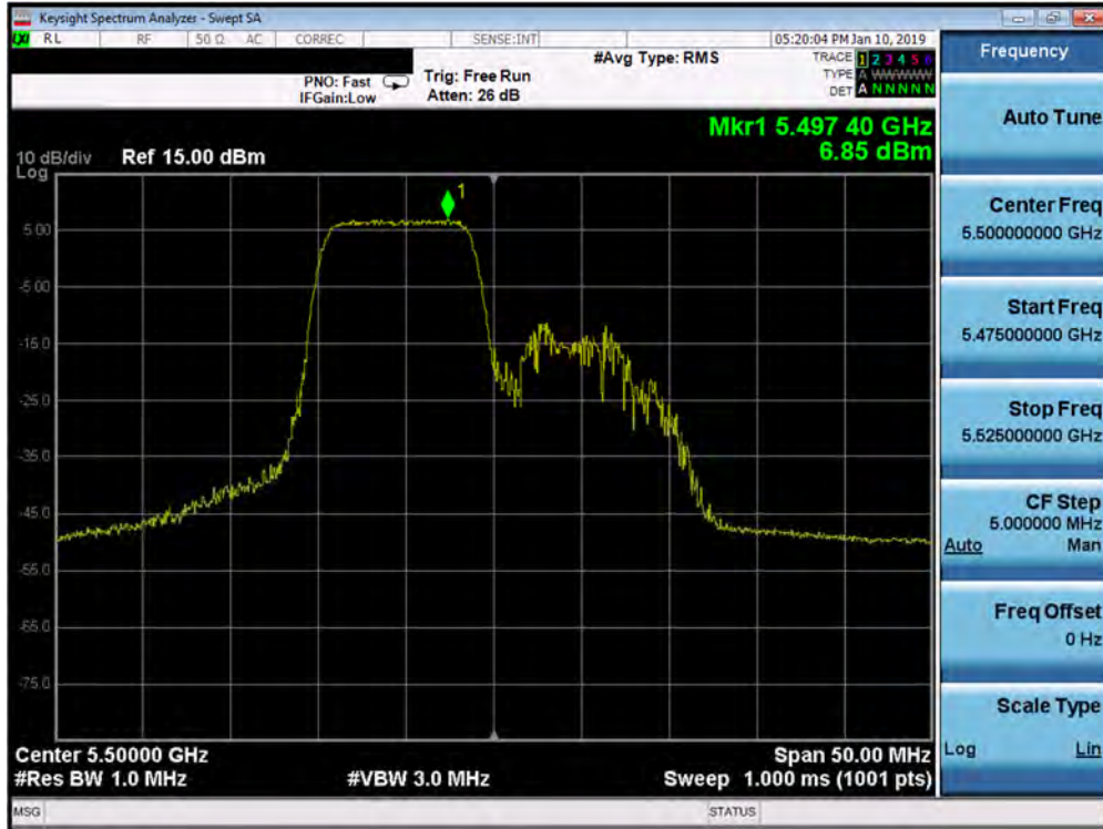
Plot 7-175. Power Spectral Density Plot SISO ANT1 (20MHz BW 802.11ax – 106 Tones (UNII Band 2C) – Ch. 100)
