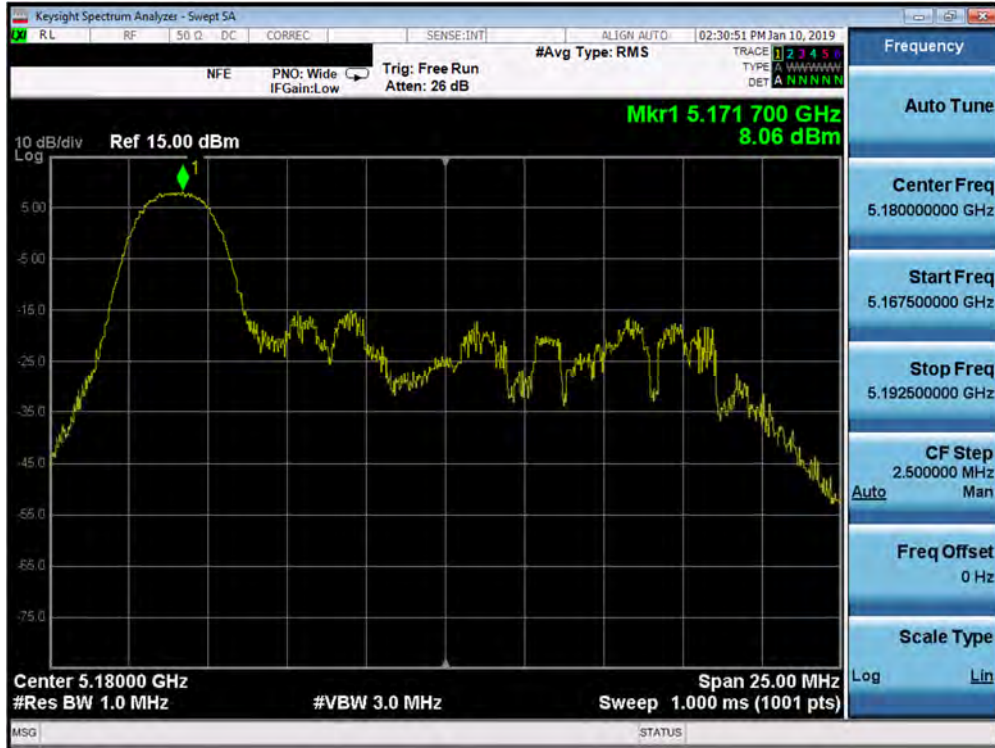
Plot 7-238. Power Spectral Density Plot SISO ANT2 (20MHz BW 802.11ax – 26 Tones (UNII Band 1) – Ch. 36)
