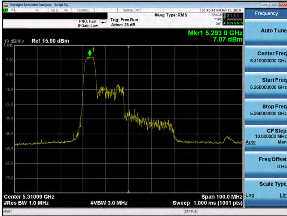
Plot 7-146. Power Spectral Density Plot SISO ANT1 (40MHz BW 802.11ax – 52 Tones (UNII Band 2A) – Ch. 62)
