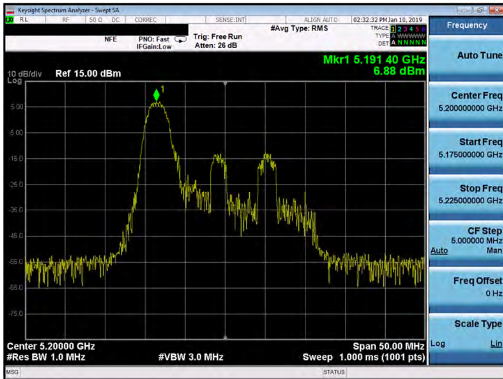
Plot 7-239. Power Spectral Density Plot SISO ANT2 (20MHz BW 802.11ax – 26 Tones (UNII Band 1) – Ch. 40)
