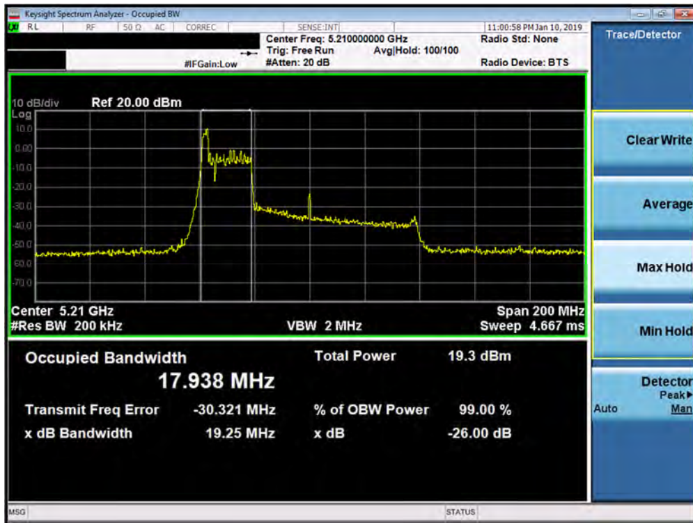
Plot 7-48. 26dB Bandwidth Plot SISO ANT2 (80MHz BW 802.11ax – 26 Tones (UNII Band 1) – Ch. 42)
