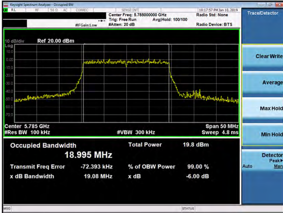
Plot 7-104. 6dB Bandwidth Plot SISO ANT2 (20MHz BW 802.11ax – 242 Tones (UNII Band 3) – Ch. 157)
