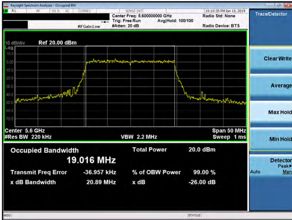
Plot 7-71. 26dB Bandwidth Plot SISO ANT2 (20MHz BW 802.11ax – 242 Tones (UNII Band 2C) – Ch. 120)
