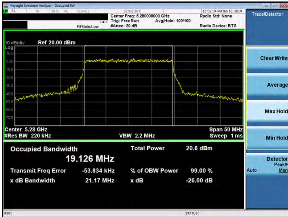
Plot 7-68. 26dB Bandwidth Plot SISO ANT2 (20MHz BW 802.11ax – 242 Tones (UNII Band 2A) – Ch. 56)
