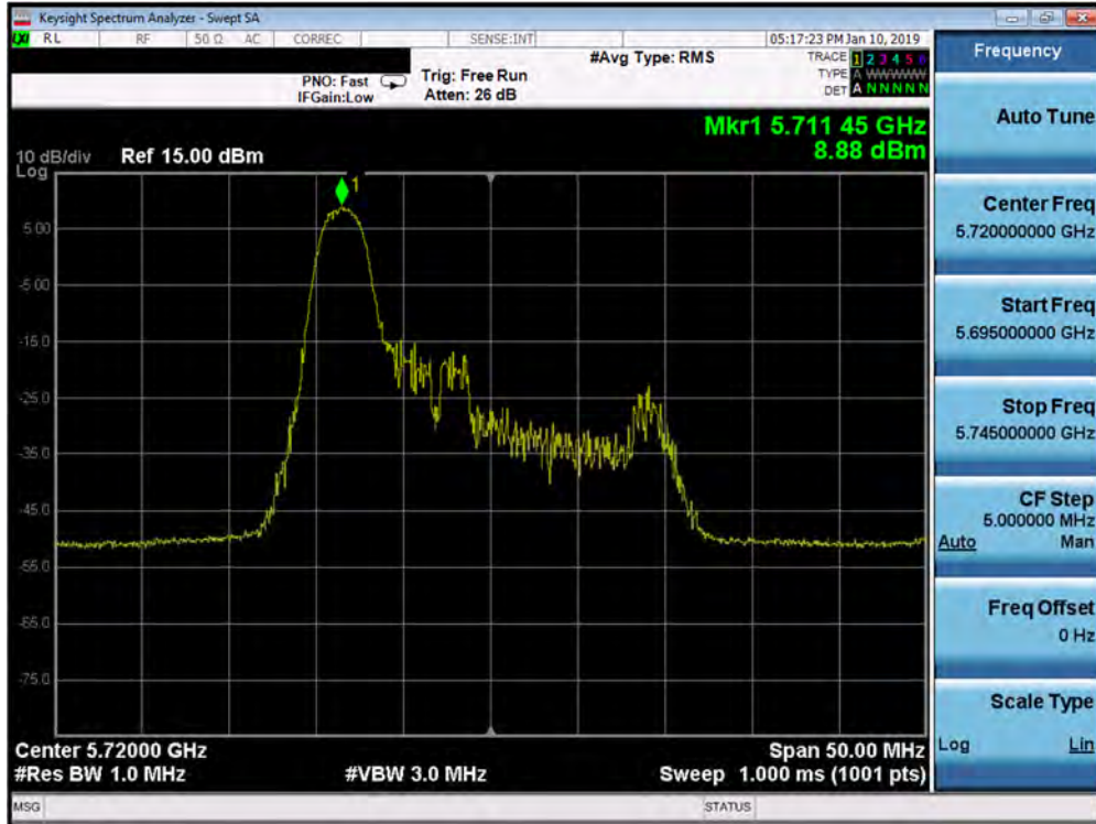
Plot 7-123. Power Spectral Density Plot SISO ANT1 (20MHz BW 802.11ax – 26 Tones (UNII Band 2C) – Ch. 144)
