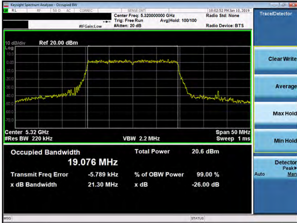
Plot 7-69. 26dB Bandwidth Plot SISO ANT2 (20MHz BW 802.11ax – 242 Tones (UNII Band 2A) – Ch. 64)
