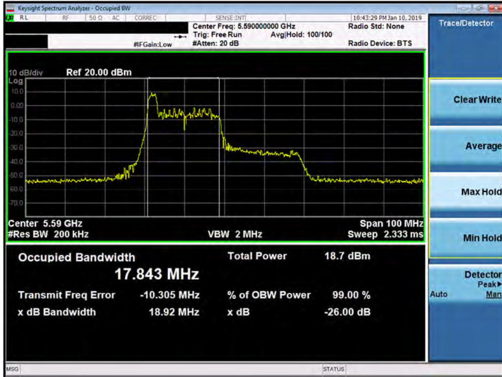
Plot 7-59. 26dB Bandwidth Plot SISO ANT2 (40MHz BW 802.11ax – 26 Tones (UNII Band 2C) – Ch. 118)
