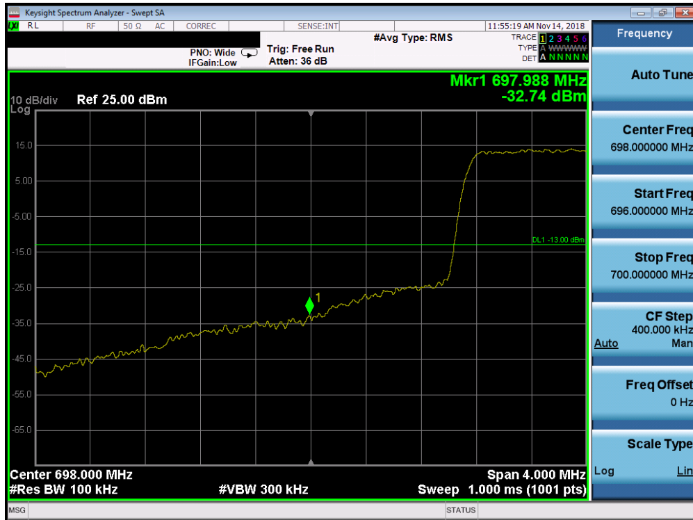
Plot 7-130. Lower Band Edge Plot (Band 12 - 1.4MHz QPSK - Full RB Configuration)
