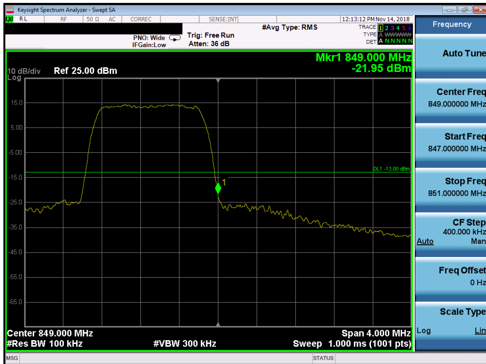
Plot 7-147. Upper Band Edge Plot (Band 26/5 - 1.4MHz QPSK - Full RB Configuration)
