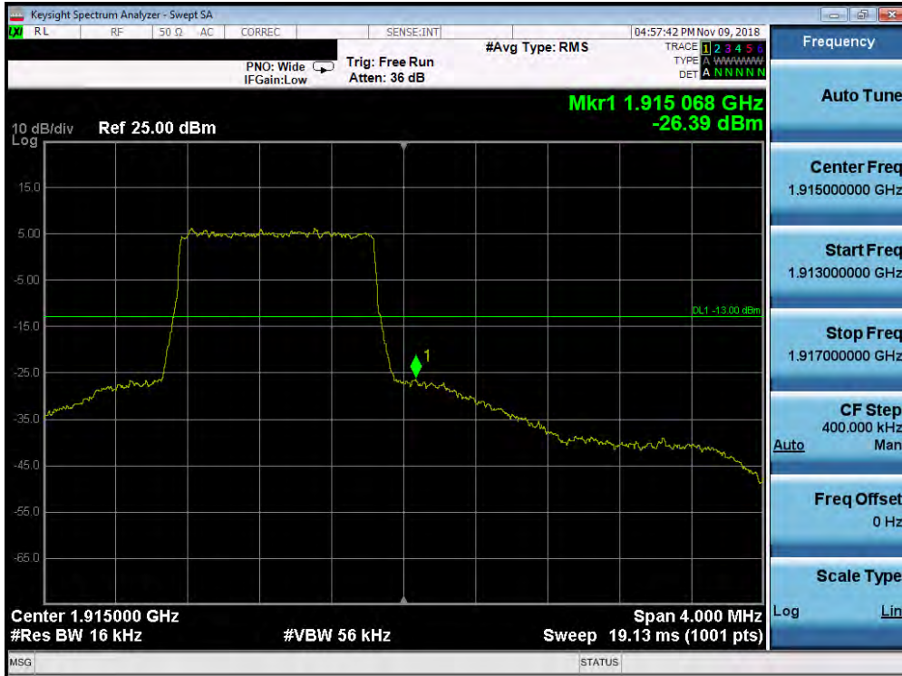
Plot 7-184. Upper Band Edge Plot (Band 25 - 1.4MHz QPSK - Full RB Configuration)
