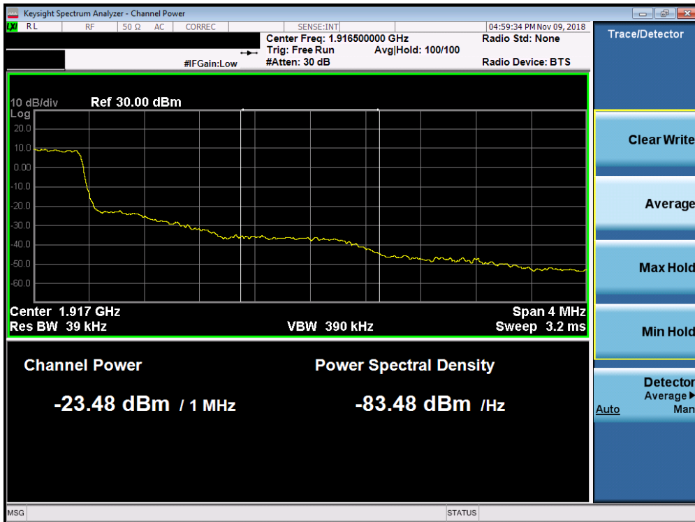
Plot 7-185. Upper Extended Band Edge Plot (Band 25 - 1.4MHz QPSK - Full RB Configuration)
