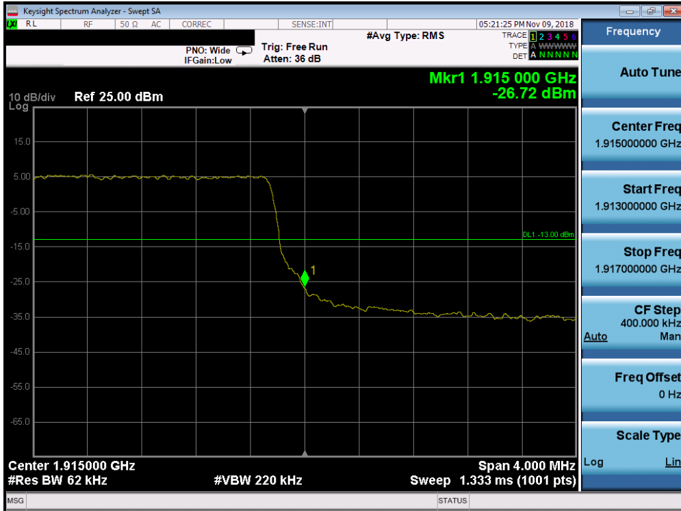
Plot 7-196. Upper Band Edge Plot (Band 25 - 5.0MHz QPSK - Full RB Configuration)
