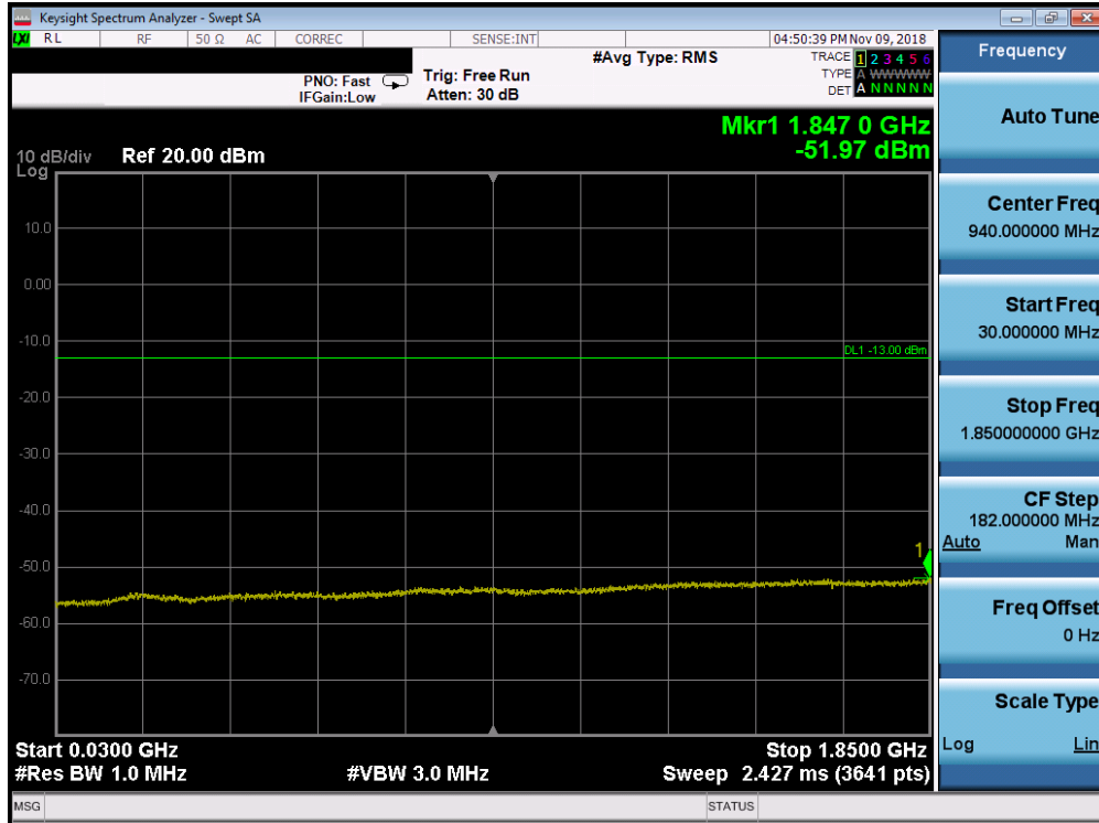
Plot 7-118. Conducted Spurious Plot (Band 25/2 - 20.0MHz QPSK - RB Size 1, RB Offset 0 - High Channel)
