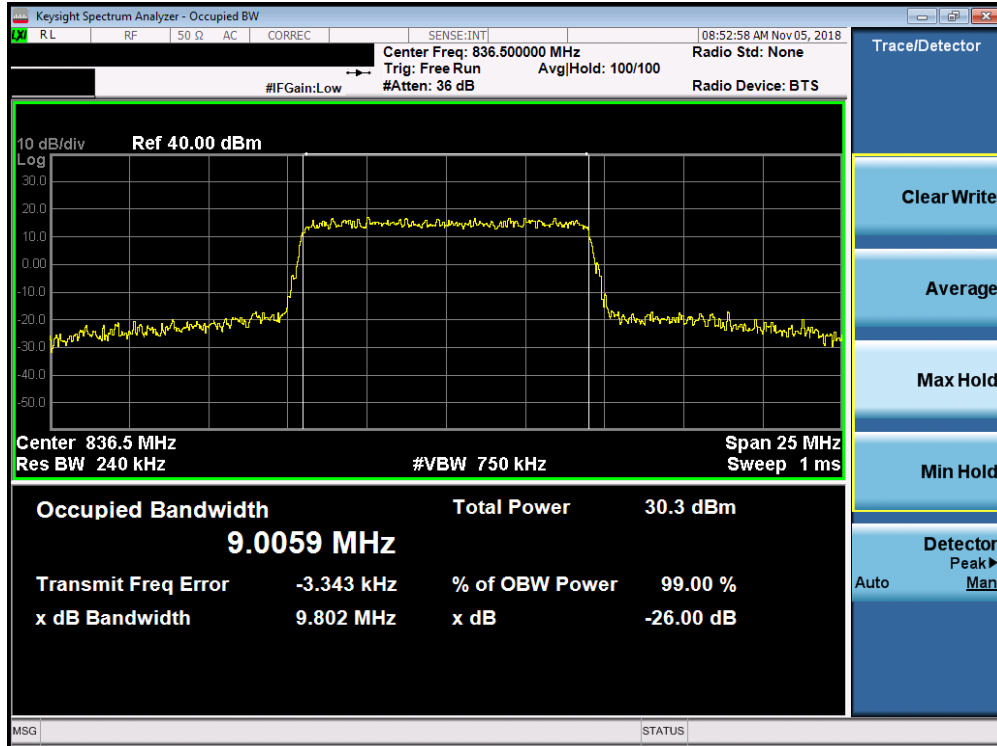
Plot 7-29. Occupied Bandwidth Plot (Band 26/5 - 10.0MHz 16-QAM - Full RB Configuration)
