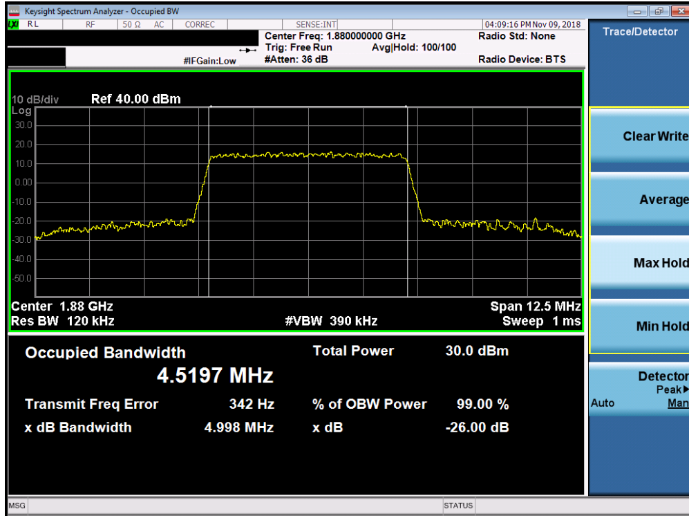
Plot 7-60. Occupied Bandwidth Plot (Band 2/25 - 5.0MHz 64-QAM - Full RB Configuration)
