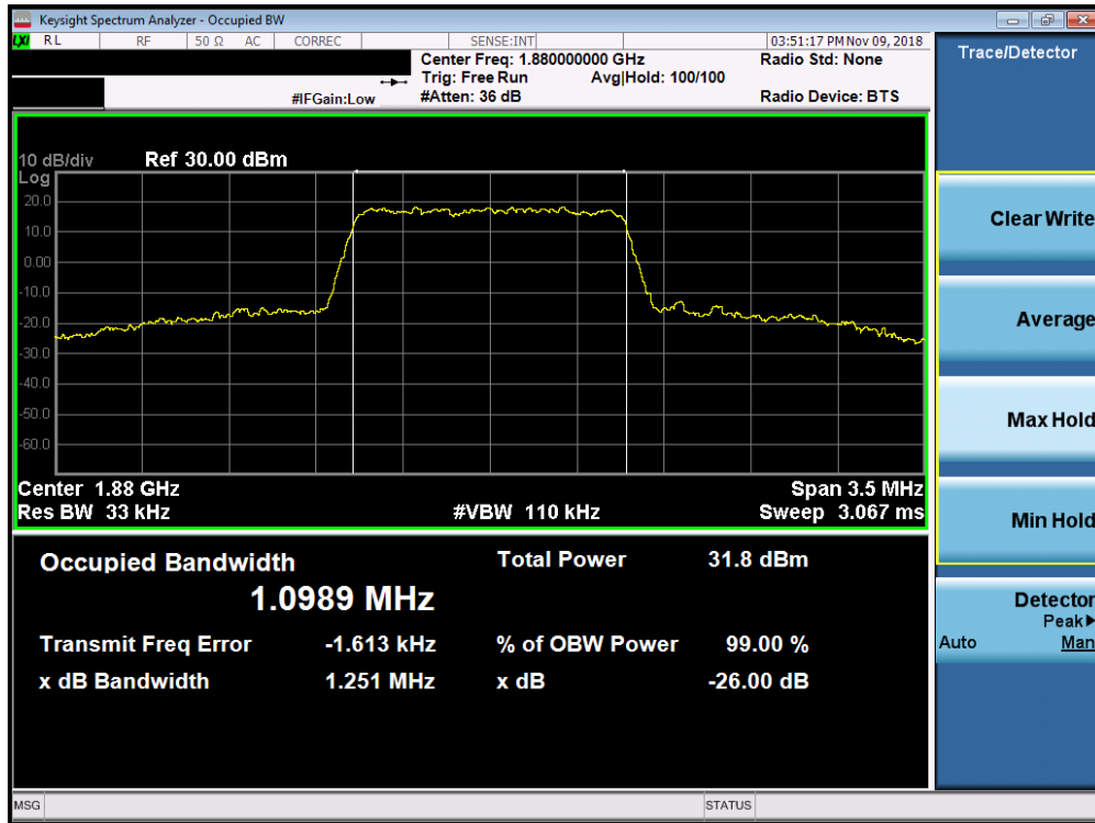
Plot 7-52. Occupied Bandwidth Plot (Band 2/25 - 1.4MHz QPSK - Full RB Configuration)
