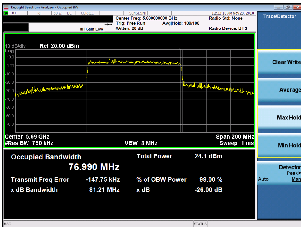
Plot 7-102. 26dB Bandwidth Plot SISO ANT2 (80MHz BW 802.11ax (UNII Band 2C) – Ch. 138)
