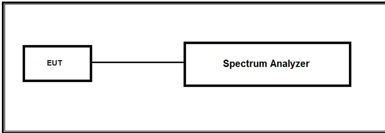
**SETUP DIAGRAM FOR TESTS (RADIATED TEST SETUP)**
