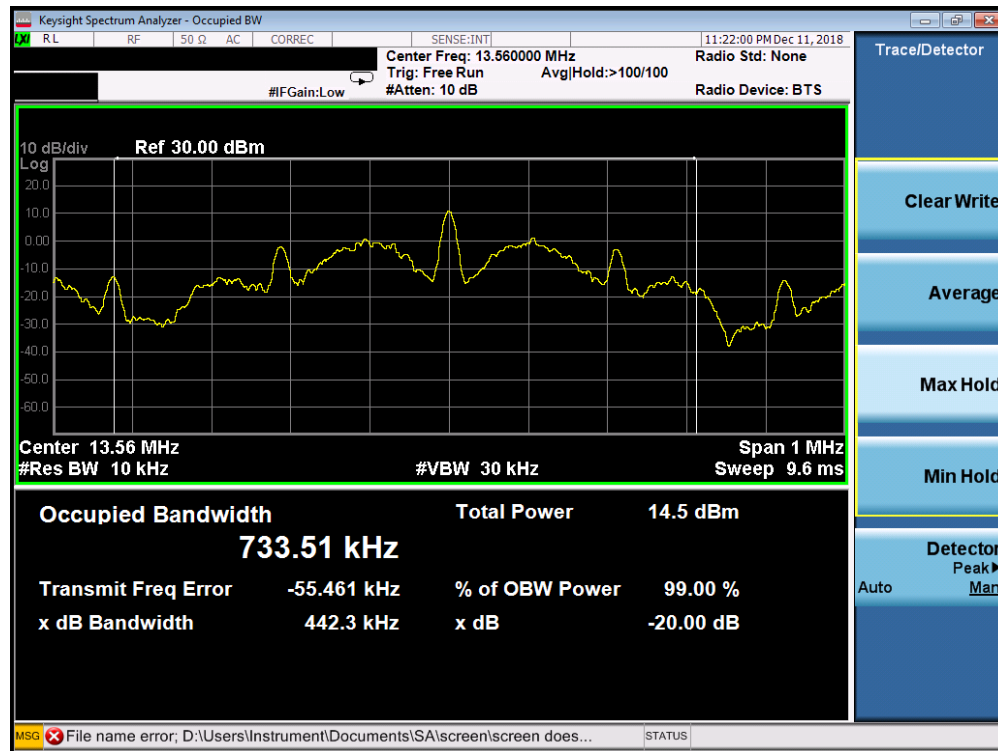
Figure 7-2. Occupied Bandwidth Plot
