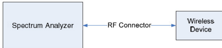
Figure 7-1. Test Instrument & Measurement Setup
