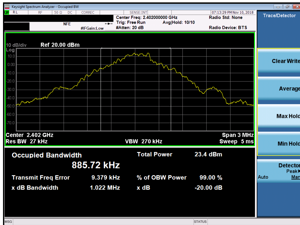
Plot 7-1. 20dB Bandwidth Plot (Bluetooth, 1Mbps – Ch. 0)
