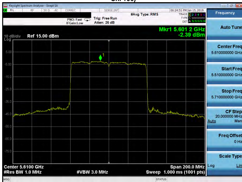
Plot 7-622. Power Spectral Density Plot MIMO ANT2 (80MHz BW 802.11ax – 996 Tones (UNII Band 2C) – Ch. 122)
