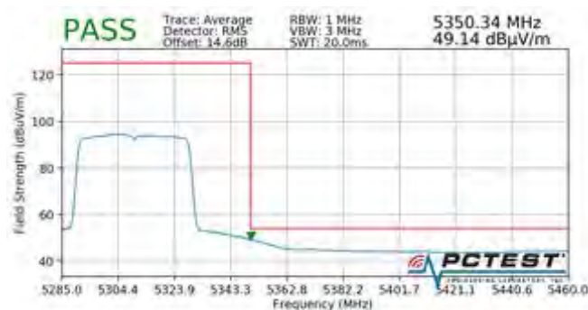
Plot 7-686. Radiated Upper Band Edge Plot SISO ANT1 (Average – UNII Band 2A – 484 Tones)
