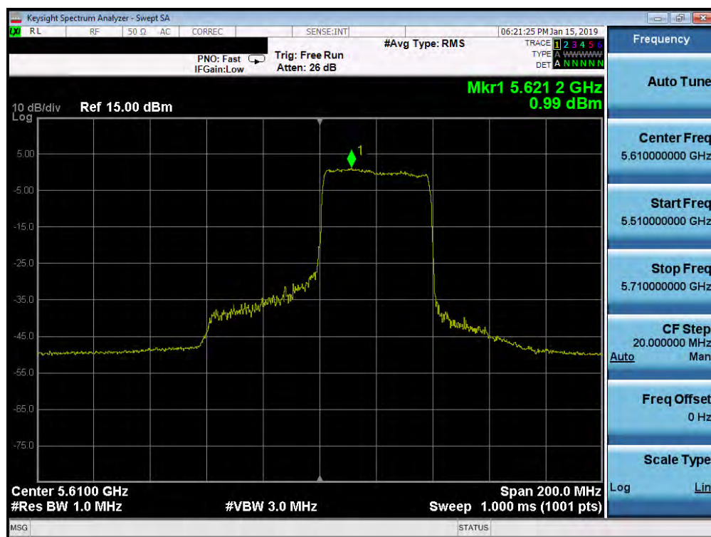
Plot 7-614. Power Spectral Density Plot MIMO ANT2 (80MHz BW 802.11ax – 484 Tones (UNII Band 2C) – Ch. 122)
