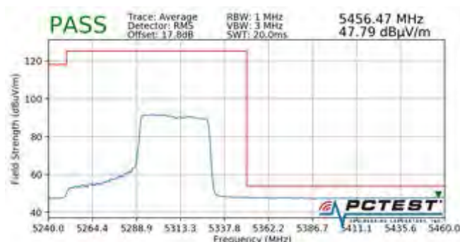
Plot 7-791. Radiated Upper Band Edge Plot MIMO (Average – UNII Band 2A – 484 Tones)
