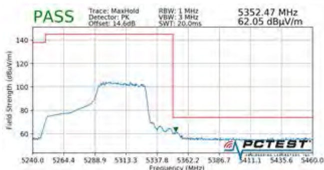
Plot 7-696. Radiated Upper Band Edge Plot SISO ANT1 (Peak – UNII Band 2A – 484 Tones)
