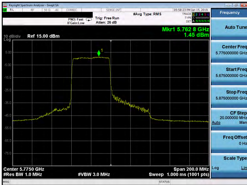
Plot 7-618. Power Spectral Density Plot MIMO ANT2 (80MHz BW 802.11ax – 484 Tones (UNII Band 3) – Ch. 155)
