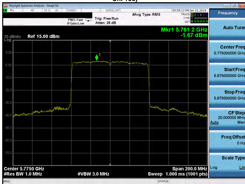
Plot 7-624. Power Spectral Density Plot MIMO ANT2 (80MHz BW 802.11ax – 996 Tones (UNII Band 3) – Ch. 155)
