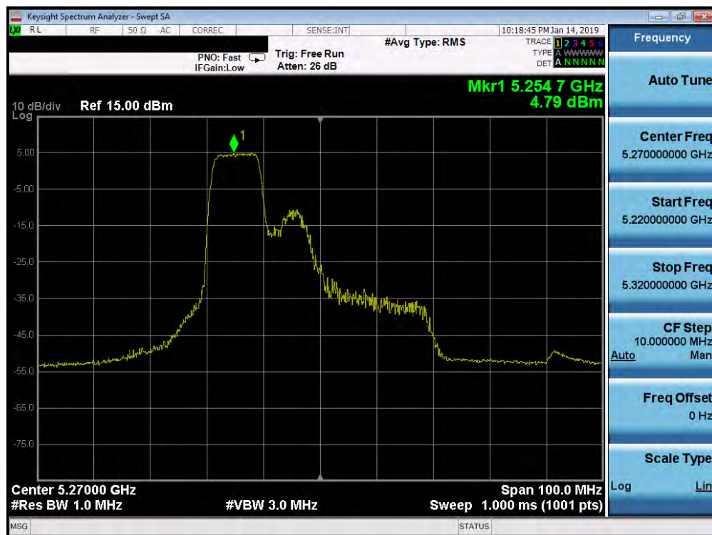
Plot 7-430. Power Spectral Density Plot MIMO ANT1 (40MHz BW 802.11ax – 106 Tones (UNII Band 2A) – Ch. 54)
