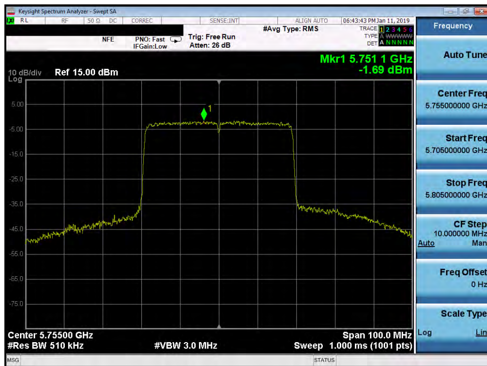
Plot 7-229. Power Spectral Density Plot SISO ANT1 (40MHz BW 802.11ax – 484 Tones (UNII Band 3) – Ch. 151)
