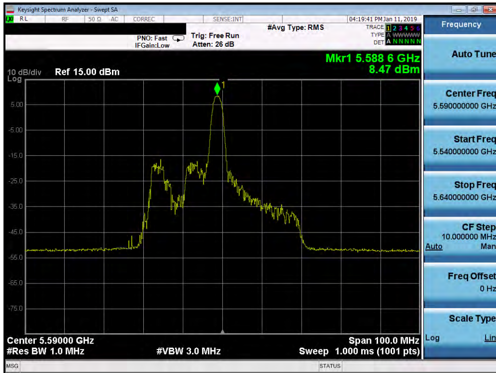
Plot 7-254. Power Spectral Density Plot SISO ANT2 (40MHz BW 802.11ax – 26 Tones (UNII Band 2C) – Ch. 118)
