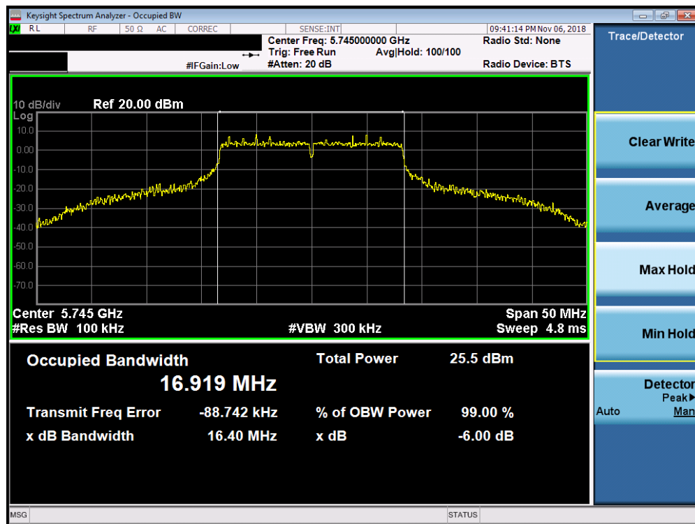
Plot 7-118. 6dB Bandwidth Plot SISO ANT2 (802.11a (UNII Band 3) - Ch. 149)
