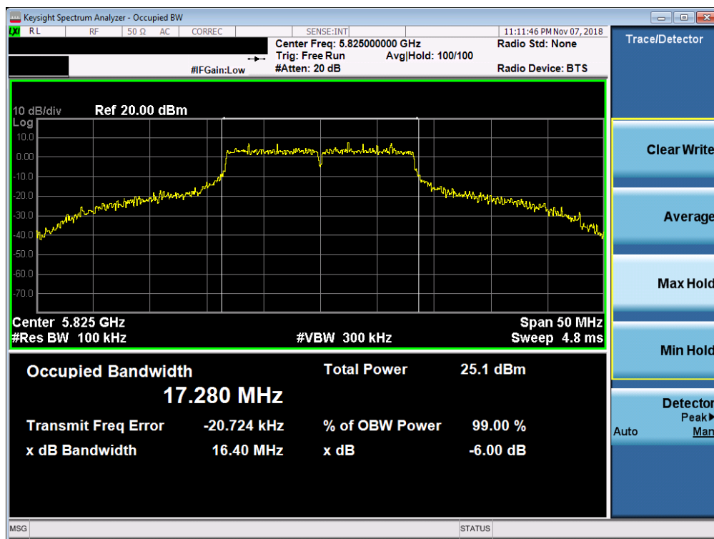
Plot 7-105. 6dB Bandwidth Plot SISO ANT1 (802.11a (UNII Band 3) – Ch. 165)
