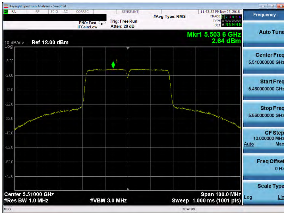
Plot 7-172. Power Spectral Density Plot SISO ANT1 (40MHz BW 802.11n (UNII Band 2C) – Ch. 102)
