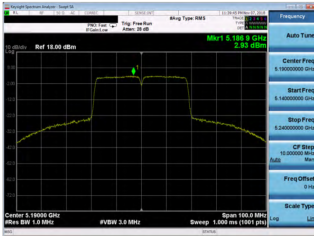
Plot 7-142. Power Spectral Density Plot SISO ANT1 (40MHz BW 802.11n (UNII Band 1) – Ch. 38)
