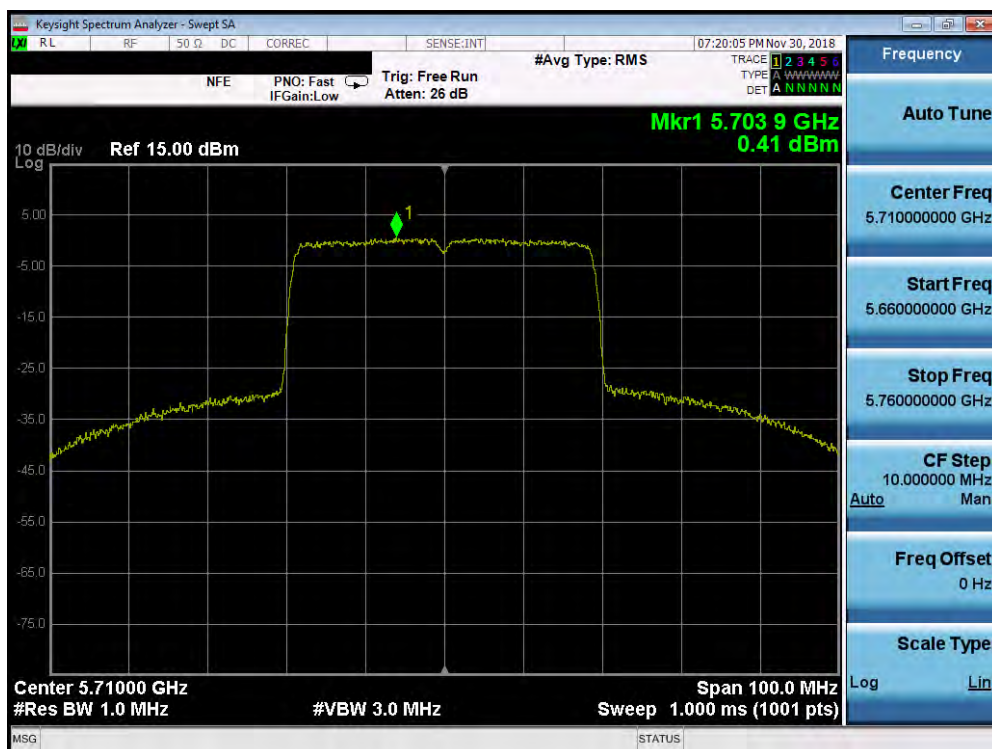
Plot 7-177. Power Spectral Density Plot SISO ANT1 (40MHz BW 802.11ax (UNII Band 2C) – Ch. 142)
