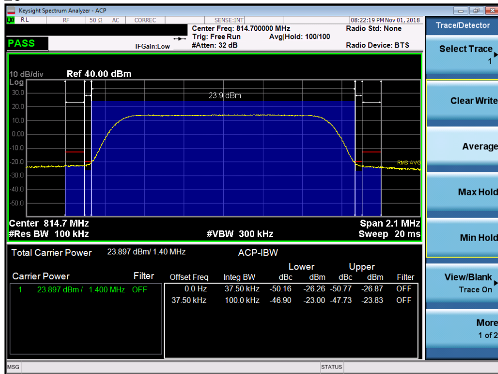
Plot 7-19. Channel Edge Plot (LTE Band 26, 1.4MHz QPSK – RB Size 6– Low Channel)
