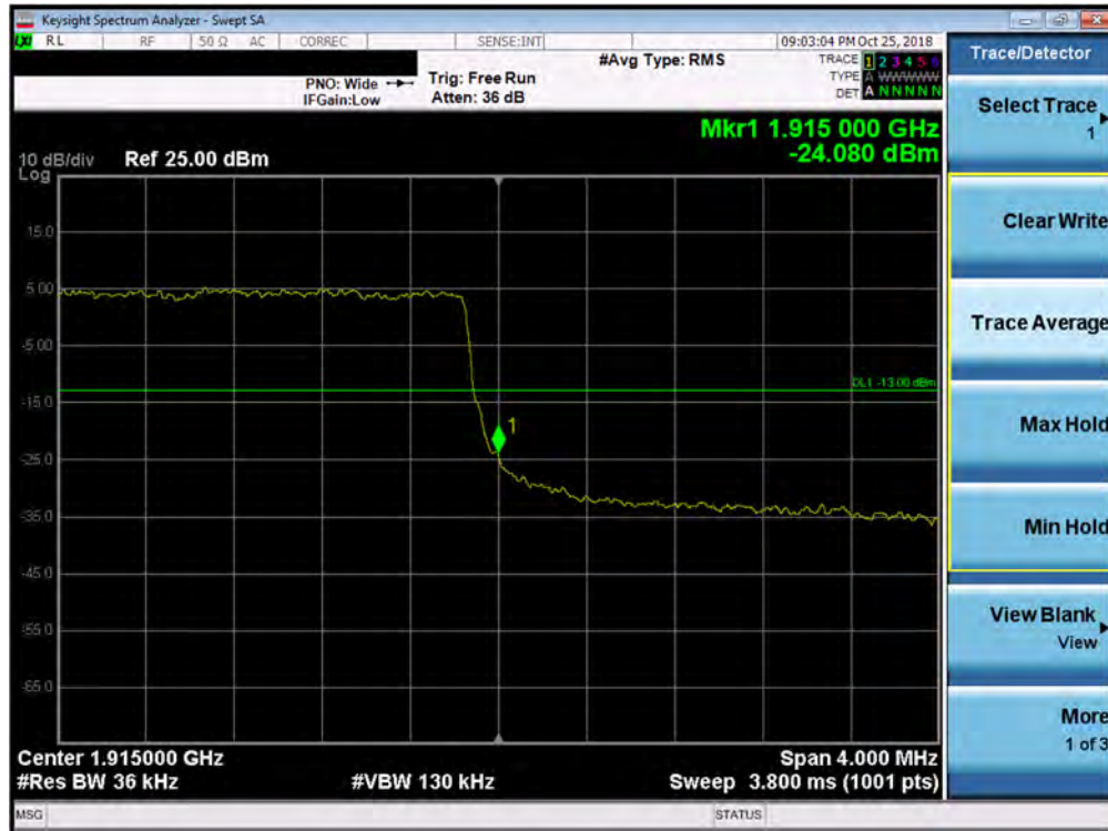
Plot 7-186. Upper Band Edge Plot (Band 25/2 - 3.0MHz QPSK - Full RB Configuration)
