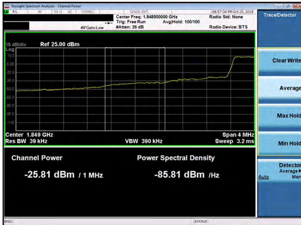
Plot 7-181. Lower Extended Band Edge Plot (Band 25/2 - 1.4MHz QPSK - Full RB Configuration)
