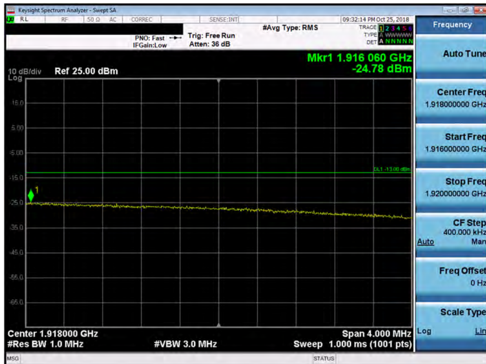
Plot 7-203. Upper Extended Band Edge Plot (Band 25/2 - 20.0MHz QPSK - Full RB Configuration)
