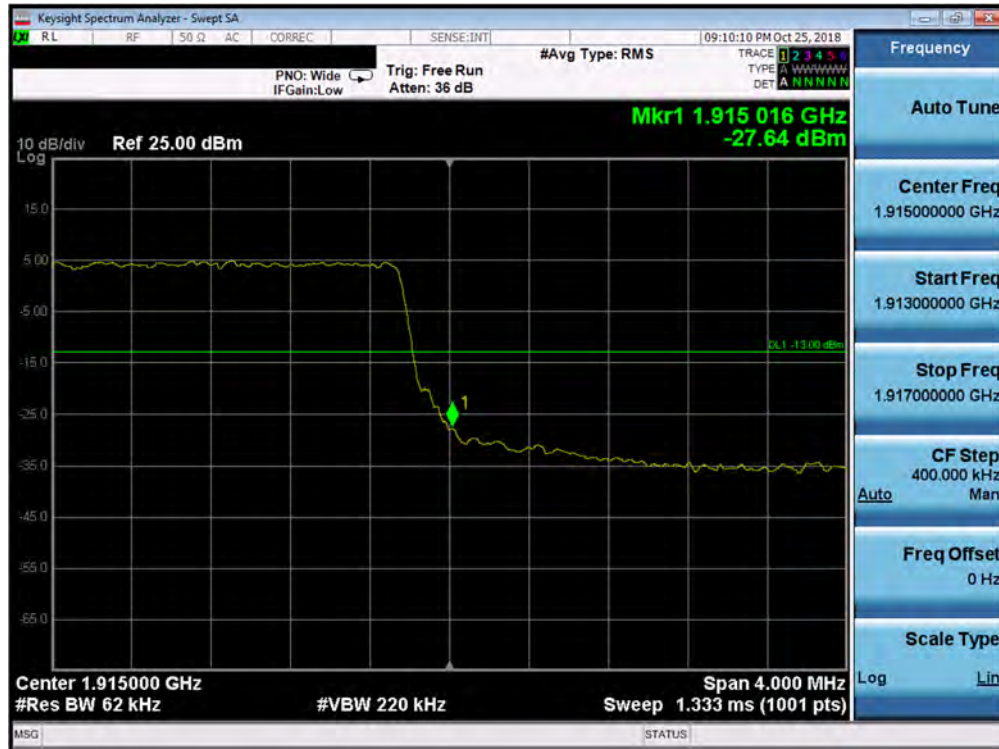
Plot 7-190. Upper Band Edge Plot (Band 25/2 - 5.0MHz QPSK - Full RB Configuration)
