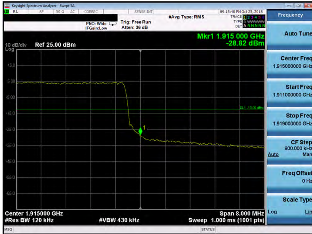
Plot 7-194. Upper Band Edge Plot (Band 25/2 - 10.0MHz QPSK - Full RB Configuration)
