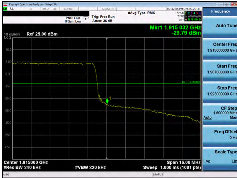
Plot 7-202. Upper Band Edge Plot (Band 25/2 - 20.0MHz QPSK - Full RB Configuration)
