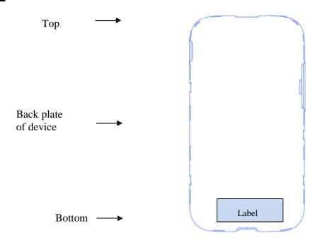
FCC ID is engraved on rear bottom of the device.
