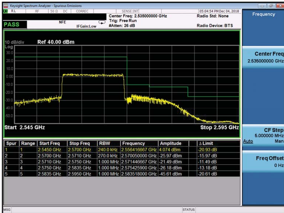
Plot 7-401. Upper ACP Plot (Band 7 Ant A - 15.0MHz QPSK - Full RB Configuration)
