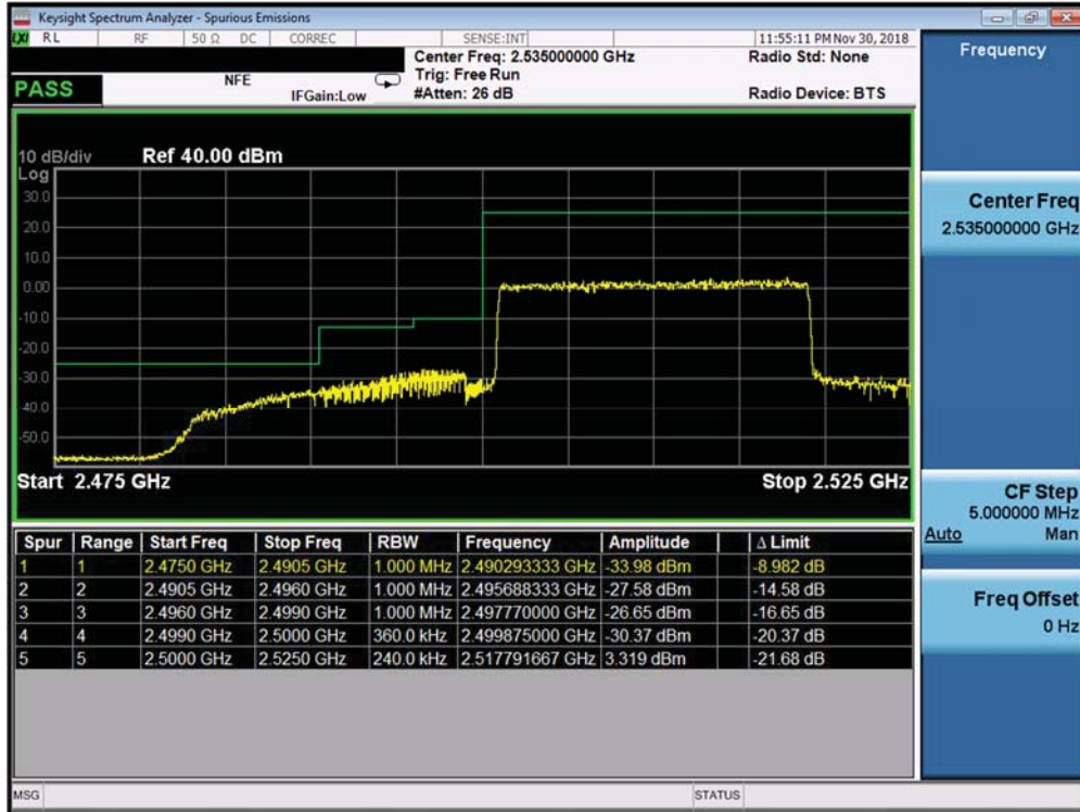
Plot 7-394. Lower ACP Plot (Band 7 ANT B - 20.0MHz QPSK - Full RB Configuration)
