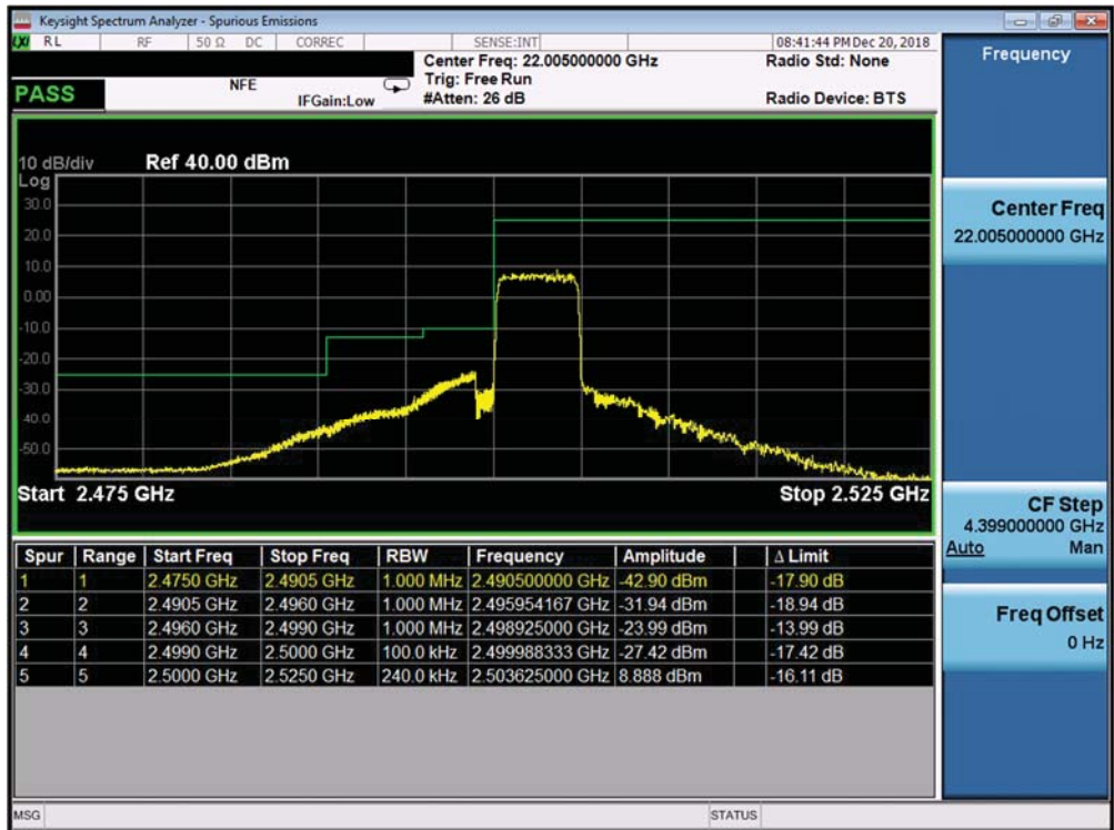
Plot 7-388. Lower ACP Plot (Band 7 ANT B - 5.0MHz QPSK - Full RB Configuration)
