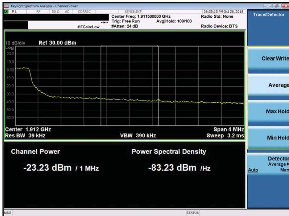
Plot 7-359. Upper Extended Band Edge Plot (Band 2 - 5.0MHz QPSK - Full RB Configuration)
