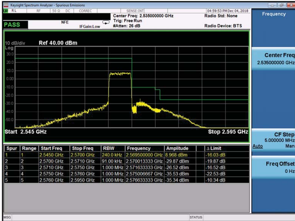
Plot 7-397. Upper ACP Plot (Band 7 Ant A - 5.0MHz QPSK - Full RB Configuration)
