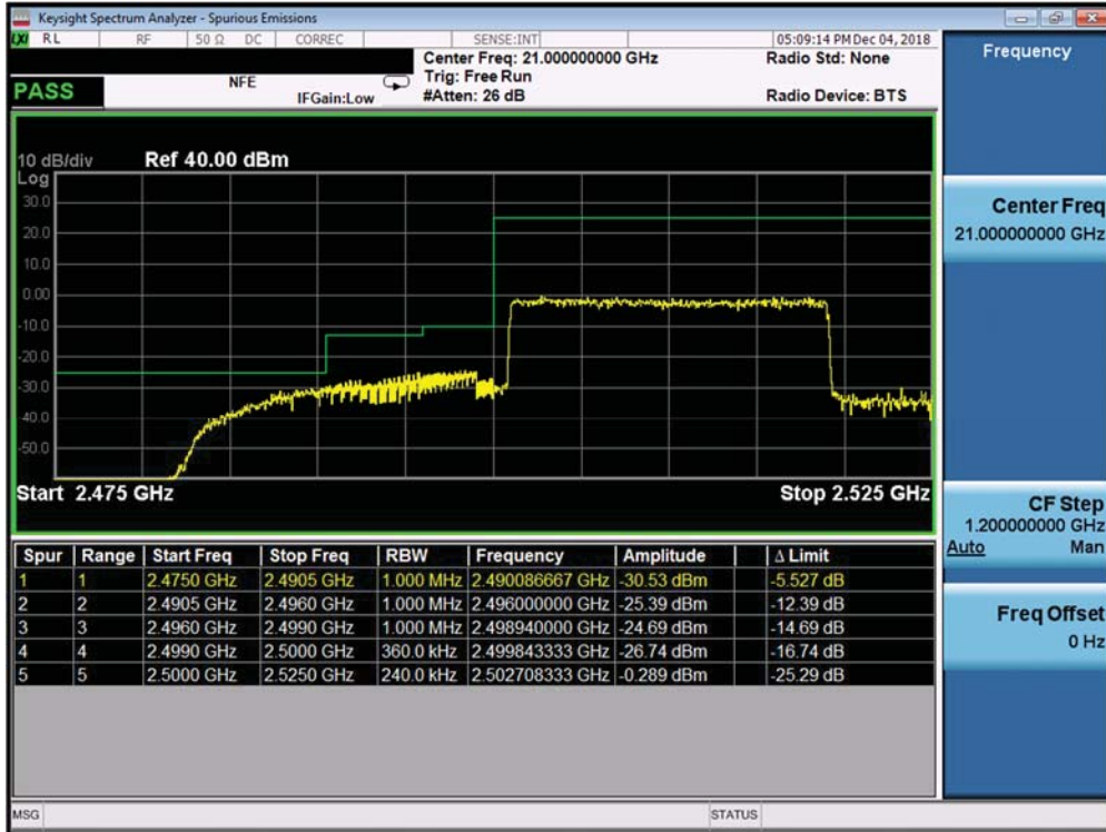
Plot 7-402. Lower ACP Plot (Band 7 Ant A - 20.0MHz QPSK - Full RB Configuration)
