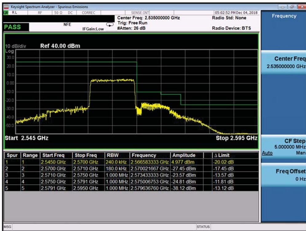
Plot 7-399. Upper ACP Plot (Band 7 Ant A - 10.0MHz QPSK - Full RB Configuration)
