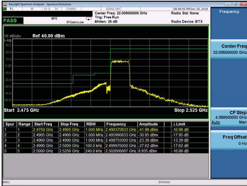
Plot 7-396. Lower ACP Plot (Band 7 Ant A - 5.0MHz QPSK - Full RB Configuration)
