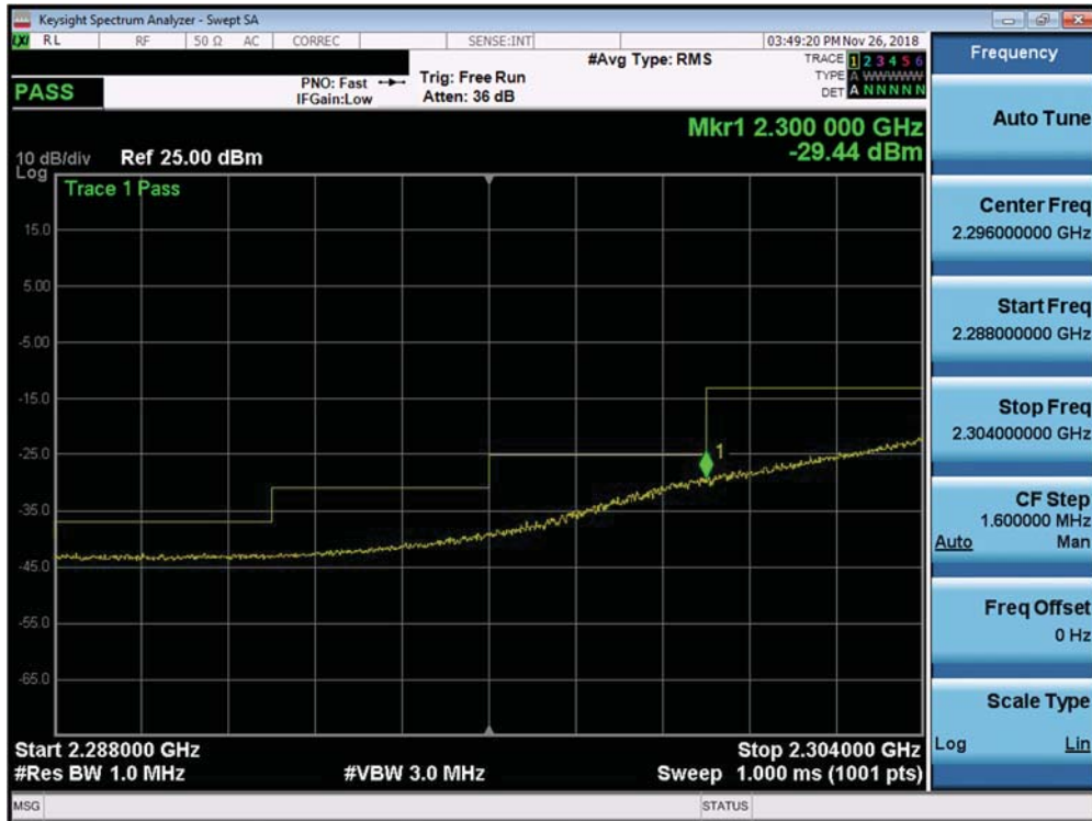
Plot 7-385. Lower Extended Band Edge Plot (Band 30 - 10.0MHz QPSK - Full RB Configuration)
