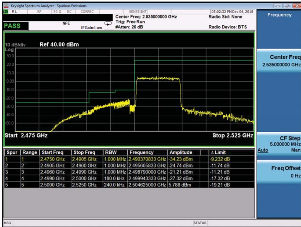
Plot 7-398. Lower ACP Plot (Band 7 Ant A - 10.0MHz QPSK - Full RB Configuration)
