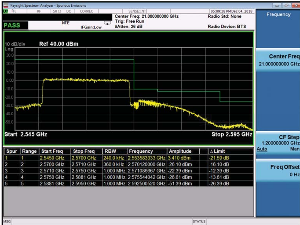
Plot 7-403. Upper ACP Plot (Band 7 Ant A - 20.0MHz QPSK - Full RB Configuration)
