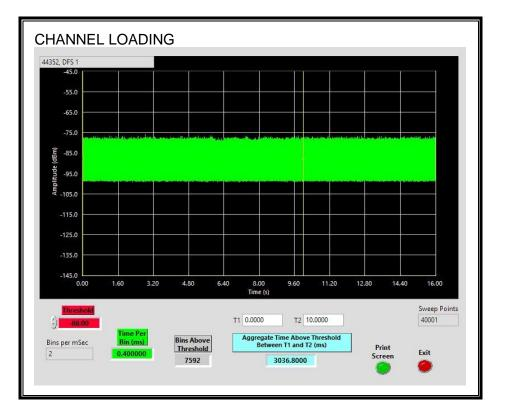
The level of traffic loading on the channel by the EUT is 30.368%.
