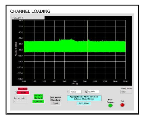
The level of traffic loading on the channel by the EUT is 31.332%.
