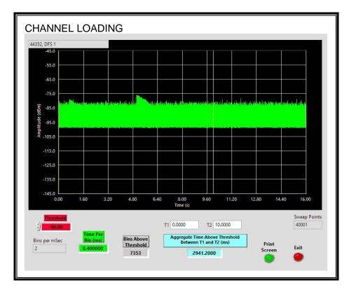
The level of traffic loading on the channel by the EUT is 29.412%.
