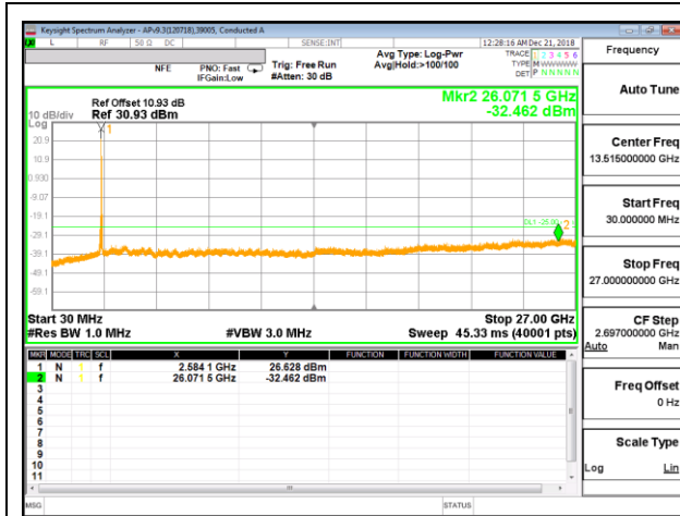
LTE B38 20MHz + 20MHz QPSK Low Channel RB1-99 + RB1-0
