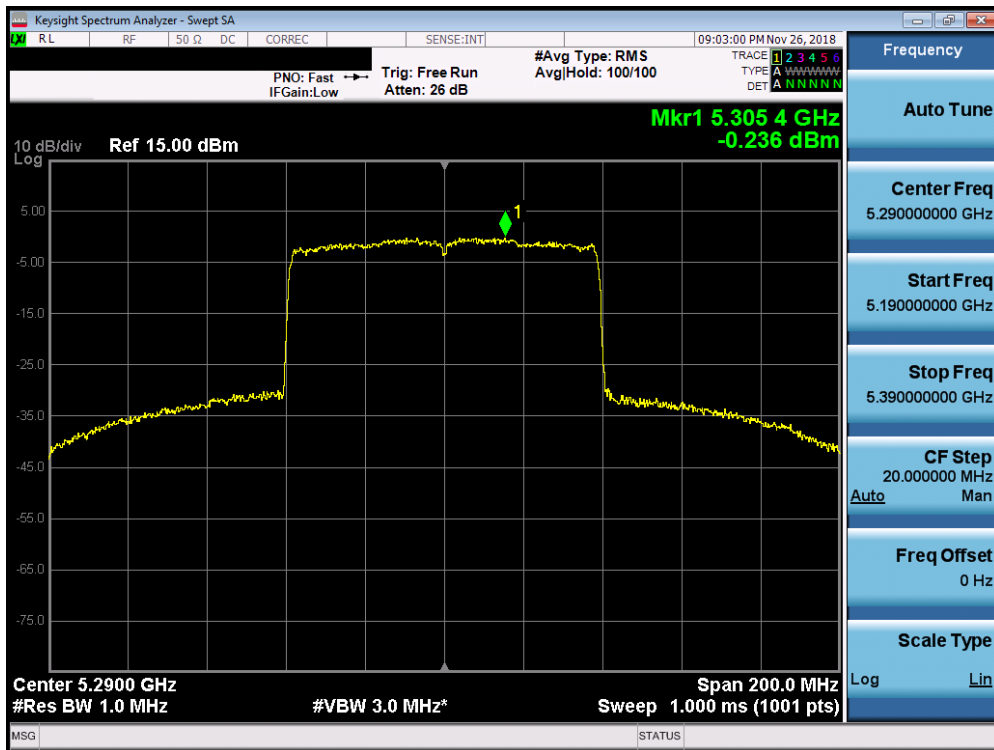
Plot 7-162. Power Spectral Density Plot SISO ANT1 (80MHz BW 802.11ax (UNII Band 2A) – Ch. 58)
