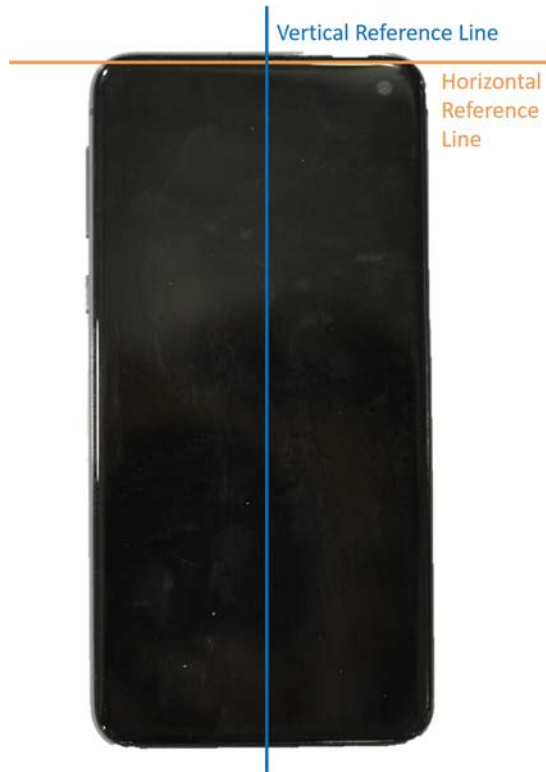
SAR Test Setup Photo 13 – Horizontal and Vertical Reference Lines
