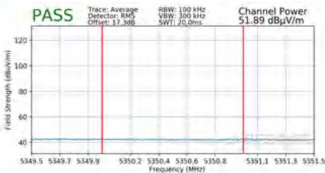
Plot 7-297. Radiated Upper Band Edge Plot SISO ANT1 (Average – UNII Band 2A)
