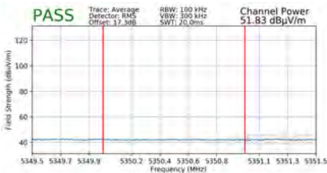
Plot 7-333. Radiated Upper Band Edge Plot SISO ANT2 (Average – UNII Band 2A)
