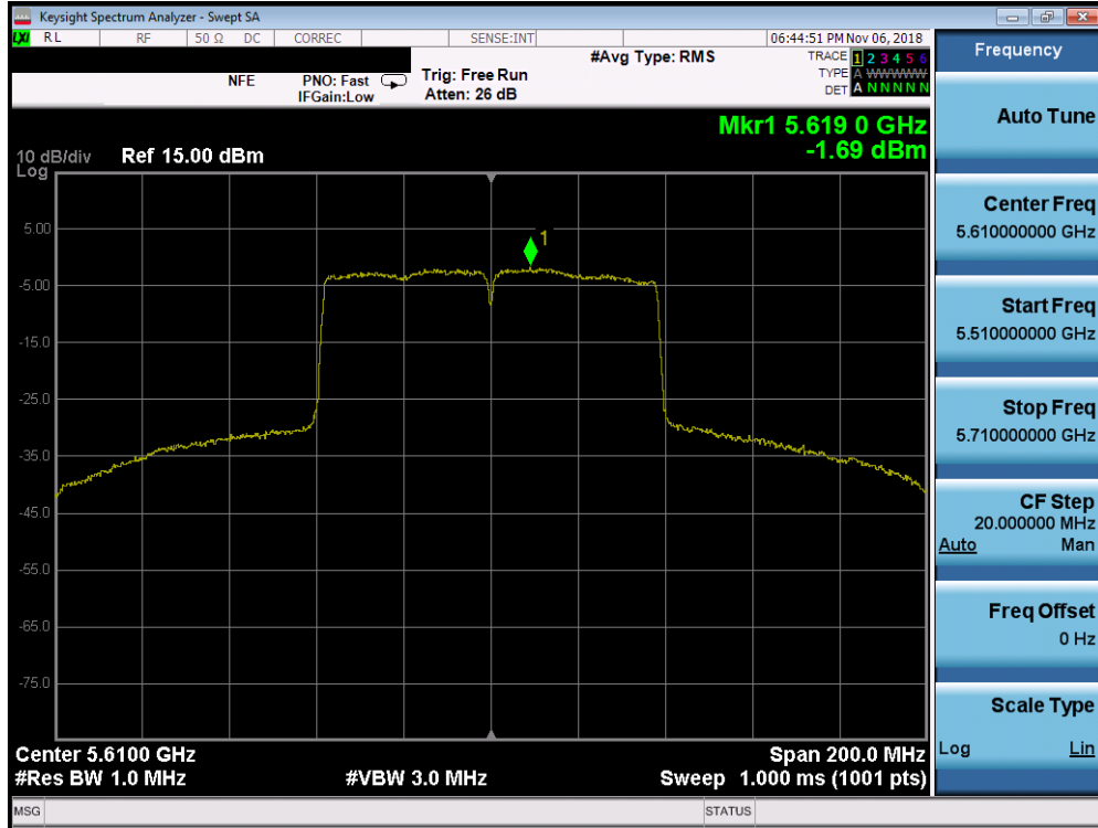
Plot 7-245. Power Spectral Density Plot SISO ANT2 (80MHz BW 802.11ac (UNII Band 2C) – Ch. 122)
