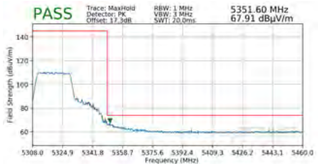
Plot 7-316. Radiated Upper Band Edge Plot SISO ANT2 (Peak – UNII Band 2A)
