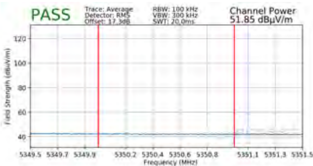
Plot 7-324. Radiated Upper Band Edge Plot SISO ANT2 (Average – UNII Band 2A)
