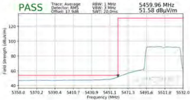
Plot 7-326. Radiated Lower Band Edge Plot SISO ANT2 (Average – UNII Band 2C)
