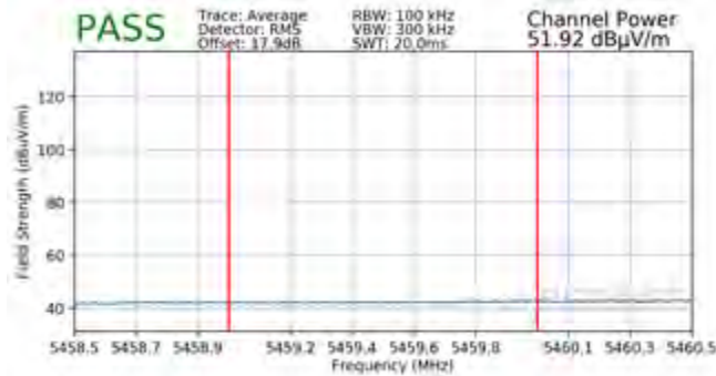
Plot 7-299. Radiated Lower Band Edge Plot SISO ANT1 (Average – UNII Band 2C)
