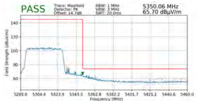
Plot 7-687. Radiated Upper Band Edge Plot SISO ANT1 (Peak – UNII Band 2A – 484 Tones)
