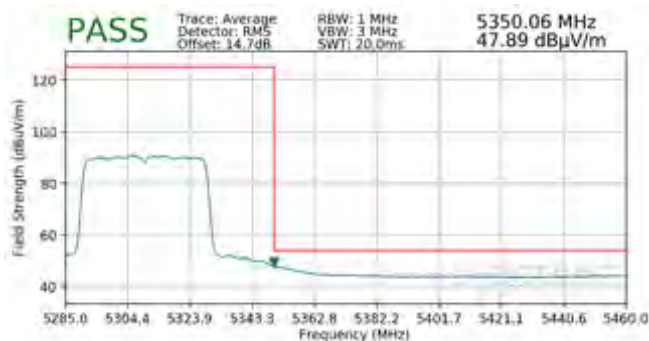
Plot 7-782. Radiated Upper Band Edge Plot MIMO (Average – UNII Band 2A – 484 Tones)
