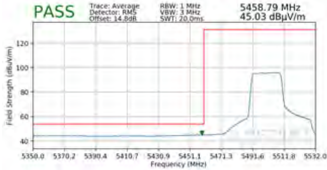
Plot 7-777. Radiated Lower Band Edge Plot MIMO (Average – UNII Band 2C – 242 Tones)
