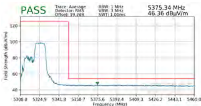
Plot 7-711. Radiated Upper Band Edge Plot SISO ANT2 (Average – UNII Band 2A – 106 Tones)
