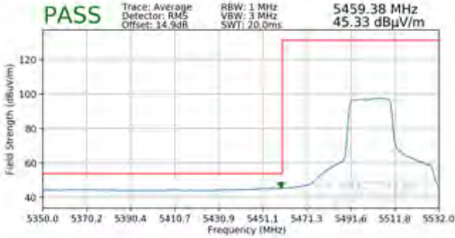
Plot 7-681. Radiated Lower Band Edge Plot SISO ANT1 (Average – UNII Band 2C – 242 Tones)
