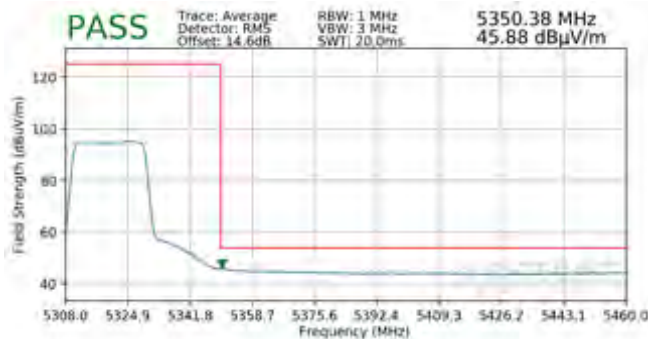
Plot 7-766. Radiated Upper Band Edge Plot MIMO (Average – UNII Band 2A – 242 Tones)
