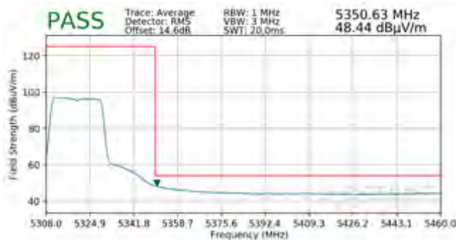
Plot 7-718. Radiated Upper Band Edge Plot SISO ANT2 (Average – UNII Band 2A – 242 Tones)
