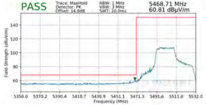
Plot 7-682. Radiated Lower Band Edge Plot SISO ANT1 (Peak – UNII Band 2C – 242 Tones)
