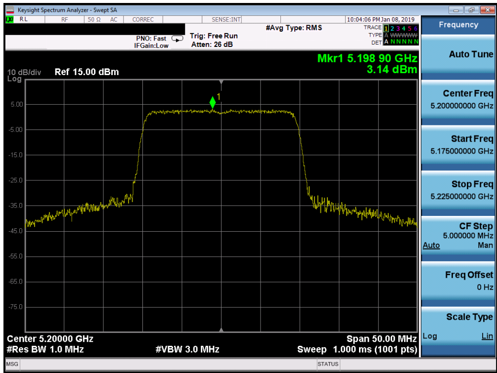
Plot 7-578. Power Spectral Density Plot MIMO ANT2 (20MHz BW 802.11ax – 242 Tones (UNII Band 1) – Ch. 40)
