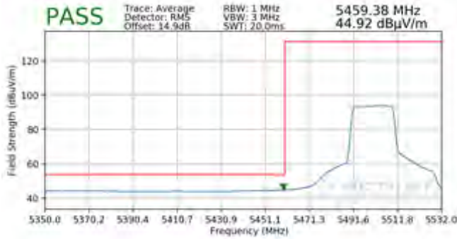
Plot 7-729. Radiated Lower Band Edge Plot SISO ANT2 (Average – UNII Band 2C – 242 Tones)
