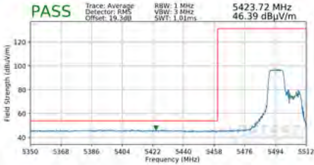
Plot 7-713. Radiated Lower Band Edge Plot SISO ANT2 (Average – UNII Band 2C – 106 Tones)
