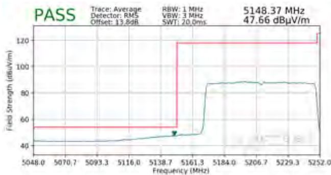
Plot 7-700. Radiated Lower Band Edge Plot SISO ANT1 (Average – UNII Band 1 – 996 Tones)
