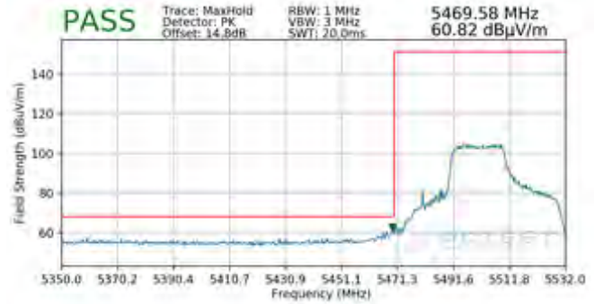
Plot 7-730. Radiated Lower Band Edge Plot SISO ANT2 (Peak – UNII Band 2C – 242 Tones)
