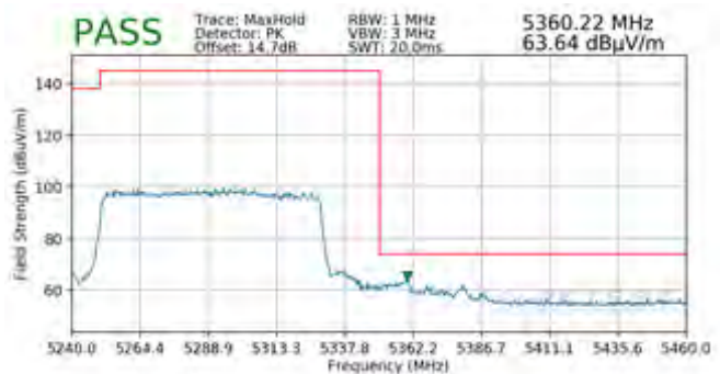
Plot 7-751. Radiated Upper Band Edge Plot SISO ANT2 (Peak – UNII Band 2A – 996 Tones)
