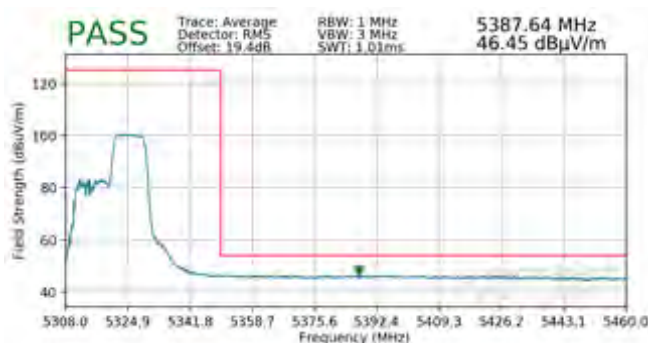
Plot 7-663. Radiated Upper Band Edge Plot SISO ANT1 (Average – UNII Band 2A – 106 Tones)
