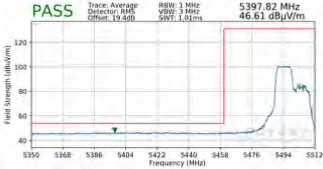
Plot 7-665. Radiated Lower Band Edge Plot SISO ANT1 (Average – UNII Band 2C – 106 Tones)
