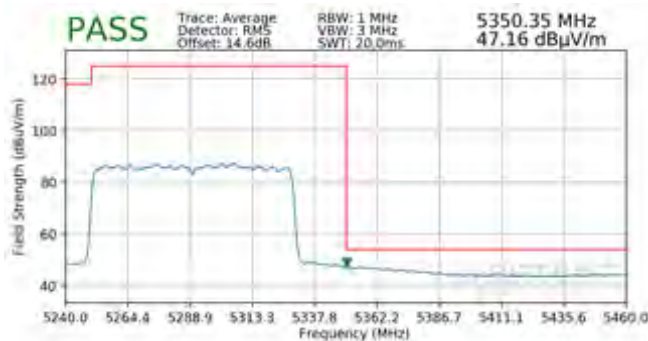
Plot 7-798. Radiated Upper Band Edge Plot MIMO (Average – UNII Band 2A – 996 Tones)
