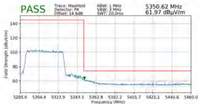
Plot 7-735. Radiated Upper Band Edge Plot SISO ANT2 (Peak – UNII Band 2A – 484 Tones)
