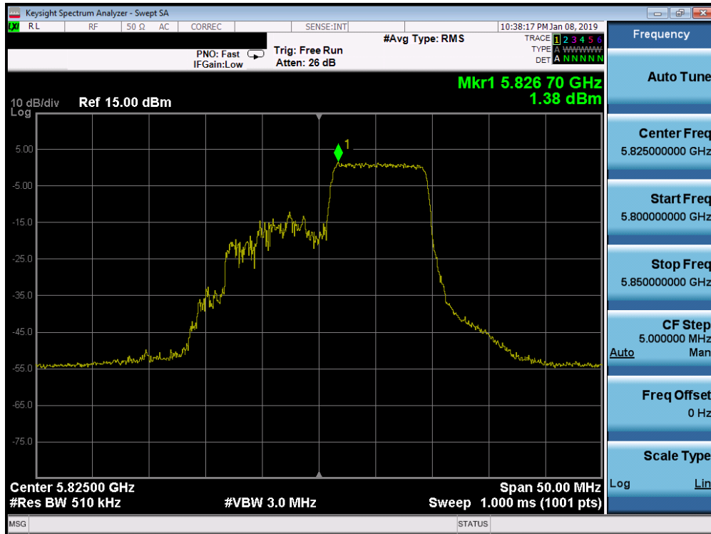
Plot 7-573. Power Spectral Density Plot MIMO ANT2 (20MHz BW 802.11ax – 106 Tones (UNII Band 3) – Ch. 165)
