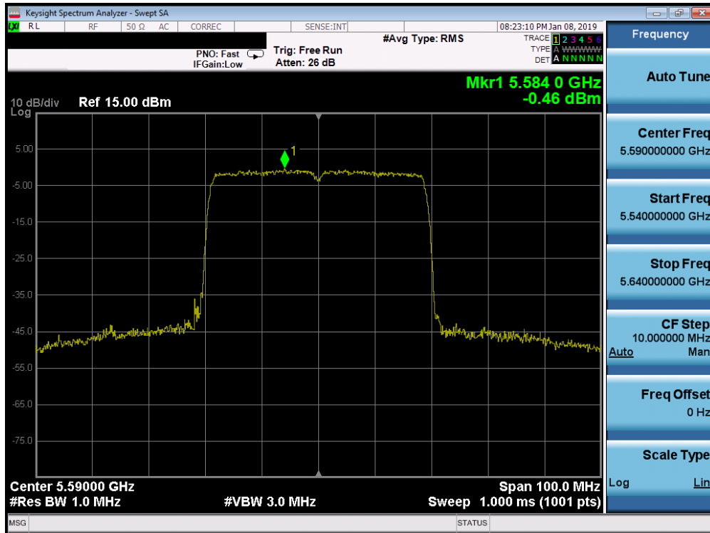
Plot 7-482. Power Spectral Density Plot MIMO ANT1 (40MHz BW 802.11ax – 484 Tones (UNII Band 2C) – Ch. 118)
