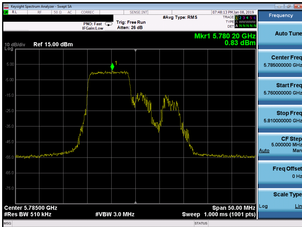
Plot 7-443. Power Spectral Density Plot MIMO ANT1 (20MHz BW 802.11ax – 106 Tones (UNII Band 3) – Ch. 157)
