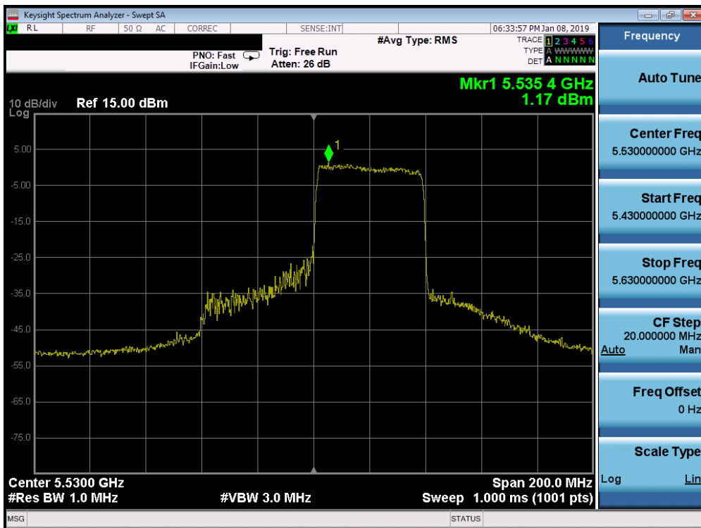
Plot 7-355. Power Spectral Density Plot SISO ANT2 (80MHz BW 802.11ax – 484 Tones (UNII Band 2C) – Ch. 106)
