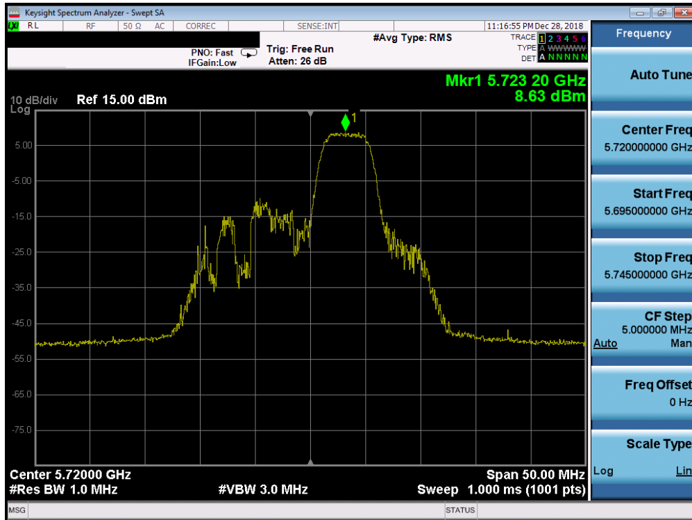
Plot 7-279. Power Spectral Density Plot SISO ANT2 (20MHz BW 802.11ax – 52 Tones (UNII Band 2C) – Ch. 144)
