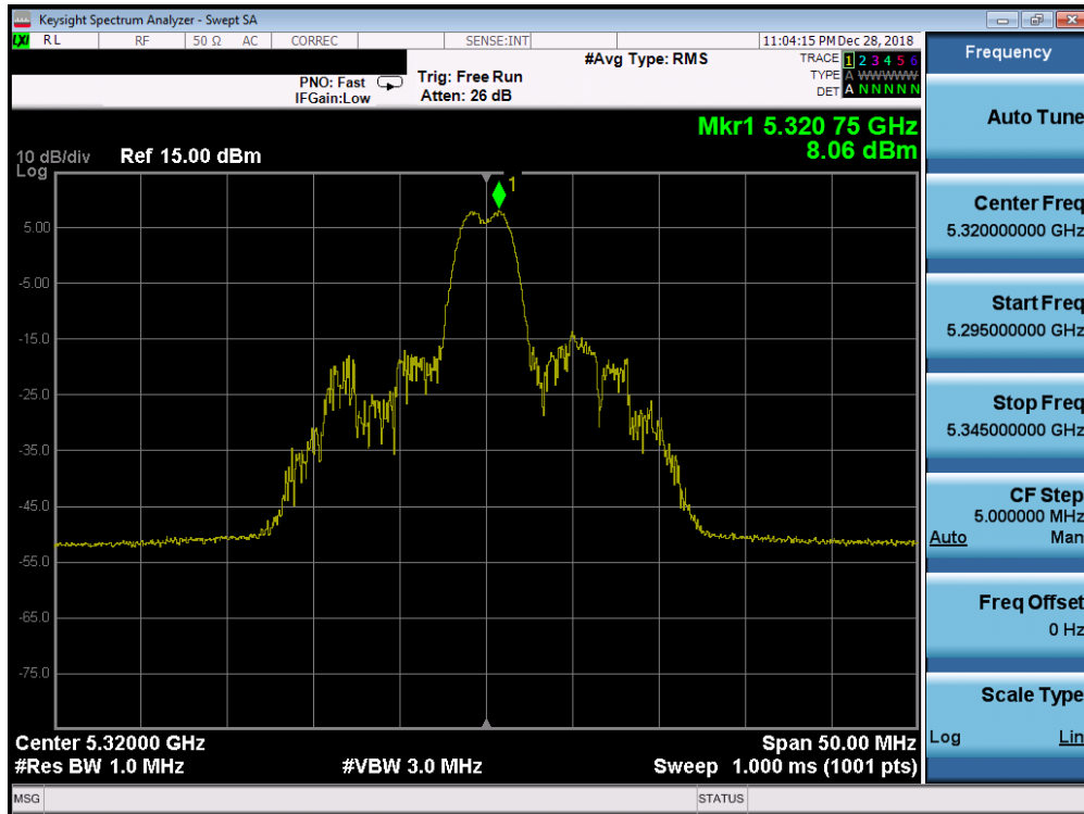
Plot 7-246. Power Spectral Density Plot SISO ANT2 (20MHz BW 802.11ax – 26 Tones (UNII Band 2A) – Ch. 64)
