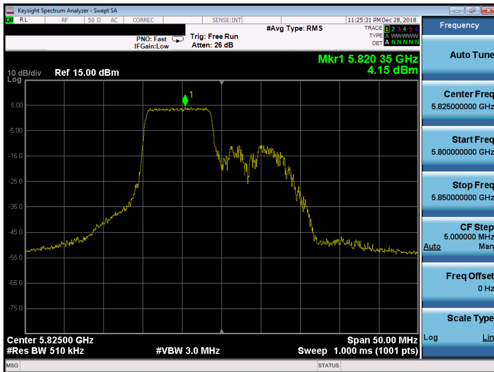
Plot 7-315. Power Spectral Density Plot SISO ANT2 (20MHz BW 802.11ax – 106 Tones (UNII Band 3) – Ch. 165)
