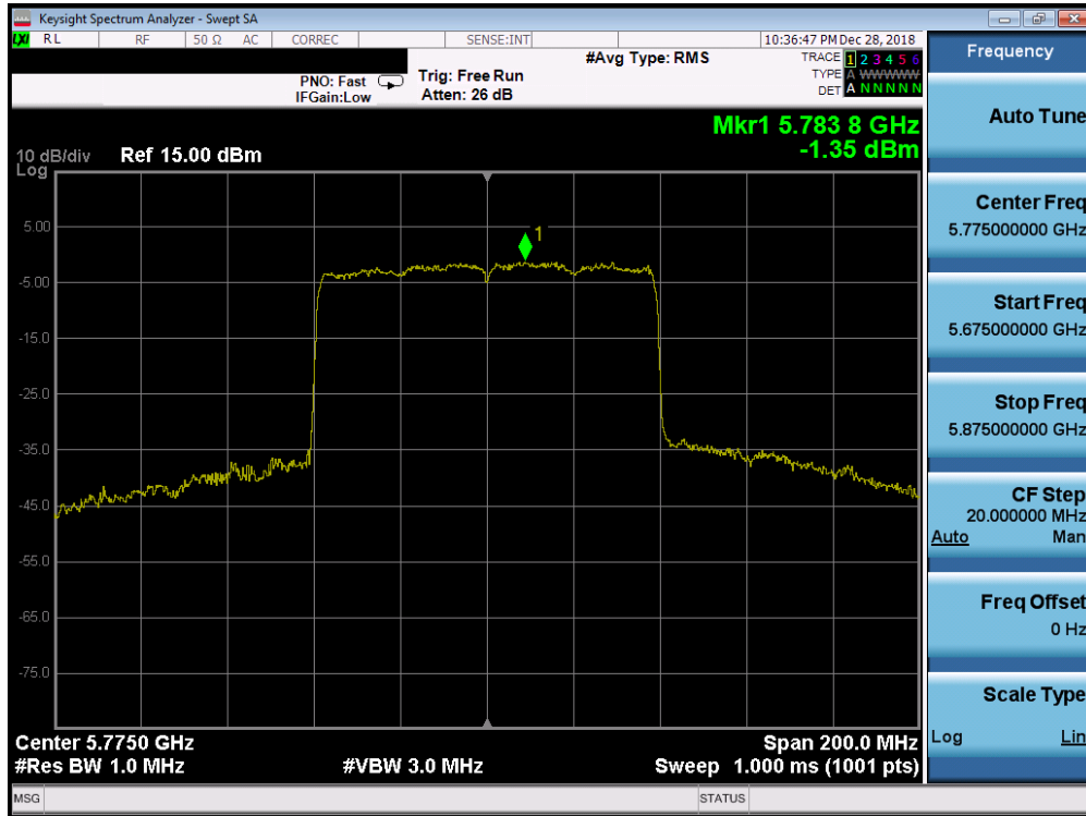
Plot 7-237. Power Spectral Density Plot SISO ANT1 (80MHz BW 802.11ax – 996 Tones (UNII Band 3) – Ch. 155)
