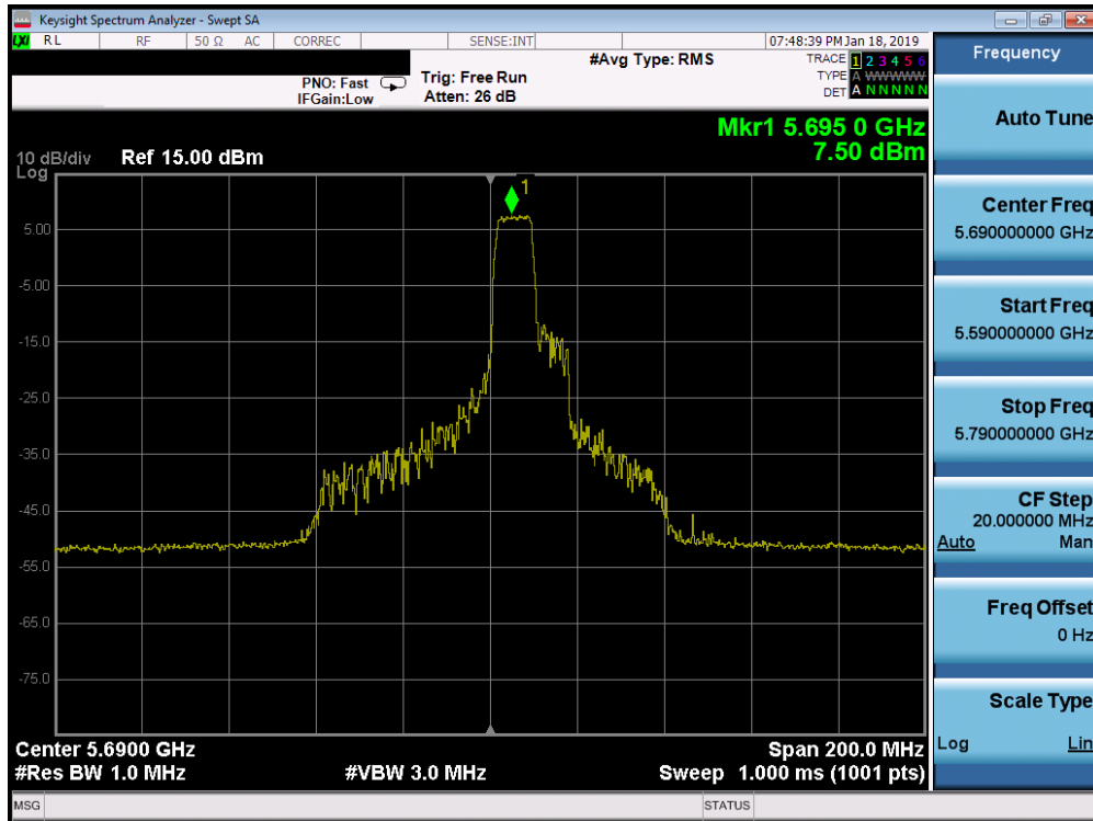
Plot 7-312. Power Spectral Density Plot SISO ANT2 (80MHz BW 802.11ax – 106 Tones (UNII Band 2C) – Ch. 138)
