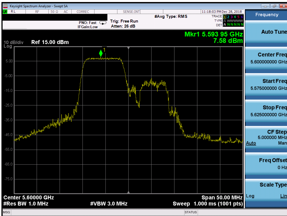
Plot 7-305. Power Spectral Density Plot SISO ANT2 (20MHz BW 802.11ax – 106 Tones (UNII Band 2C) – Ch. 120)
