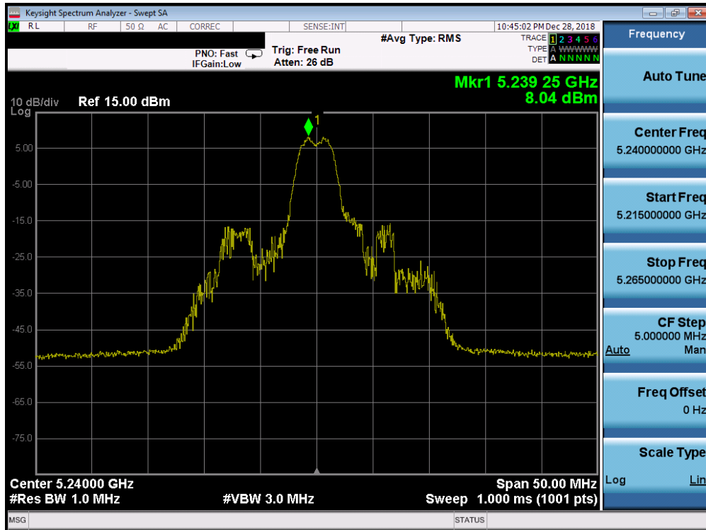
Plot 7-240. Power Spectral Density Plot SISO ANT2 (20MHz BW 802.11ax – 26 Tones (UNII Band 1) – Ch. 48)
