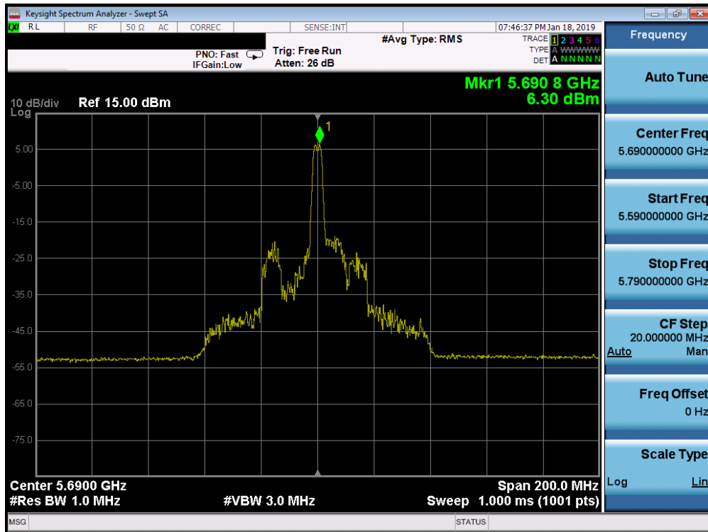
Plot 7-258. Power Spectral Density Plot SISO ANT2 (80MHz BW 802.11ax – 26 Tones (UNII Band 2C) – Ch. 138)
