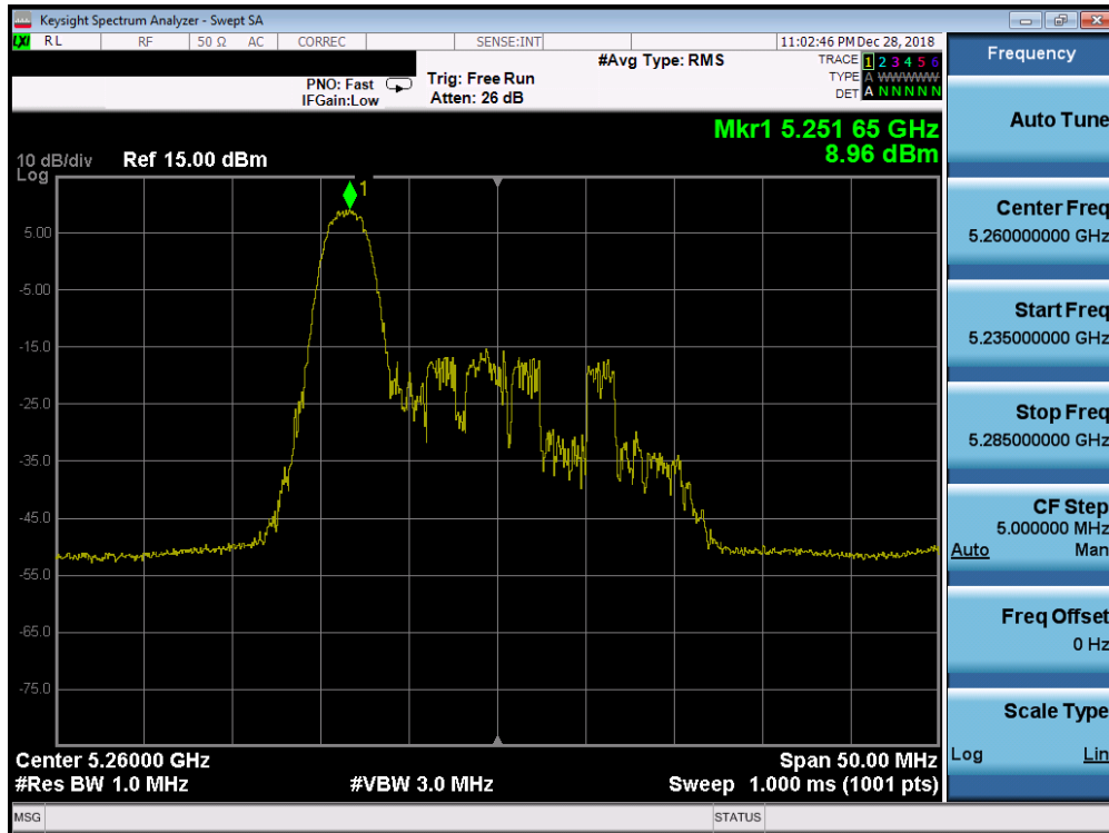
Plot 7-244. Power Spectral Density Plot SISO ANT2 (20MHz BW 802.11ax – 26 Tones (UNII Band 2A) – Ch. 52)
