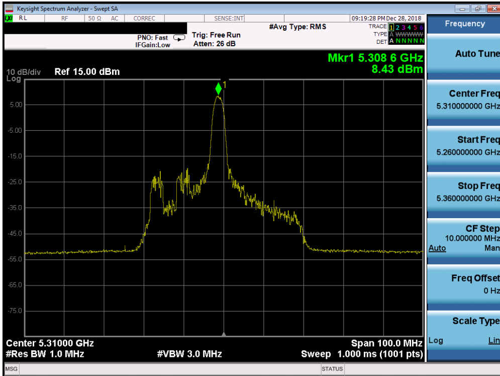
Plot 7-119. Power Spectral Density Plot SISO ANT1 (40MHz BW 802.11ax – 26 Tones (UNII Band 2A) – Ch. 62)
