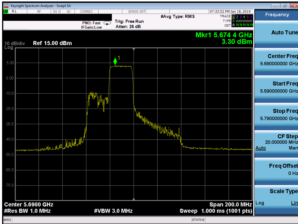
Plot 7-210. Power Spectral Density Plot SISO ANT1 (80MHz BW 802.11ax – 242 Tones (UNII Band 2C) – Ch. 138)
