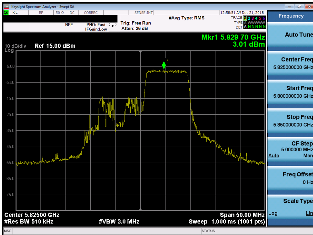
Plot 7-186. Power Spectral Density Plot SISO ANT1 (20MHz BW 802.11ax – 106 Tones (UNII Band 3) – Ch. 165)
