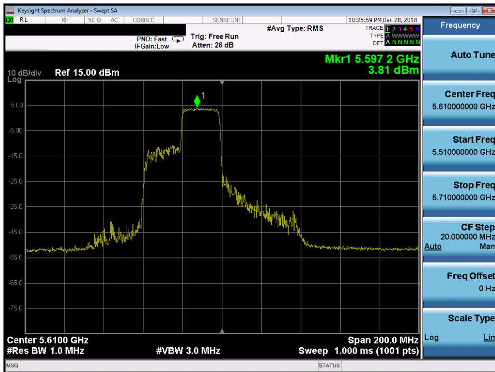
Plot 7-209. Power Spectral Density Plot SISO ANT1 (80MHz BW 802.11ax – 242 Tones (UNII Band 2C) – Ch. 122)
