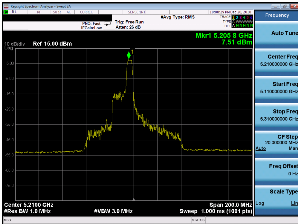
Plot 7-141. Power Spectral Density Plot SISO ANT1 (80MHz BW 802.11ax – 52 Tones (UNII Band 1) – Ch. 42)
