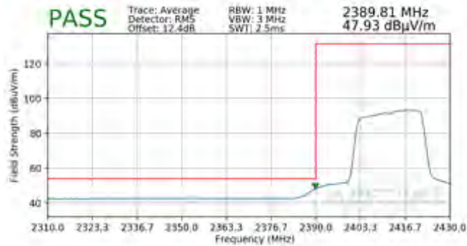
Plot 7-177. Radiated Restricted Band Edge Measurement SISO ANT1 with WCP (Average – 242 Tones)
