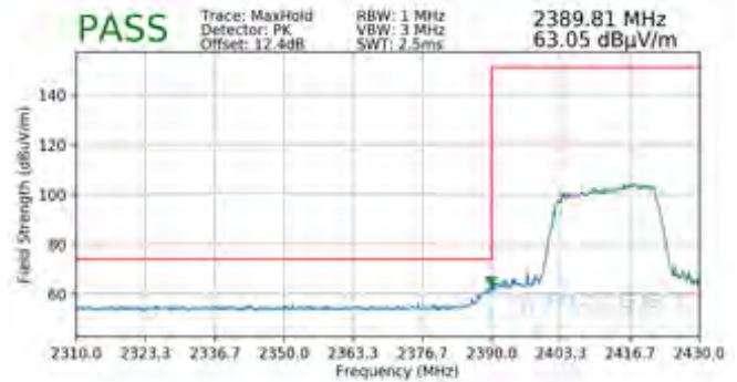
Plot 7-178. Radiated Restricted Band Edge Measurement SISO ANT1 with WCP (Peak – 242 Tones)
