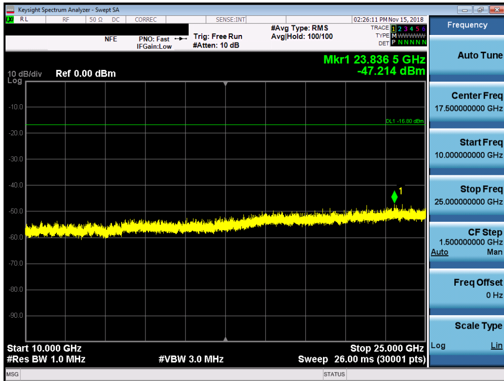
Plot 7-106. Conducted Spurious Plot SISO ANT2 (802.11ax OFDMA– 26 Tones – Ch. 1)
