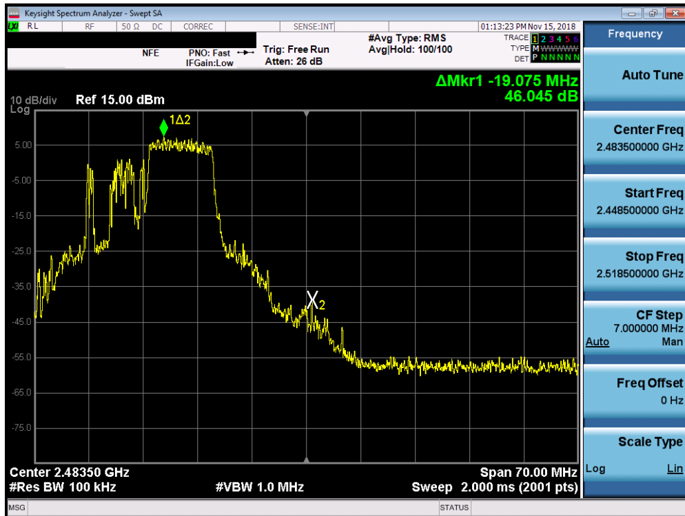
Plot 7-74. Band Edge Plot SISO ANT2 (802.11ax OFDMA – 106 Tones – Ch. 11)
