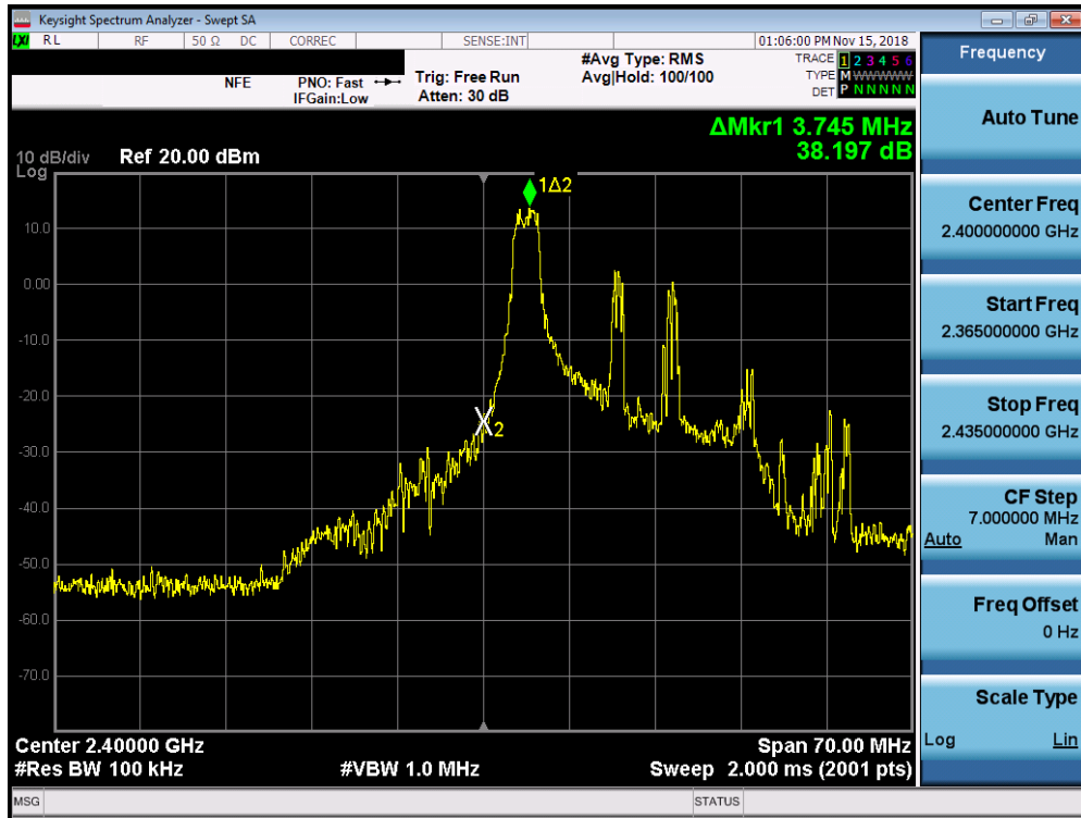
Plot 7-65. Band Edge Plot SISO ANT2 (802.11ax OFDMA – 26 Tones – Ch. 1)
