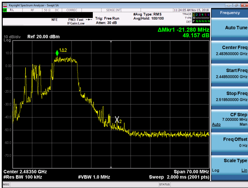
Plot 7-58. Band Edge Plot SISO ANT1 (802.11ax OFDMA – 106 Tones – Ch. 11)
