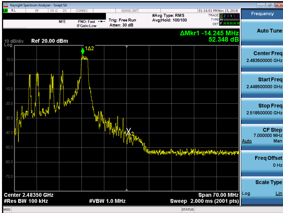
Plot 7-66. Band Edge Plot SISO ANT2 (802.11ax OFDMA – 26 Tones – Ch. 11)
