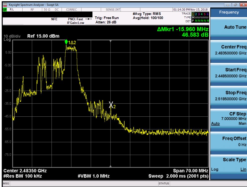
Plot 7-70. Band Edge Plot SISO ANT2 (802.11ax OFDMA – 52 Tones – Ch. 11)
