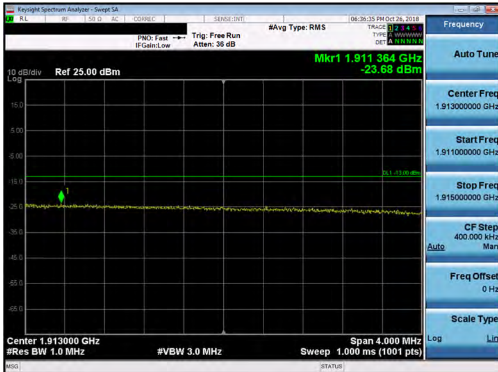
Plot 7-207. Upper Extended Band Edge Plot (Band 2 - 15.0MHz QPSK - Full RB Configuration)
