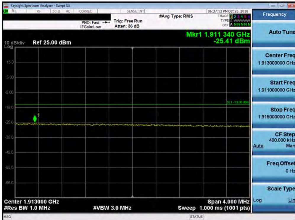
Plot 7-213. Upper Extended Band Edge Plot (Band 2 - 20.0MHz QPSK - Full RB Configuration)
