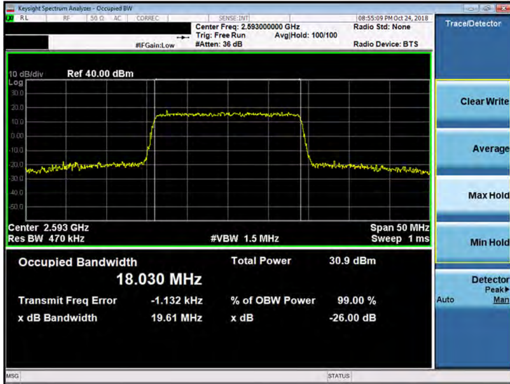
Plot 7-80. Occupied Bandwidth Plot (Band 41 PC3 - 20.0MHz 16-QAM - Full RB Configuration)
