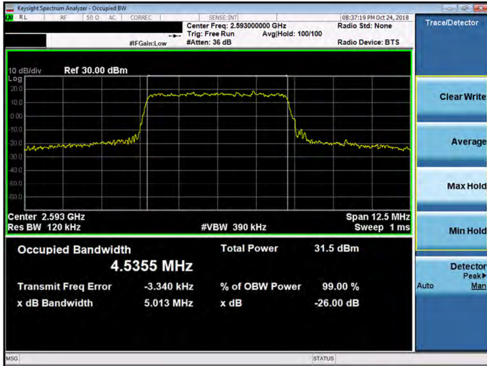
Plot 7-70. Occupied Bandwidth Plot (Band 41 PC3– 5.0MHz QPSK - Full RB Configuration)
