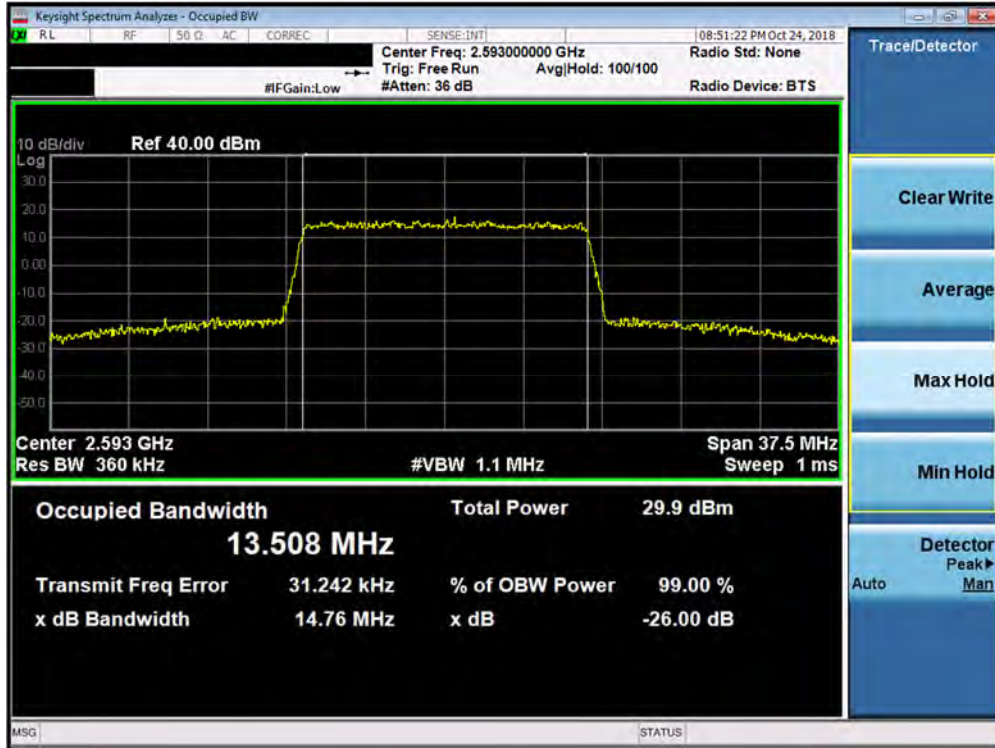
Plot 7-78. Occupied Bandwidth Plot (Band 41 PC3 - 15.0MHz 64-QAM - Full RB Configuration)
