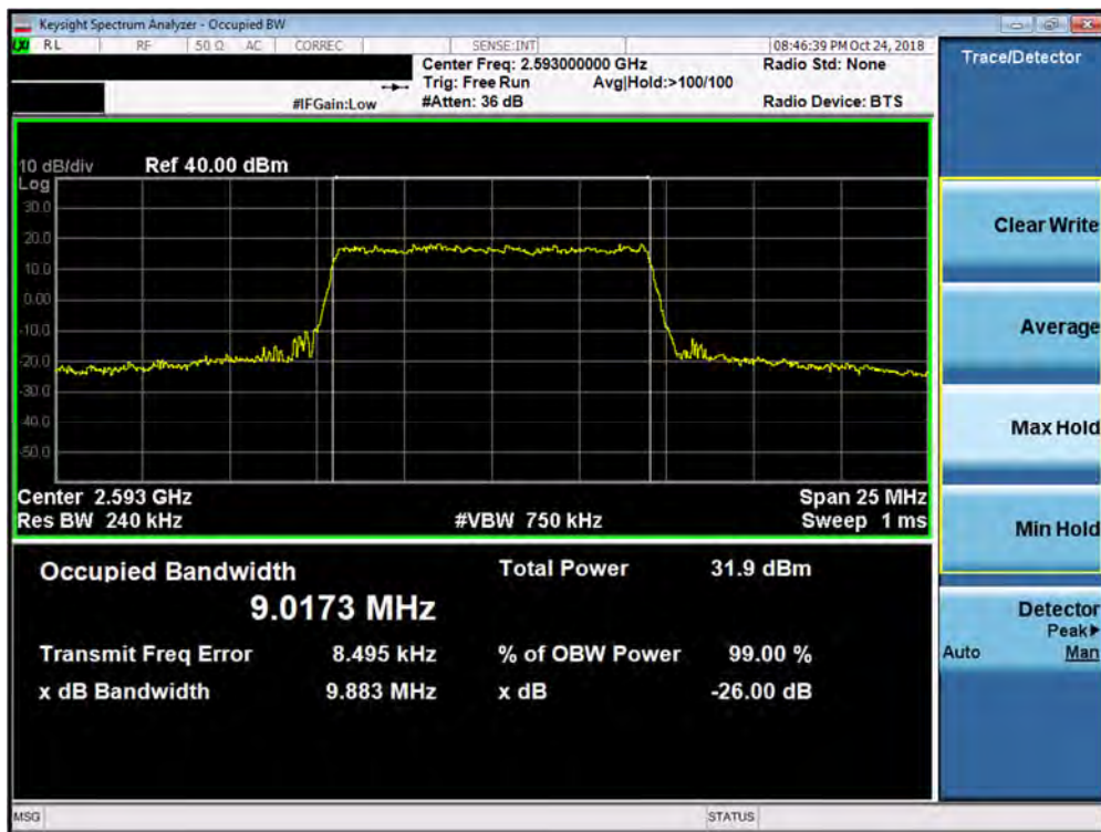
Plot 7-73. Occupied Bandwidth Plot (Band 41 PC3 - 10.0MHz QPSK - Full RB Configuration)
