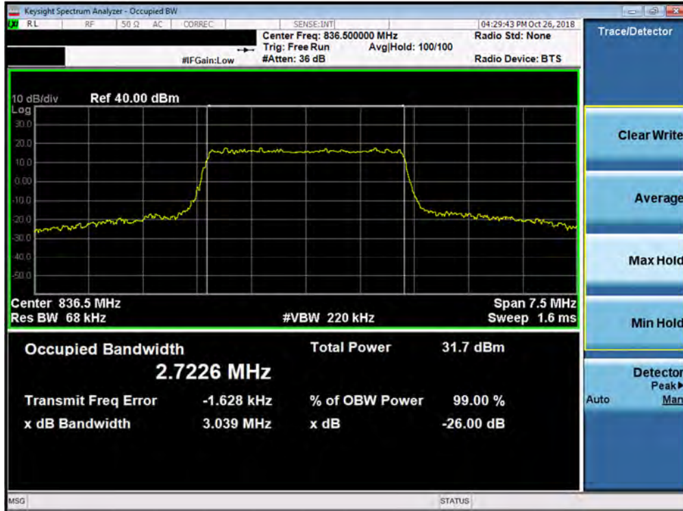
Plot 7-23. Occupied Bandwidth Plot (Band 26/5 - 3.0MHz 16-QAM - Full RB Configuration)
