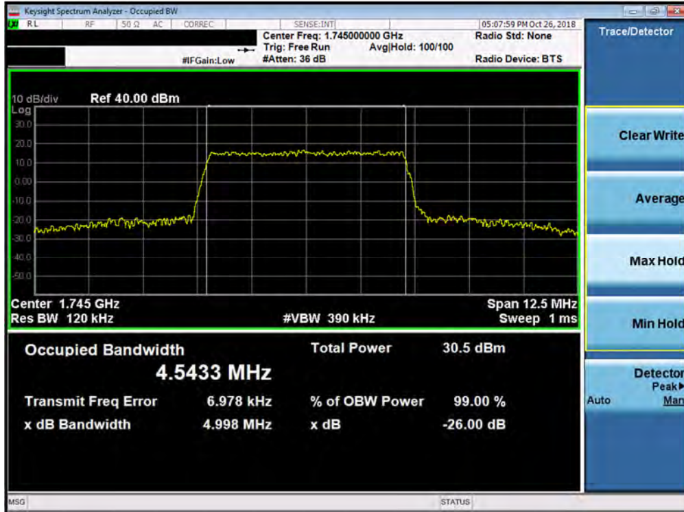
Plot 7-42. Occupied Bandwidth Plot (Band 4 - 5.0MHz 64-QAM - Full RB Configuration)
