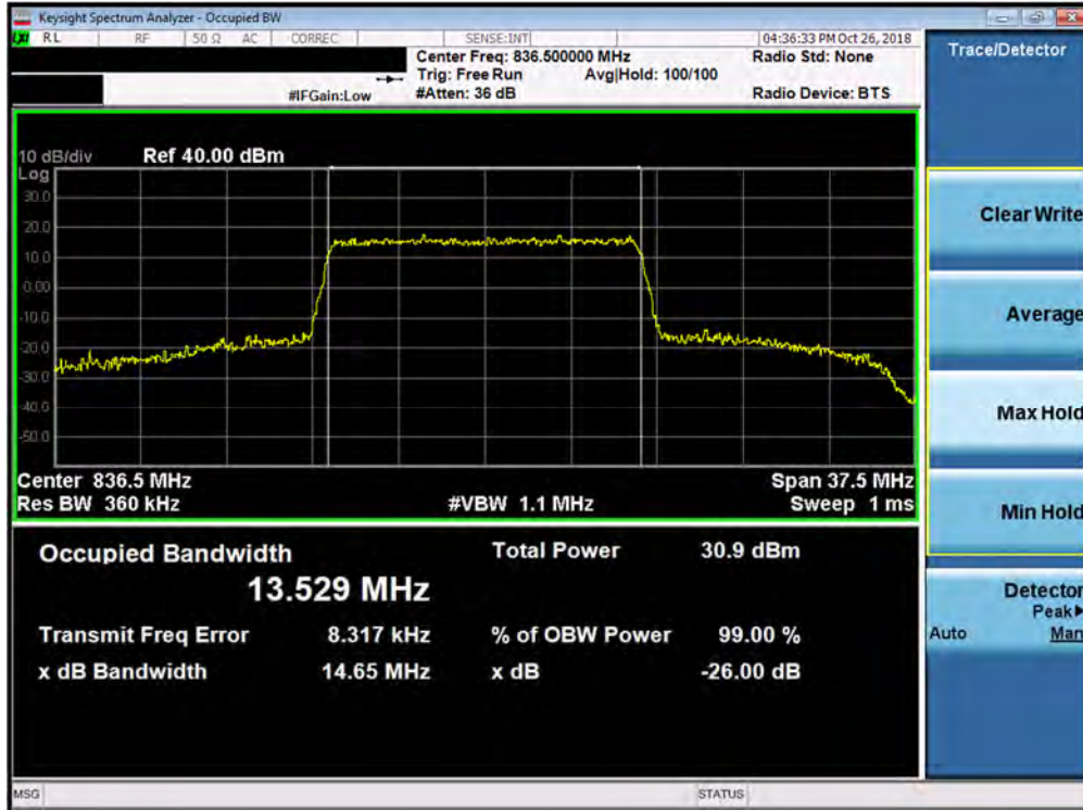
Plot 7-33. Occupied Bandwidth Plot (Band 26 - 15.0MHz 64-QAM - Full RB Configuration)
