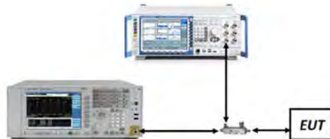
Figure 7-2. Test Instrument & Measurement Setup
