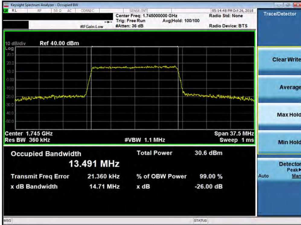
Plot 7-48. Occupied Bandwidth Plot (Band 4 - 15.0MHz 64-QAM - Full RB Configuration)
