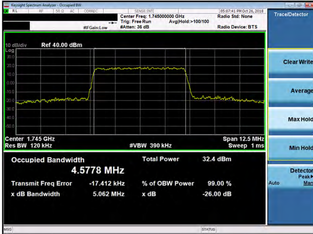
Plot 7-40. Occupied Bandwidth Plot (Band 4 - 5.0MHz QPSK - Full RB Configuration)
