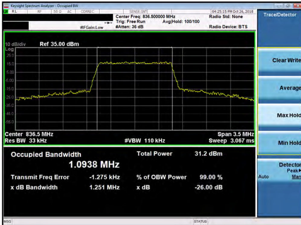
Plot 7-20. Occupied Bandwidth Plot (Band 26/5 - 1.4MHz 16-QAM - Full RB Configuration)
