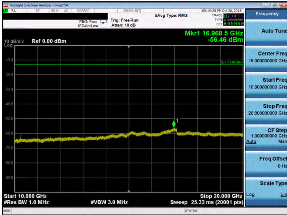
Plot 7-105. Conducted Spurious Plot (Band 4 - 15.0MHz QPSK - RB Size 1, RB Offset 0 - Low Channel)
