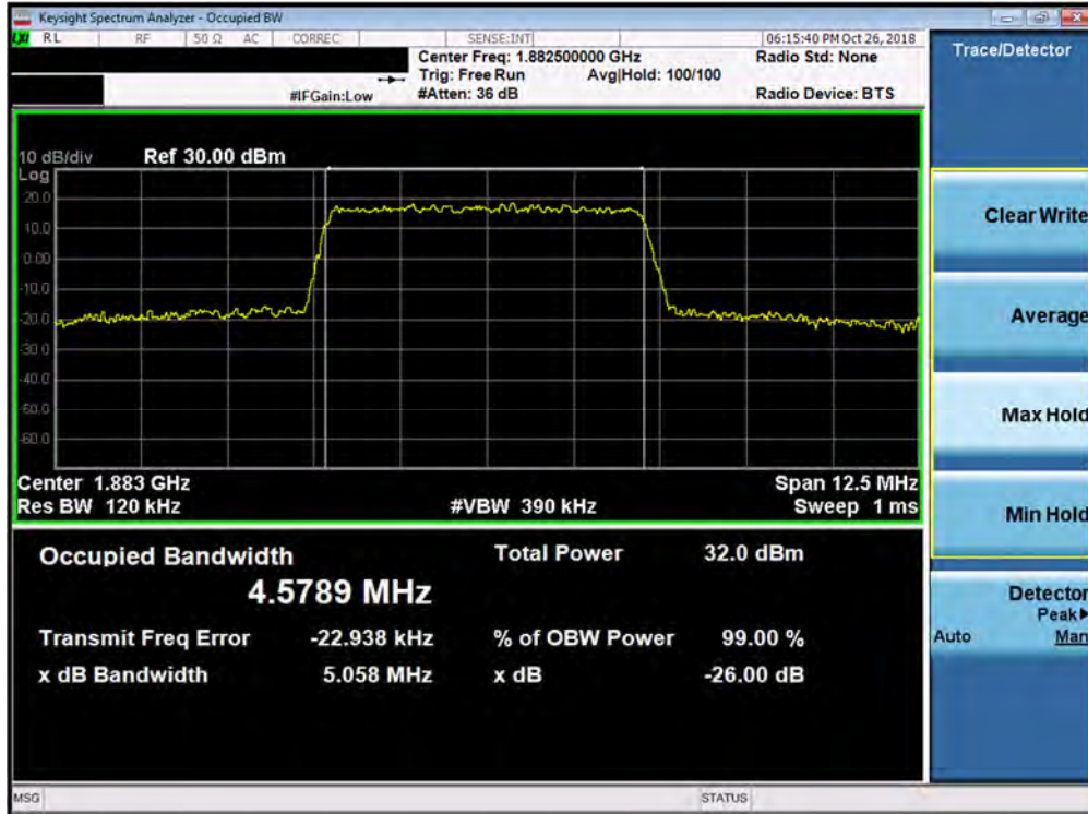
Plot 7-58. Occupied Bandwidth Plot (Band 25/2 - 5.0MHz QPSK - Full RB Configuration)
