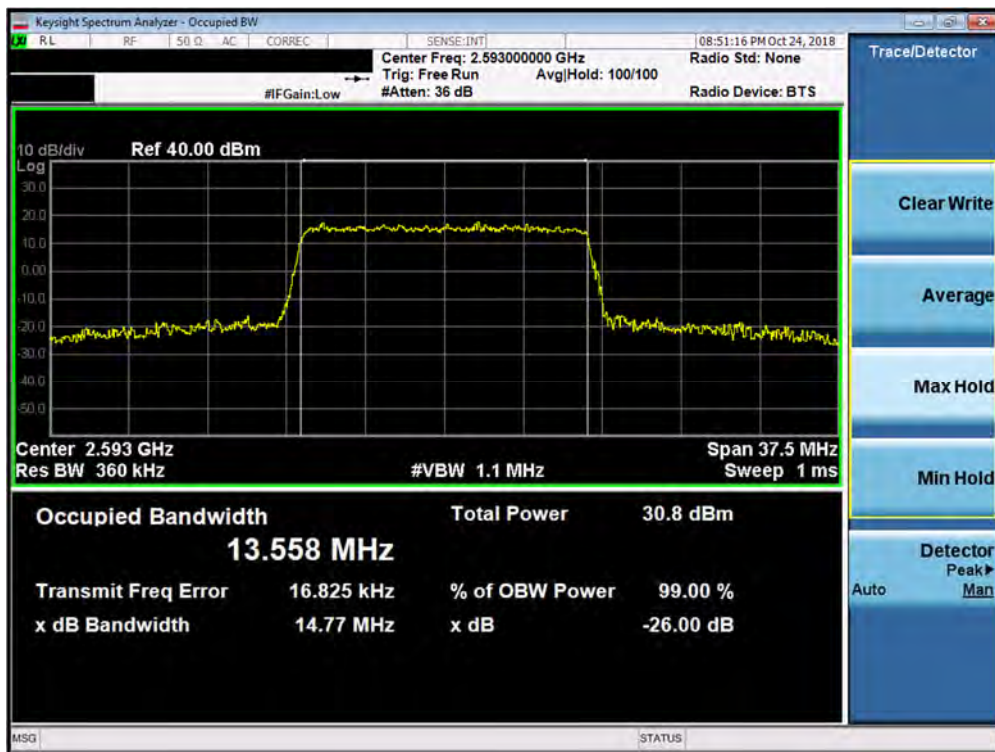
Plot 7-77. Occupied Bandwidth Plot (Band 41 PC3 - 15.0MHz 16-QAM - Full RB Configuration)
