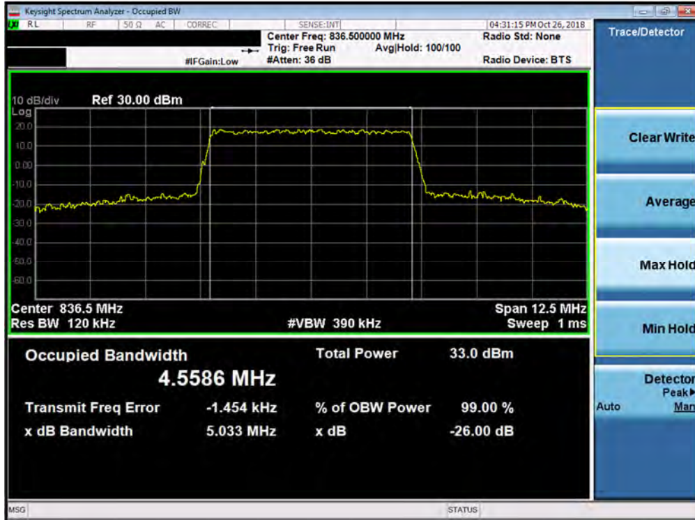
Plot 7-25. Occupied Bandwidth Plot (Band 26/5 - 5.0MHz QPSK - Full RB Configuration)
