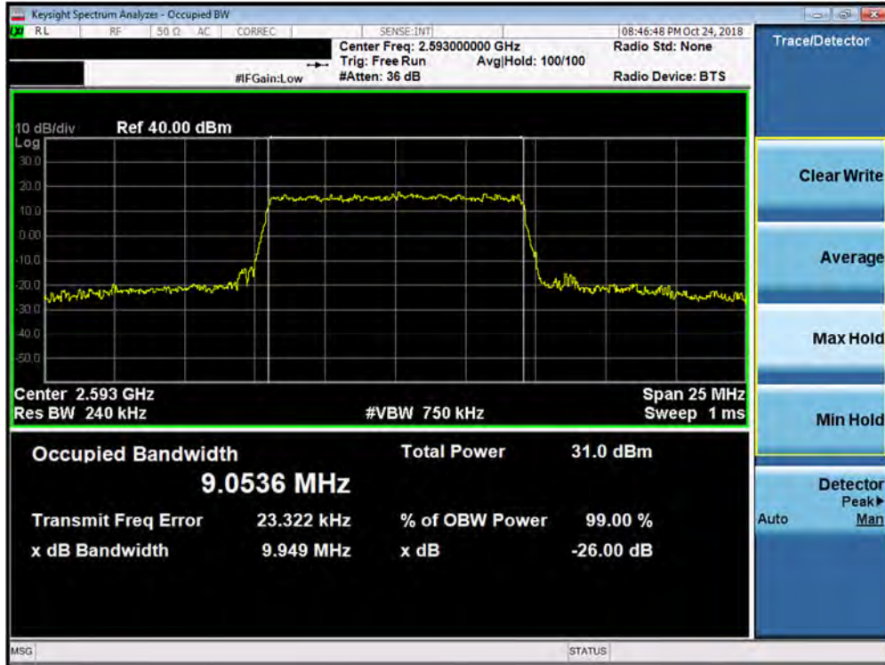
Plot 7-74. Occupied Bandwidth Plot (Band 41 PC3 - 10.0MHz 16-QAM - Full RB Configuration)
