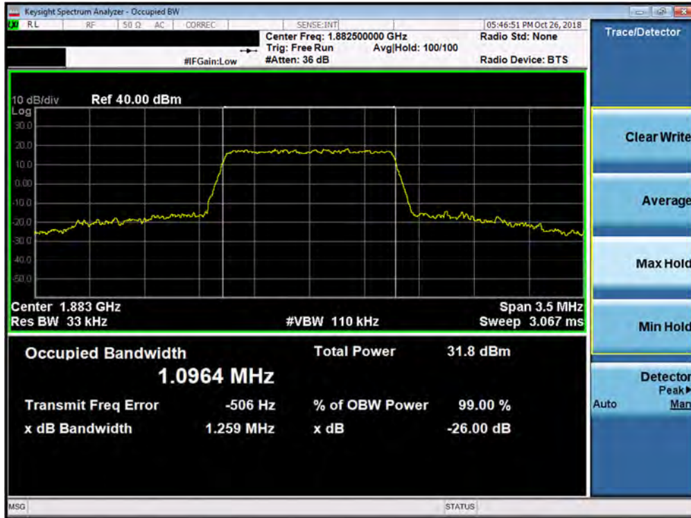
Plot 7-52. Occupied Bandwidth Plot (Band 25/2 - 1.4MHz QPSK - Full RB Configuration)
