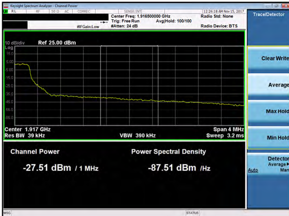
Plot 7-306. Upper Extended Band Edge Plot (Band 25 - 5.0MHz QPSK - Full RB Configuration)
