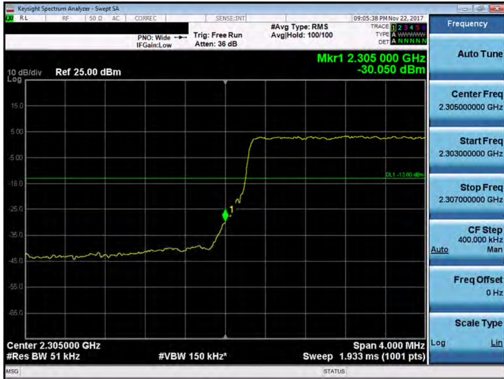
Plot 7-325. Lower Band Edge Plot (Band 30 - 5.0MHz QPSK - Full RB Configuration – Antenna A)
