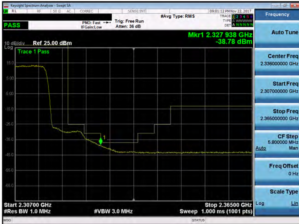
Plot 7-332. Upper Extended Band Edge Plot (Band 30 - 10.0MHz QPSK - Full RB Configuration–Antenna A)
