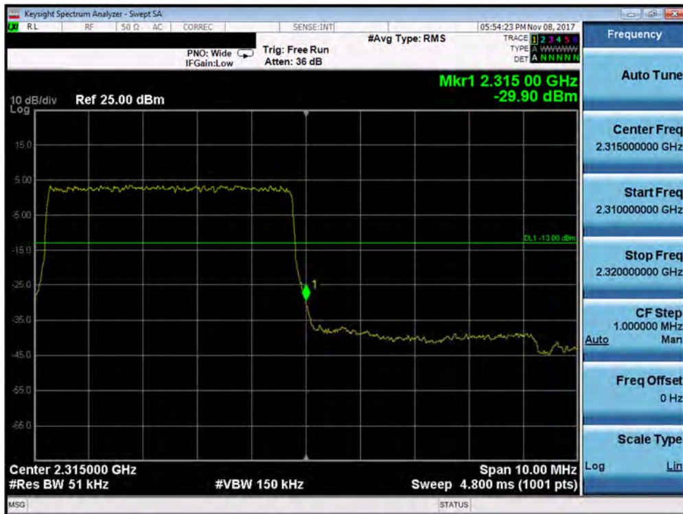
Plot 7-335. Upper Band Edge Plot (Band 30 - 5.0MHz QPSK - Full RB Configuration – Antenna B)
