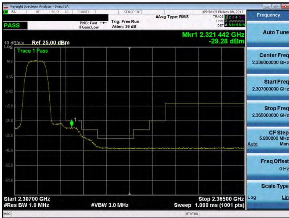
Plot 7-336. Upper Extended Band Edge Plot (Band 30 - 5.0MHz QPSK - Full RB Configuration – Antenna B)
