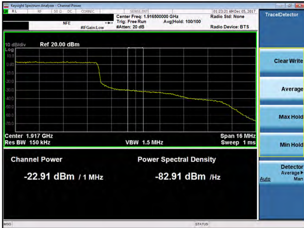
Plot 7-324. Upper Extended Band Edge Plot (Band 25 - 20.0MHz QPSK - Full RB Configuration)
