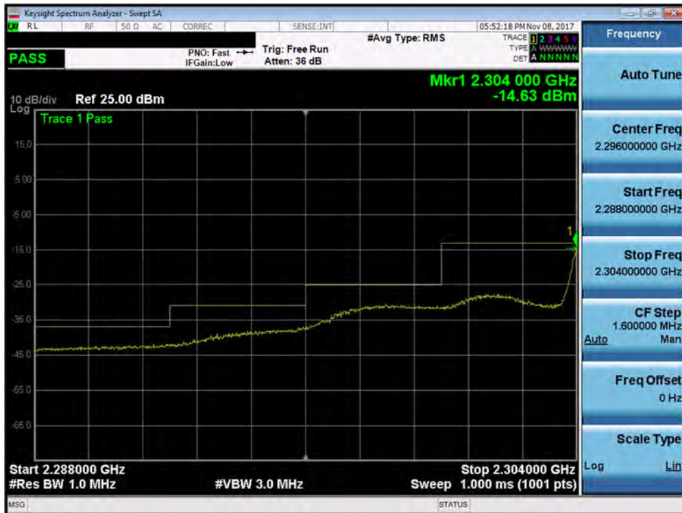
Plot 7-334. Lower Extended Band Edge Plot (Band 30 - 5.0MHz QPSK - Full RB Configuration – Antenna B)
