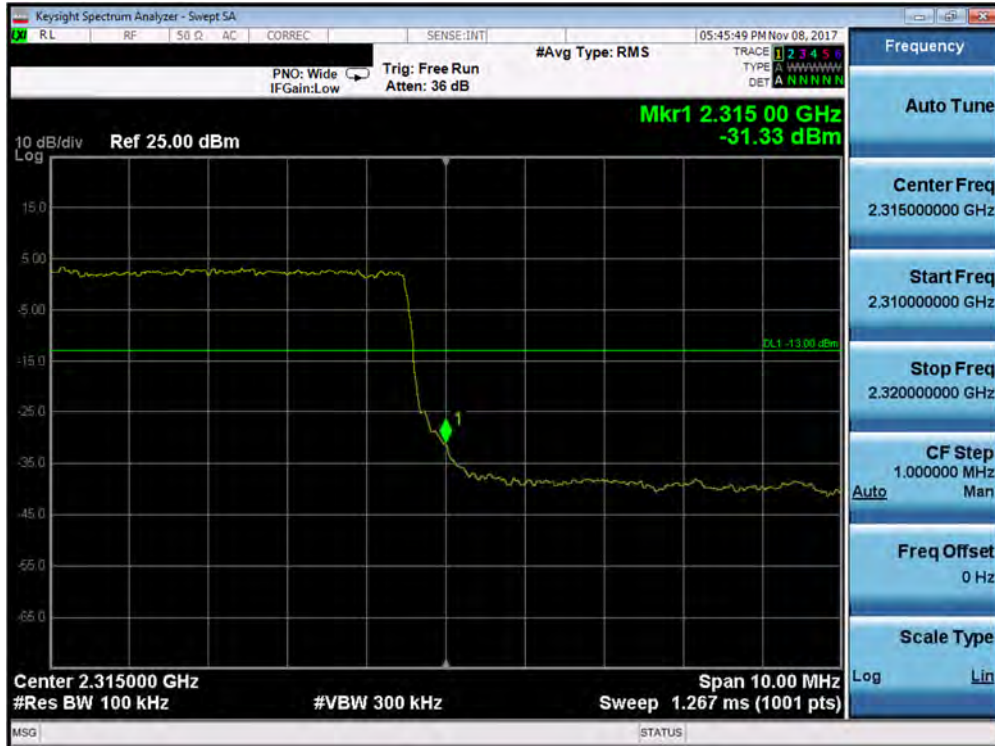
Plot 7-339. Upper Band Edge Plot (Band 30 - 10.0MHz QPSK - Full RB Configuration – Antenna B)
