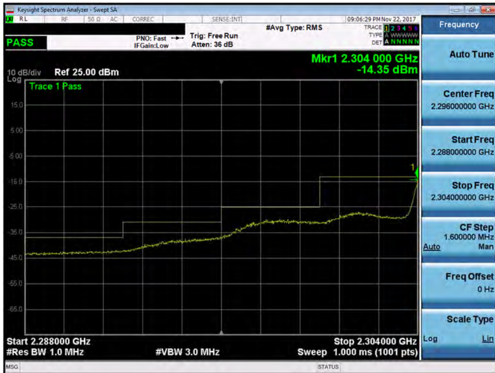
Plot 7-326. Lower Extended Band Edge Plot (Band 30 - 5.0MHz QPSK - Full RB Configuration – Antenna A)
