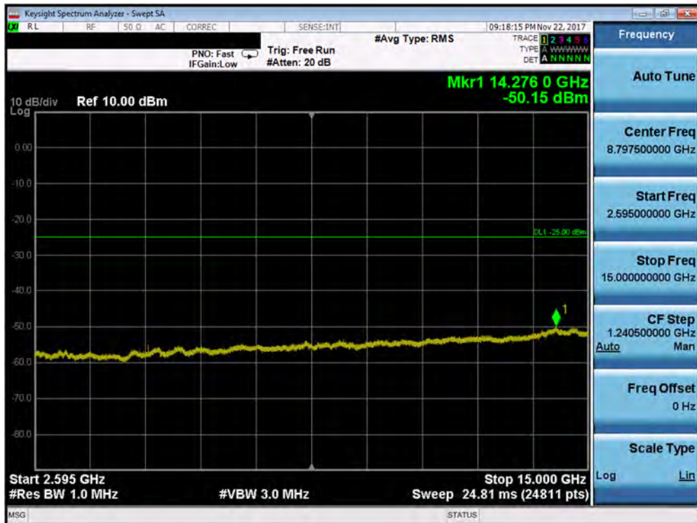
Plot 7-197. Conducted Spurious Plot (Band 7 - 5.0MHz QPSK - RB Size 1, RB Offset 0 - High Channel – Antenna A)
