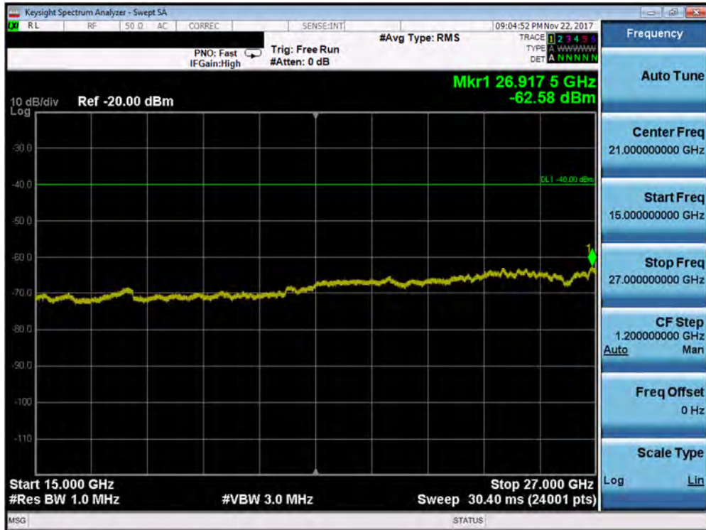
Plot 7-183. Conducted Spurious Plot (Band 30 - 5.0MHz QPSK - RB Size 1, RB Offset 0 - High Channel – Antenna A)
