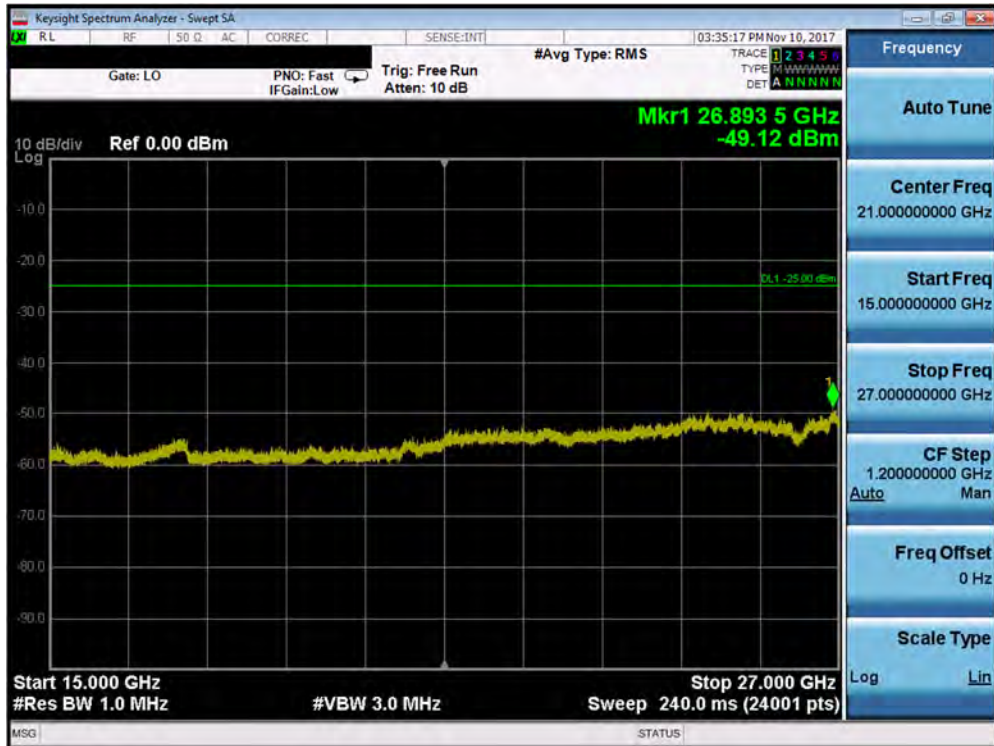
Plot 7-213. Conducted Spurious Plot (Band 41 - 20.0MHz QPSK - RB Size 1, RB Offset 0 - Mid Channel)
