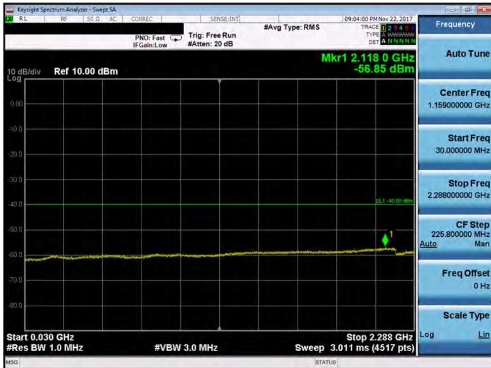
Plot 7-181. Conducted Spurious Plot (Band 30 - 5.0MHz QPSK - RB Size 1, RB Offset 0 - High Channel – Antenna A)
