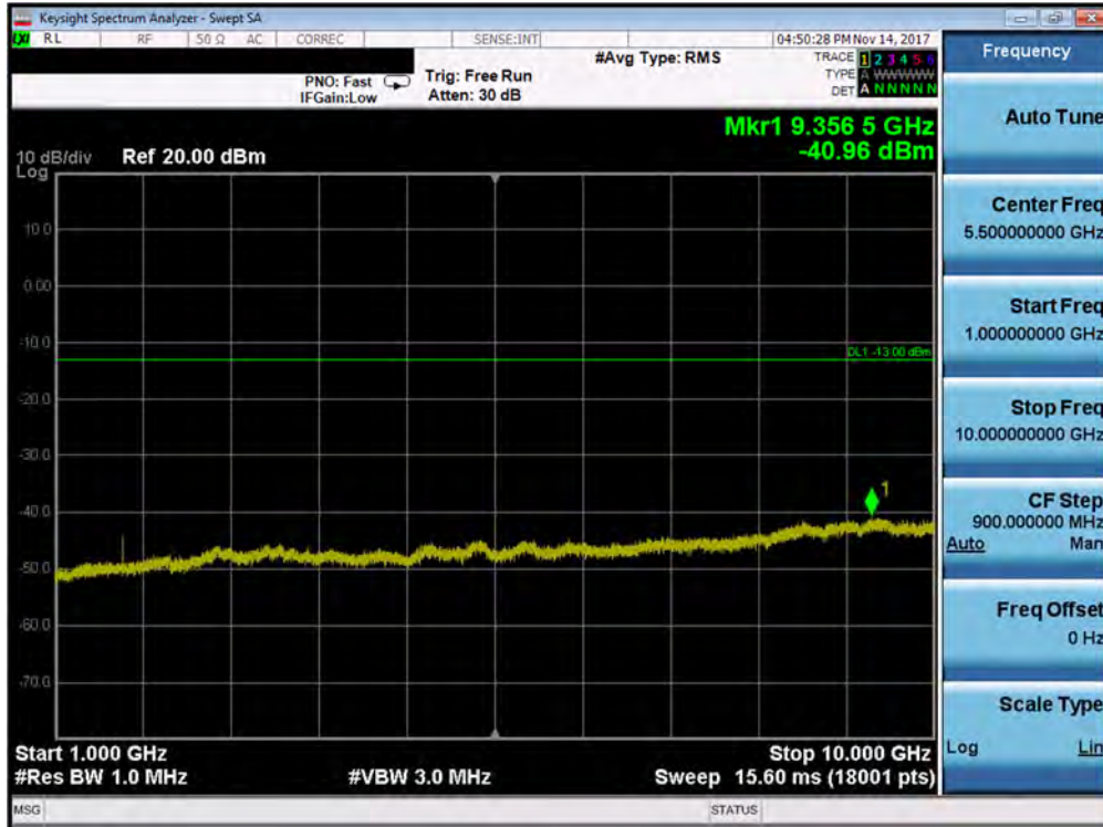
Plot 7-159. Conducted Spurious Plot (Band 26/5 - 5.0MHz QPSK - RB Size 1, RB Offset 0 - High Channel)
