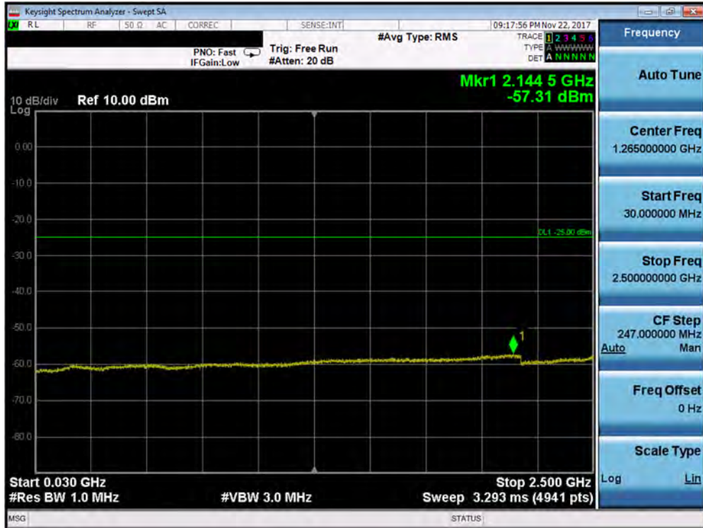
Plot 7-196. Conducted Spurious Plot (Band 7 - 5.0MHz QPSK - RB Size 1, RB Offset 0 - High Channel – Antenna A)
