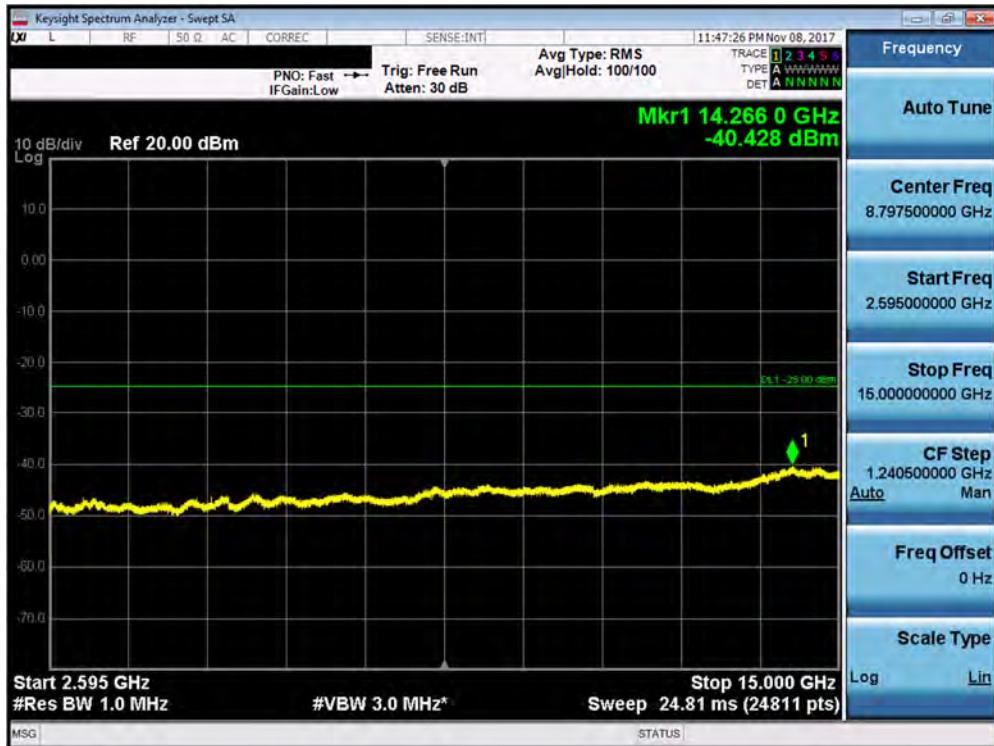
Plot 7-206. Conducted Spurious Plot (Band 7 - 5.0MHz QPSK - RB Size 1, RB Offset 0 - High Channel – Antenna B)
