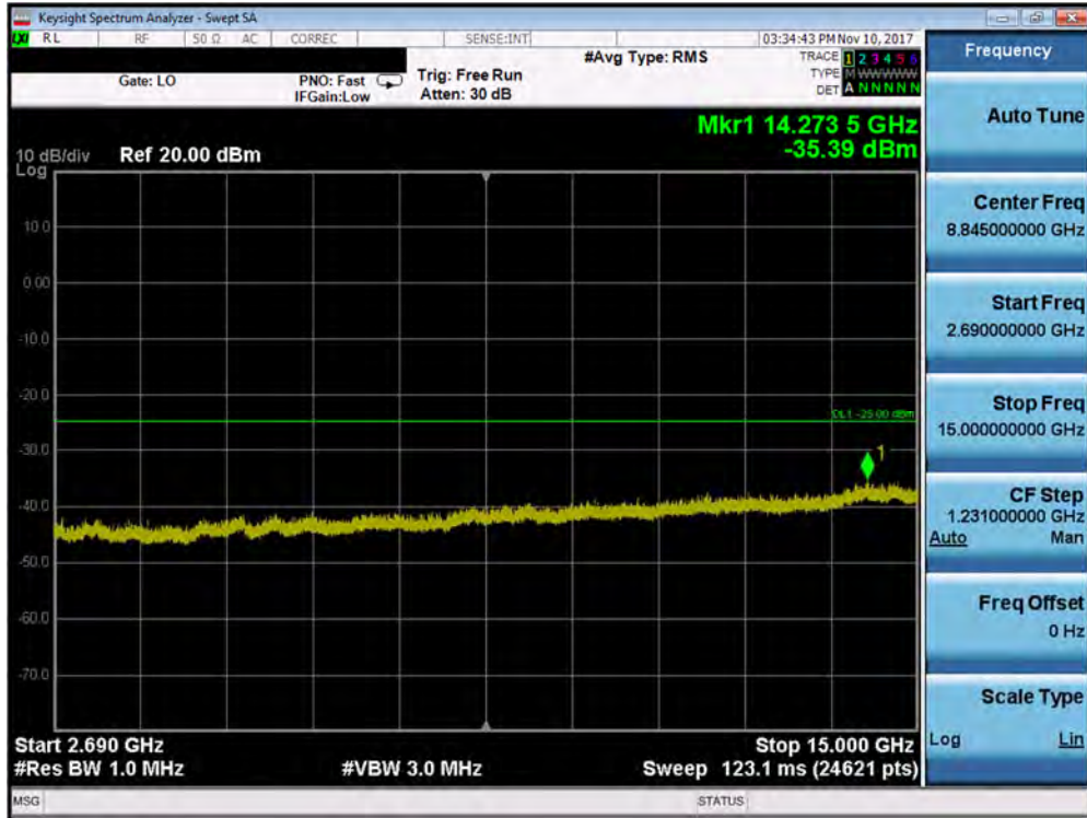
Plot 7-212. Conducted Spurious Plot (Band 41 - 20.0MHz QPSK - RB Size 1, RB Offset 0 - Mid Channel)
