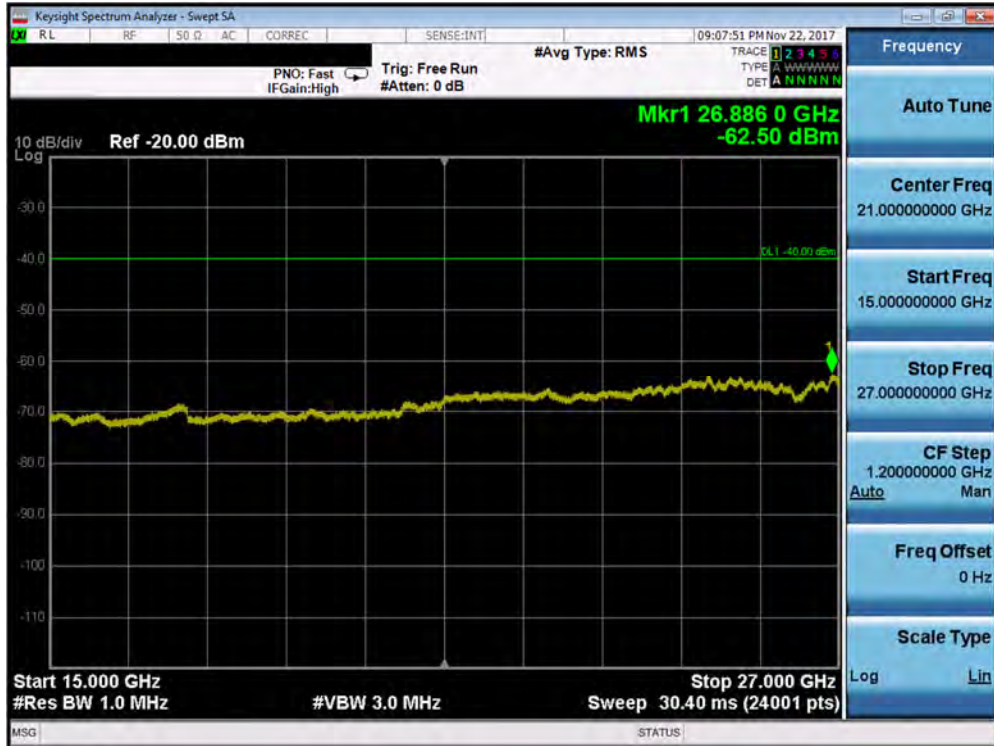
Plot 7-180. Conducted Spurious Plot (Band 30 - 5.0MHz QPSK - RB Size 1, RB Offset 0 - Low Channel – Antenna A)
