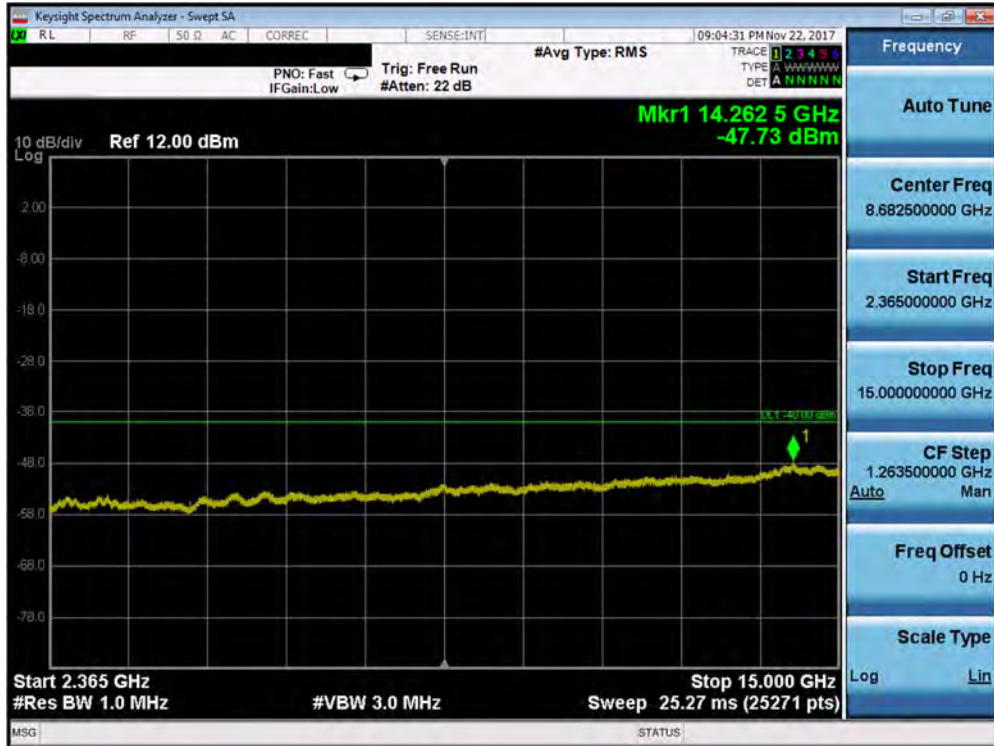
Plot 7-182. Conducted Spurious Plot (Band 30 - 5.0MHz QPSK - RB Size 1, RB Offset 0 - High Channel – Antenna A)
