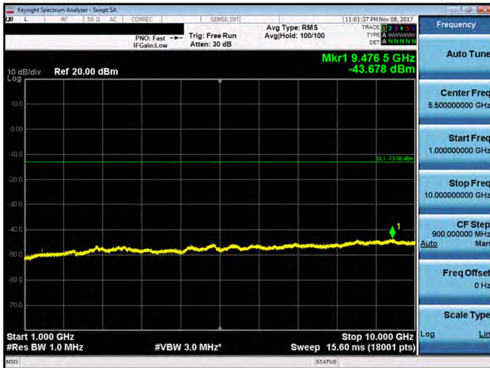
Plot 7-144. Conducted Spurious Plot (Band 12/17 - 5.0MHz QPSK - RB Size 1, RB Offset 0 - Mid Channel)
