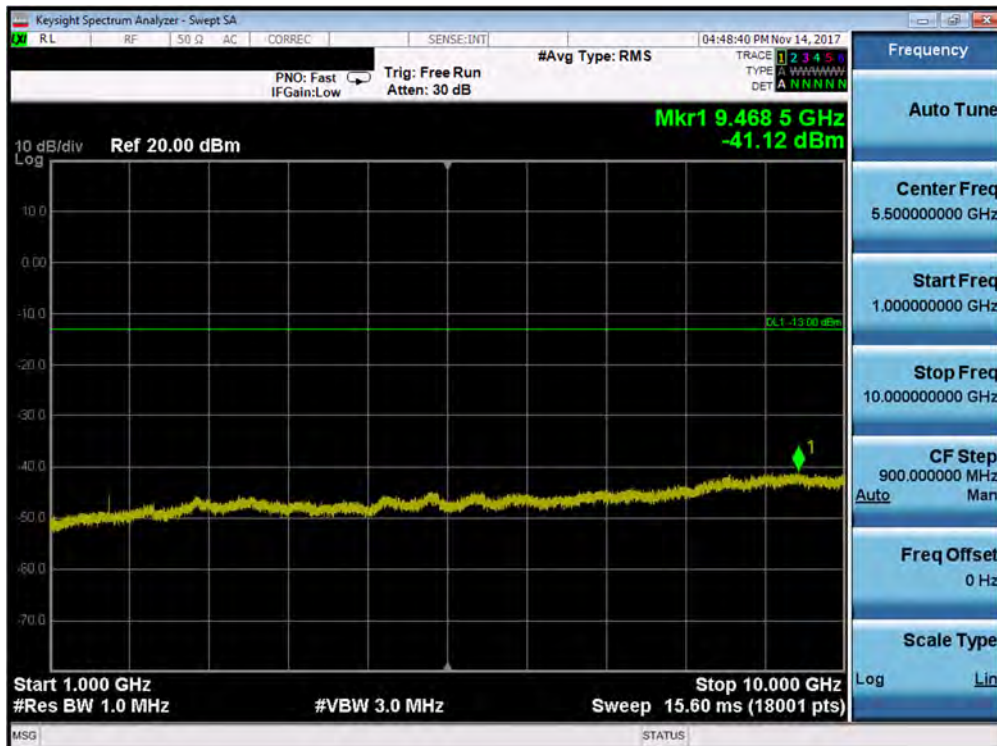
Plot 7-156. Conducted Spurious Plot (Band 26/5 - 5.0MHz QPSK - RB Size 1, RB Offset 0 - Mid Channel)
