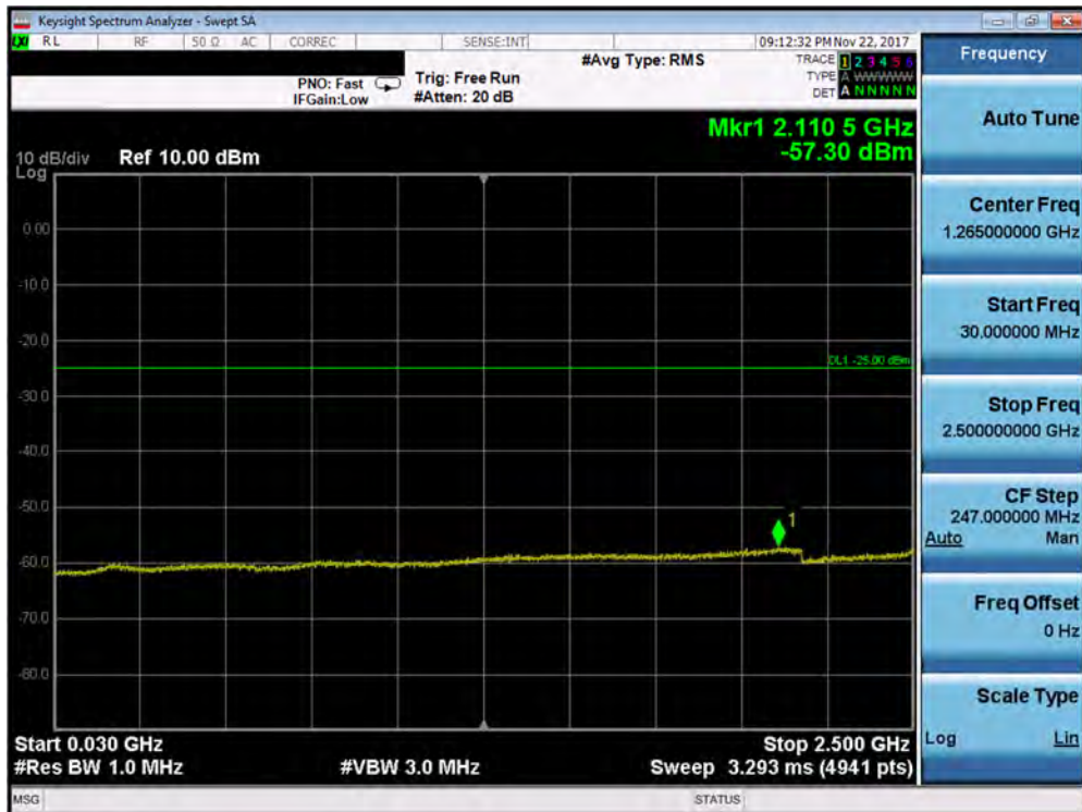
Plot 7-193. Conducted Spurious Plot (Band 7 - 5.0MHz QPSK - RB Size 1, RB Offset 0 - Mid Channel – Antenna A)
