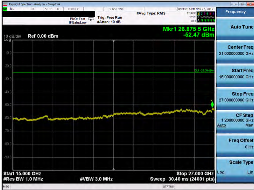
Plot 7-192. Conducted Spurious Plot (Band 7 - 5.0MHz QPSK - RB Size 1, RB Offset 0 - Low Channel – Antenna A)
