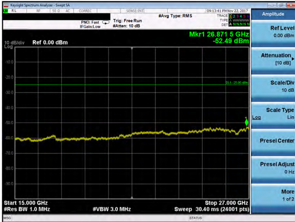
Plot 7-195. Conducted Spurious Plot (Band 7 - 5.0MHz QPSK - RB Size 1, RB Offset 0 - Mid Channel – Antenna A)
