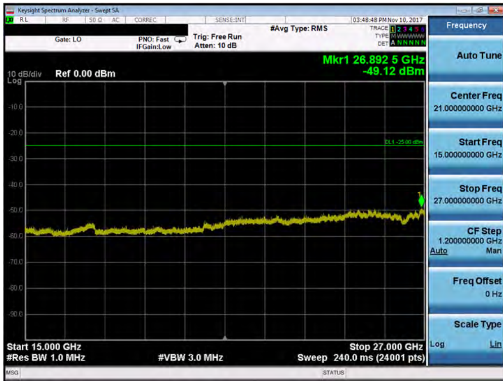
Plot 7-210. Conducted Spurious Plot (Band 41 - 20.0MHz QPSK - RB Size 1, RB Offset 0 - Low Channel)
