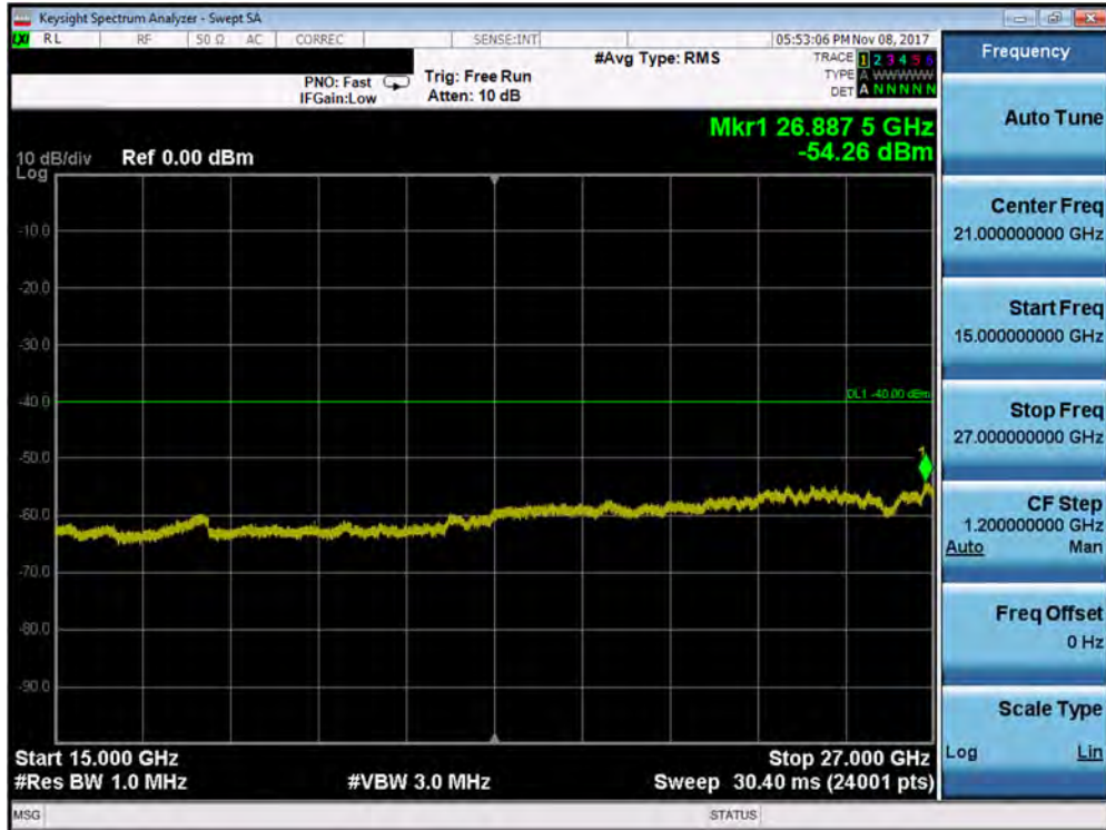
Plot 7-186. Conducted Spurious Plot (Band 30 - 5.0MHz QPSK - RB Size 1, RB Offset 0 - Low Channel – Antenna B)
