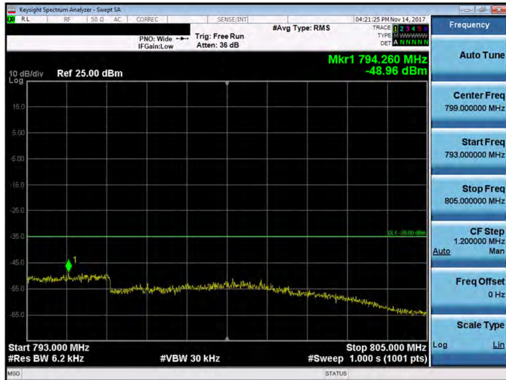
Plot 7-242. Lower Emission Mask Edge Plot (Band 13 – 10.0MHz QPSK – Full RB Configuration)
