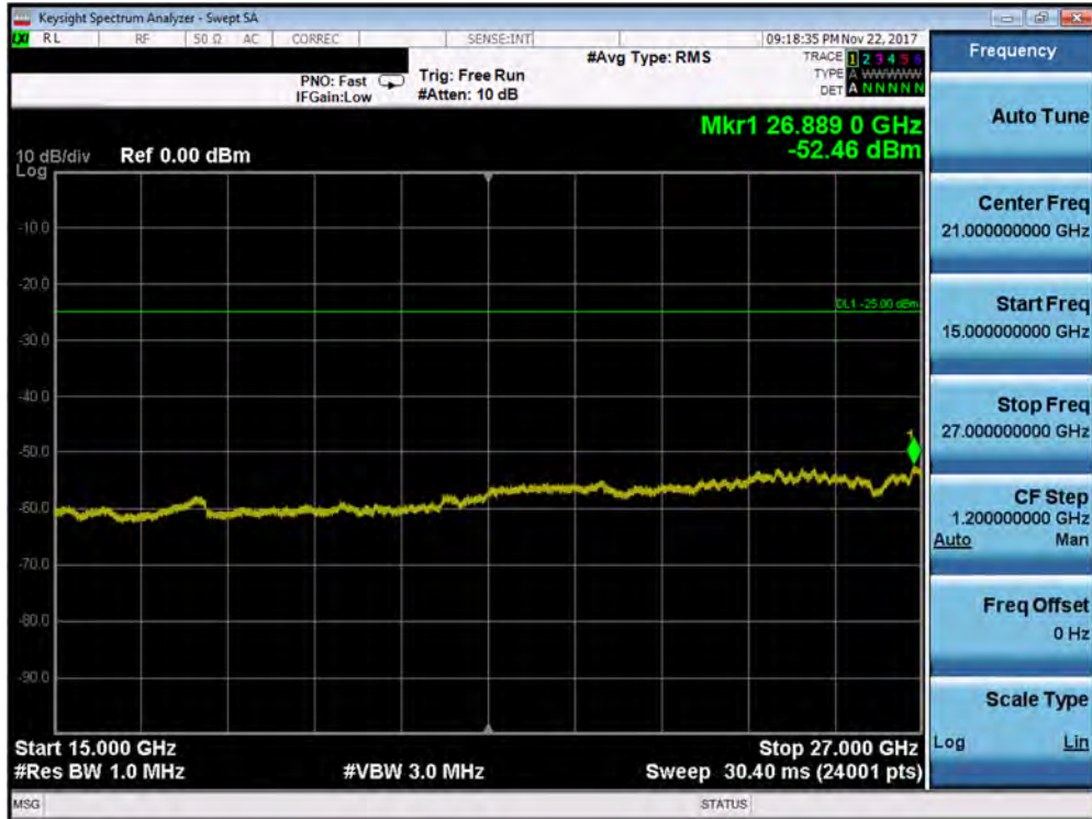
Plot 7-198. Conducted Spurious Plot (Band 7 - 5.0MHz QPSK - RB Size 1, RB Offset 0 - High Channel – Antenna A)
