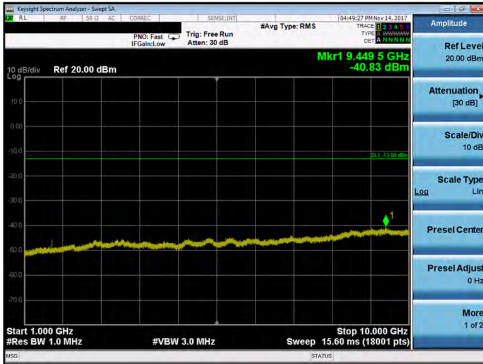
Plot 7-153. Conducted Spurious Plot (Band 26/5 - 5.0MHz QPSK - RB Size 1, RB Offset 0 - Low Channel)
