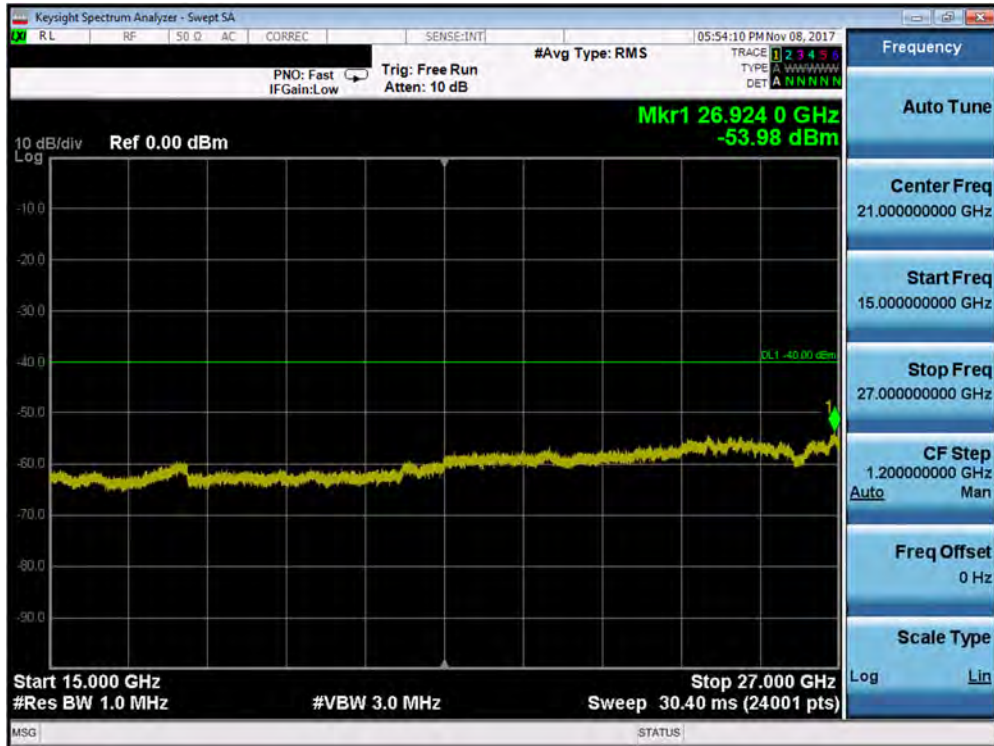
Plot 7-189. Conducted Spurious Plot (Band 30 - 5.0MHz QPSK - RB Size 1, RB Offset 0 - High Channel – Antenna B)
