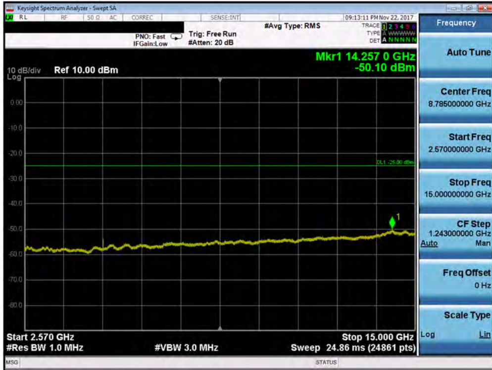
Plot 7-194. Conducted Spurious Plot (Band 7 - 5.0MHz QPSK - RB Size 1, RB Offset 0 - Mid Channel – Antenna A)
