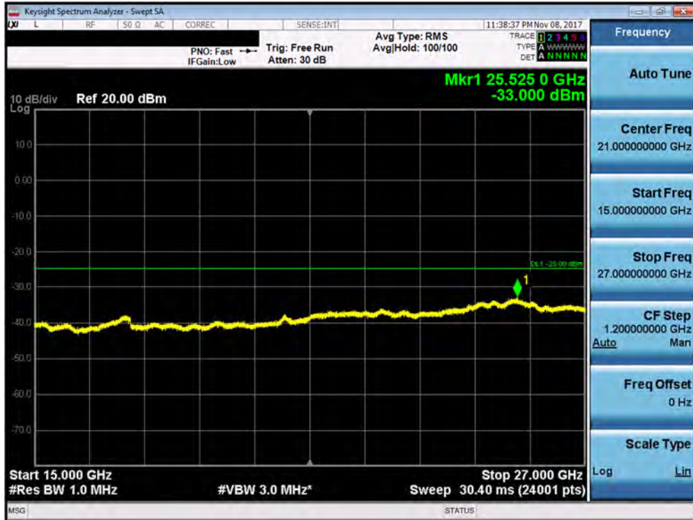
Plot 7-201. Conducted Spurious Plot (Band 7 - 5.0MHz QPSK - RB Size 1, RB Offset 0 - Low Channel – Antenna B)
