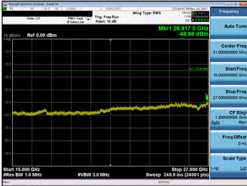
Plot 7-216. Conducted Spurious Plot (Band 41 - 20.0MHz QPSK - RB Size 1, RB Offset 0 - High Channel)
