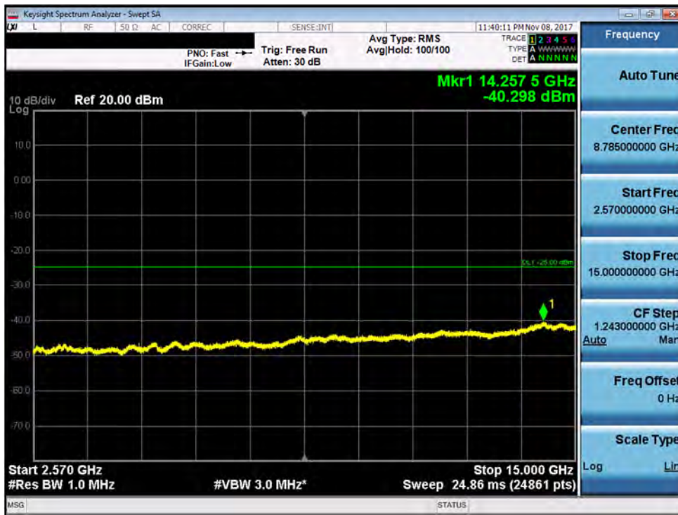
Plot 7-200. Conducted Spurious Plot (Band 7 - 5.0MHz QPSK - RB Size 1, RB Offset 0 - Low Channel – Antenna B)
