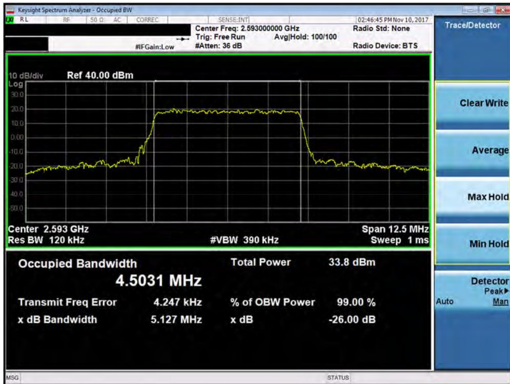
Plot 7-119. Occupied Bandwidth Plot (Band 41 - 5.0MHz 16-QAM - Full RB Configuration)
