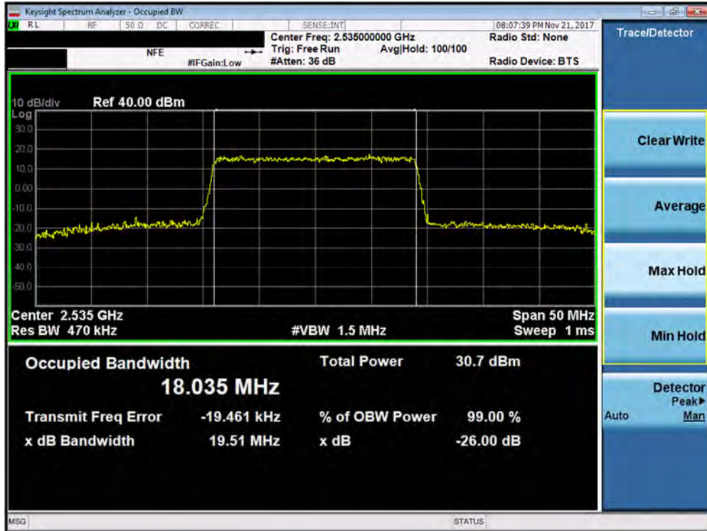
Plot 7-116. Occupied Bandwidth Plot (Band 7 - 20.0MHz 16-QAM - Full RB Configuration – Antenna B)
