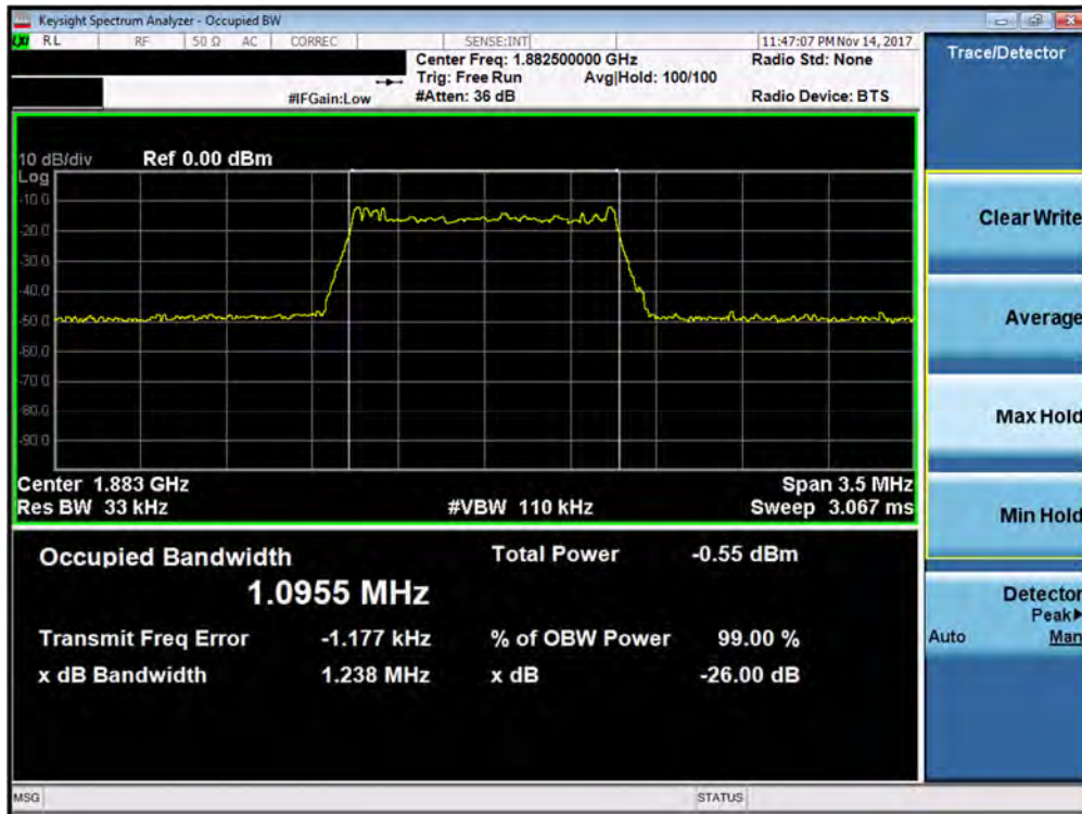
Plot 7-64. Occupied Bandwidth Plot (Band 25/2 - 1.4MHz QPSK - Full RB Configuration)
