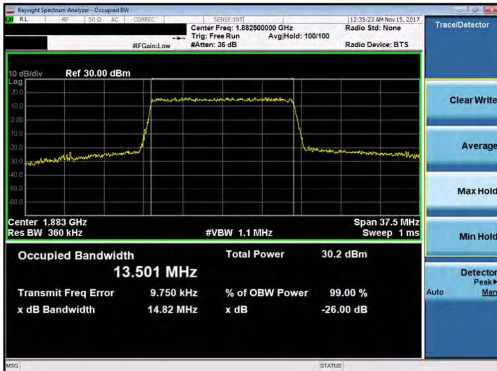
Plot 7-77. Occupied Bandwidth Plot (Band 25/2 - 15.0MHz 16-QAM - Full RB Configuration)
