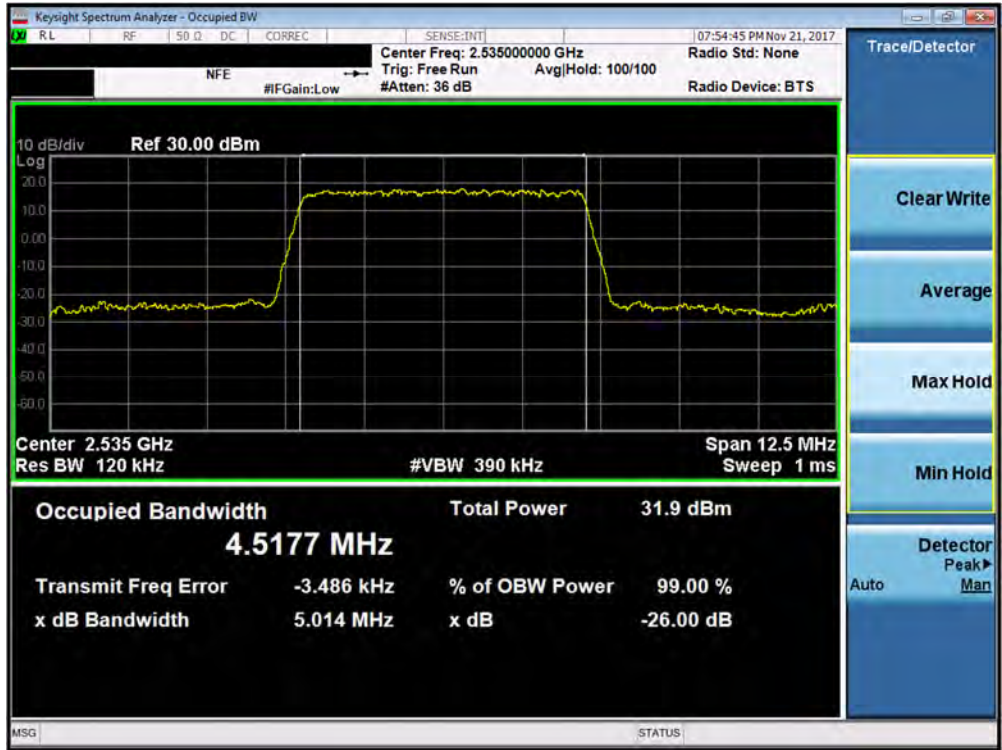
Plot 7-106. Occupied Bandwidth Plot (Band 7 - 5.0MHz QPSK - Full RB Configuration – Antenna B)
