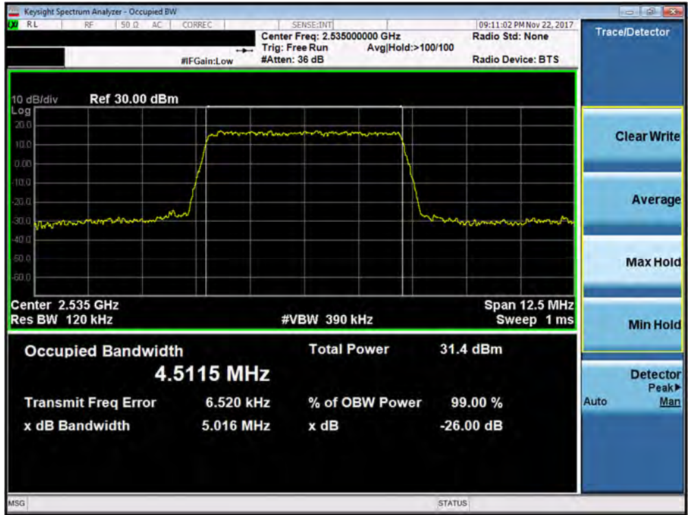
Plot 7-94. Occupied Bandwidth Plot (Band 7 - 5.0MHz QPSK - Full RB Configuration – Antenna A)
