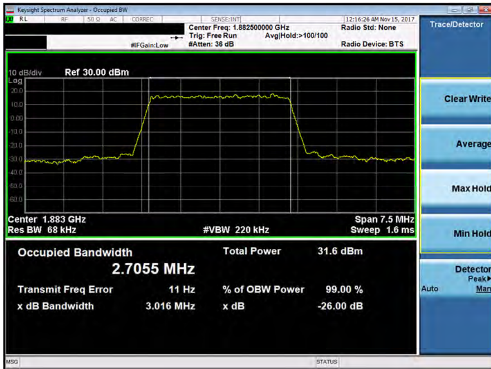
Plot 7-67. Occupied Bandwidth Plot (Band 25/2 - 3.0MHz QPSK - Full RB Configuration)
