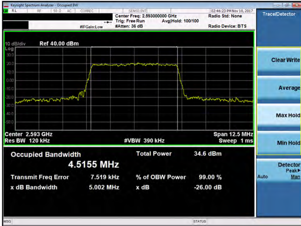
Plot 7-118. Occupied Bandwidth Plot (Band 41 - 5.0MHz QPSK - Full RB Configuration)
