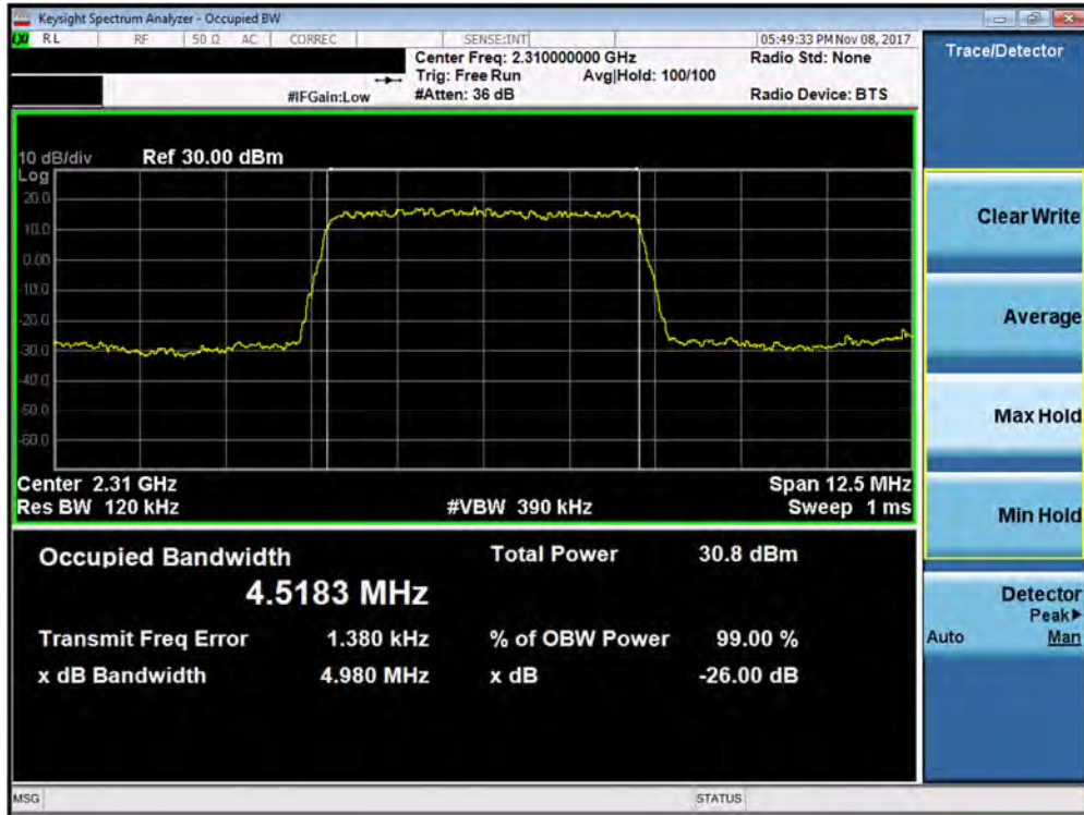
Plot 7-88. Occupied Bandwidth Plot (Band 30 - 5.0MHz QPSK - Full RB Configuration – Antenna B)
