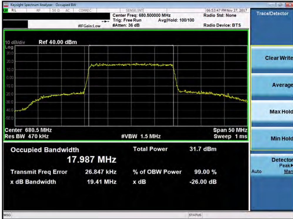
Plot 7-11. Occupied Bandwidth Plot (Band 71 - 20.0MHz 16-QAM - Full RB Configuration)
