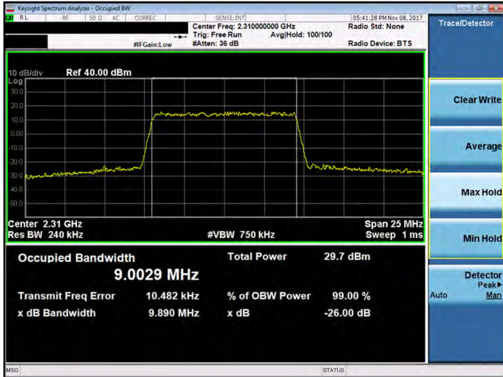
Plot 7-92. Occupied Bandwidth Plot (Band 30 - 10.0MHz 16-QAM - Full RB Configuration – Antenna B)
