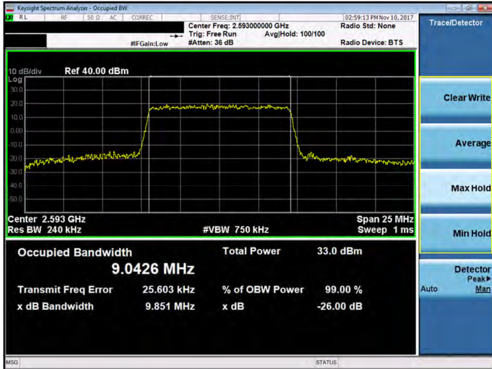
Plot 7-122. Occupied Bandwidth Plot (Band 41 - 10.0MHz 16-QAM - Full RB Configuration)
