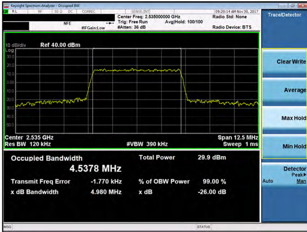
Plot 7-96. Occupied Bandwidth Plot (Band 7 - 5.0MHz 64-QAM - Full RB Configuration – Antenna A)
