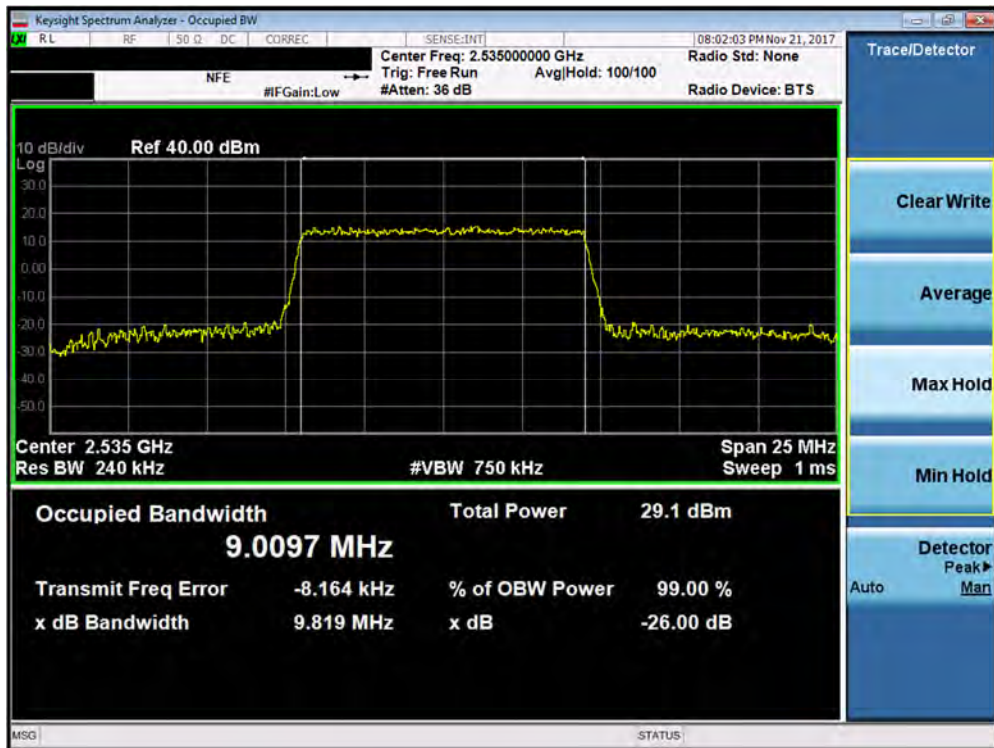
Plot 7-111. Occupied Bandwidth Plot (Band 7 - 10.0MHz 64-QAM - Full RB Configuration – Antenna B)
