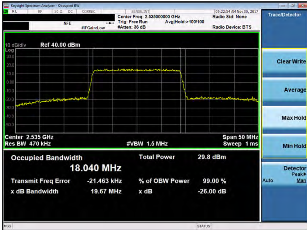
Plot 7-105. Occupied Bandwidth Plot (Band 7 - 20.0MHz 64-QAM - Full RB Configuration – Antenna A)
