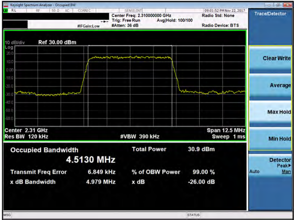
Plot 7-82. Occupied Bandwidth Plot (Band 30 - 5.0MHz QPSK - Full RB Configuration – Antenna A)
