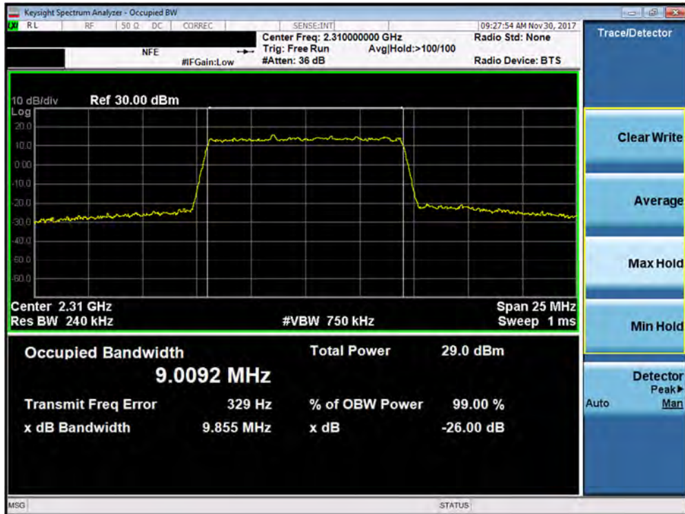
Plot 7-87. Occupied Bandwidth Plot (Band 30 - 10.0MHz 64-QAM - Full RB Configuration – Antenna A)
