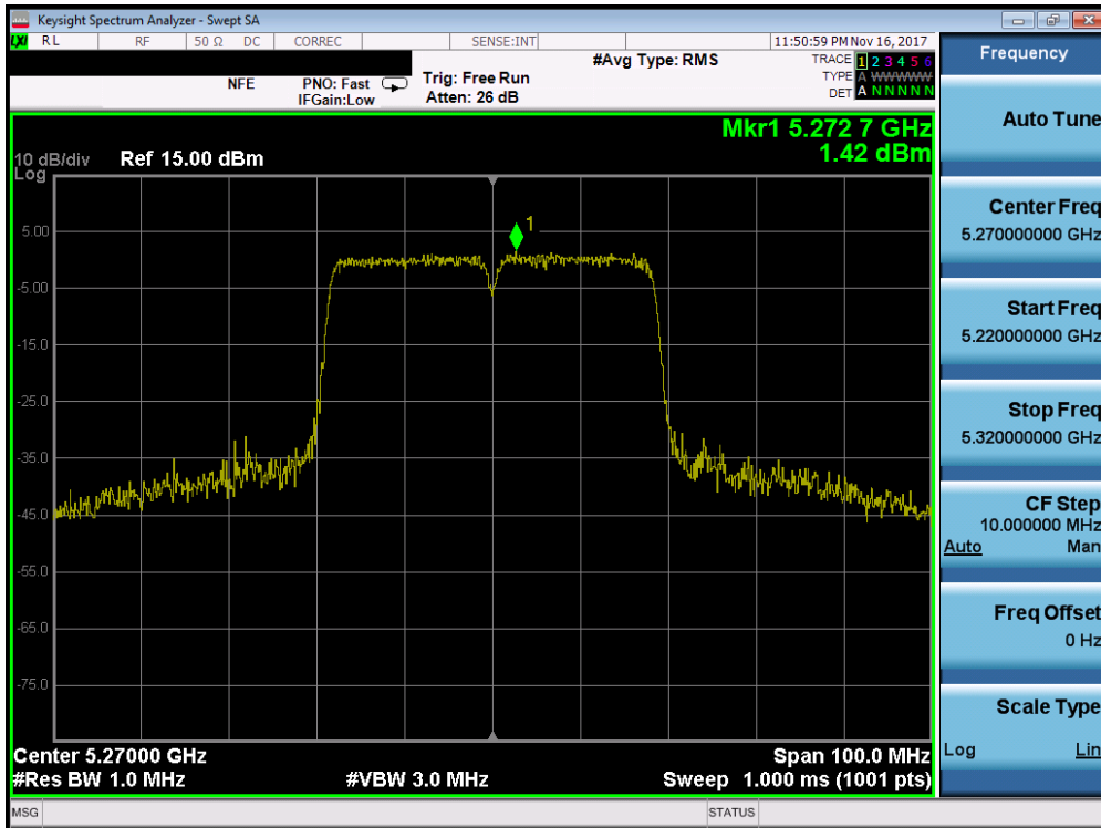
Plot 7-92. Power Spectral Density Plot (40MHz BW 802.11n (UNII Band 2A) – Ch. 54)
