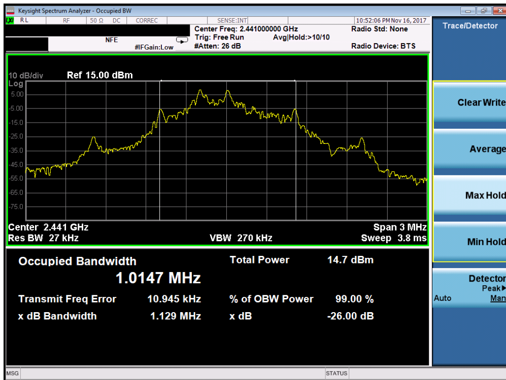
Plot 7-1. Occupied Bandwidth Plot (ANT+ – Ch. 39)
