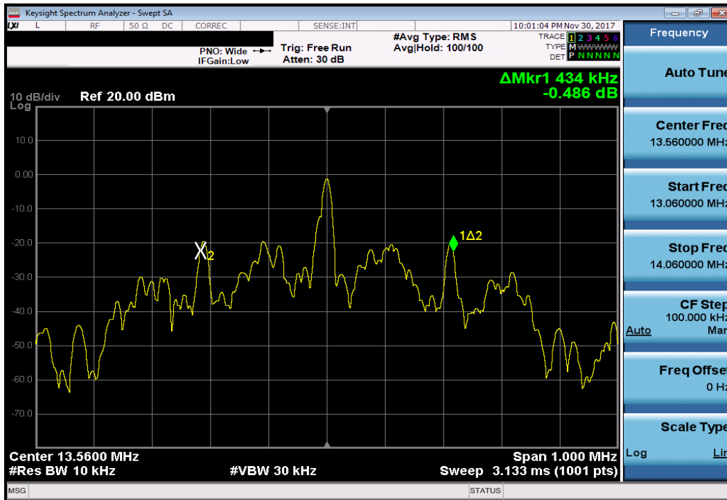
Figure 7-2. 20dB Bandwidth Plot
