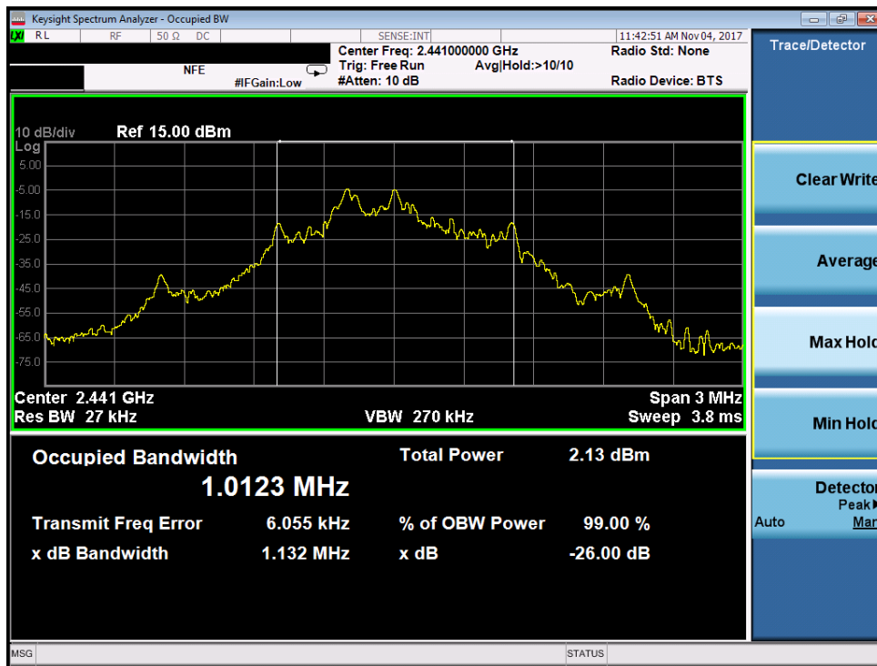
Plot 7-1. Occupied Bandwidth Plot (ANT+ – Ch. 39)
